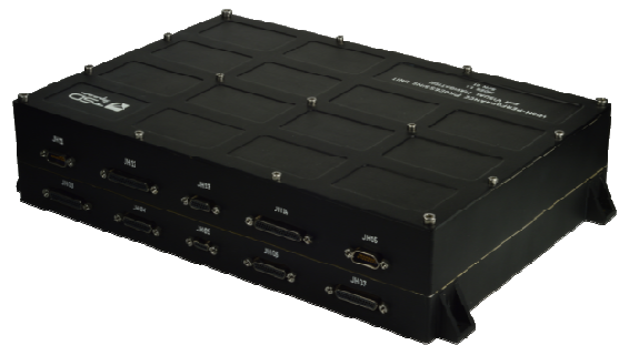
Figure 7: HPHC engineering model assembled in its cabinet
