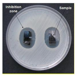
Figure 5.21: Example of inhibition halo after antibacterial test
