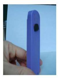
Figure 5.16: Magnetic interaction between a magnet and SC45-3Ag after annealing treatment
