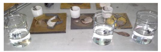
Figure 7.18: SC45 doped with ion silver after ion exchange with molten salt. The samples SC45 Ag20, SC45 ,Ag200, SC45 Ag2000) were quenched on a plate and then put in water for salt dissolution.
