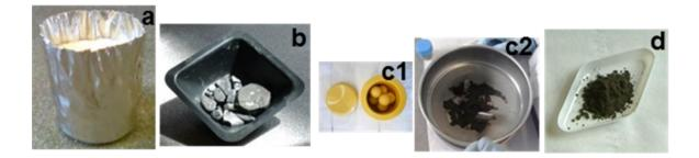
Figure 5.1: Synthesis steps for the glass ceramic production with melting and quenching technique : Reagents in a platinum crucible(a), pouring on plate (b), milling (c1) and sieving up with 20 micron mesh sieve (c2), ferrimagnetic glass ceramic powder < 20 μm (d).
