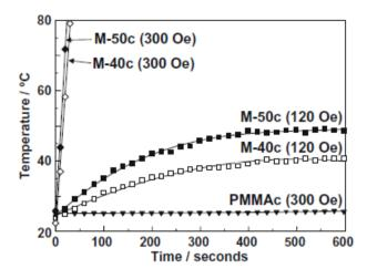
Figure 4.4: Calorimetric curve of different samples at different alternating magnetic field of 120 and 300 Oe at 100 kHz[1]
