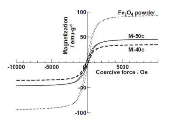
Figure 4.3: Magnetization curves of Fe<sub>3</sub>O<sub>4</sub> powder and sample M-50c and M-40c under magnetic fields of 10 kOe
