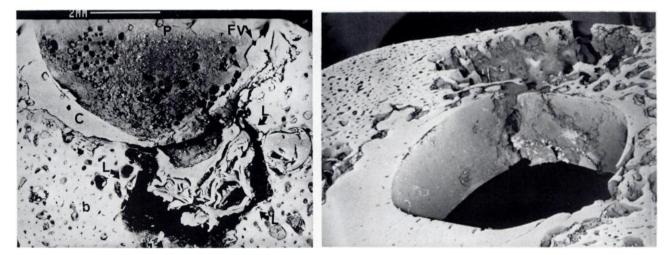
Figure 2.11: Scanning electron micrograph of a post-mortem specimen. The image on the left shows multiple cement fractures and adjacent fragmentation to the osteolysis area. P is a cement plug at the tip of the prosthesis; FV is a fracture through voids in the cement; C is bone cement; b is bone; L is focal lysis in the cortical bone. On the right a detail where it is possible to distinguish the fracture of the PMMA cement and behind it the fracture and resorption of cortical bone.[24]
