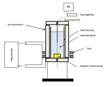
Figure 5.4: Calorimetric set up with a foam polyethylene as a thermal insulator
