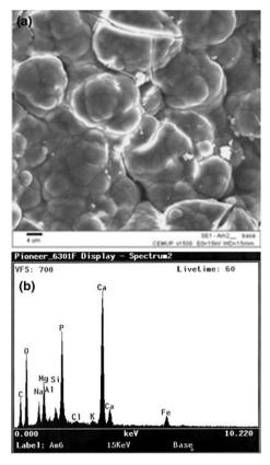
Figure 4.13:Ferrimagnetic cement immersed in normal SBF. A Precipitates covering the initial surface . b The precipitation of Ca and Mg phospjate compound is detected. All the initial cement peaks of Si and Fe decreased and a high peak of P can be observed[7]
