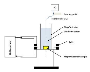
Figure 5.3: Calorimetric set-up for heating measures
