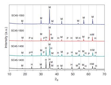
Figure 3.19: XRD patterns of ferrimagnetic glass-ceramic samples (M = magnetite, H = hematite, P = sodium calcium silicate).[14]
