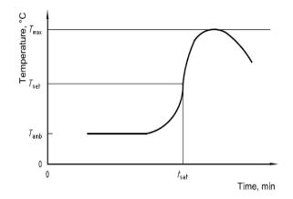
Figure 5.10: Typical setting time curve of polymeric bone cement[11]
