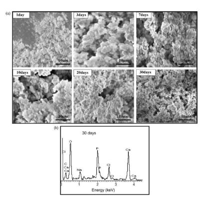
Figure 3.23: (a) SEM micrographs of the surfaces of glass-ceramic sample with x = 15 wt.% soaked in SBF for various days (magnification: 1000) and (b) EDS spectra of x = 15 wt.% soaked in SBF for 30 days.[17]
