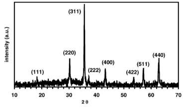
Figure 3.13: X-ray diffraction pattern (XRD) of glass ceramic[12]
