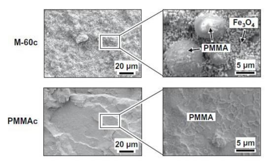
Figure 4.2:SEM analysis of cross- sectional areas of the cement samples.[1]
