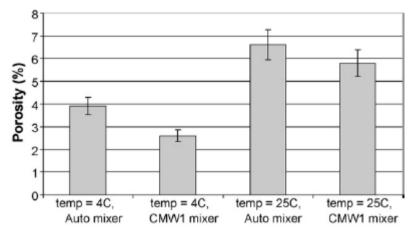
Figure 2.6: Mixing and temperature effect on the porosity of acrylic bone cement
