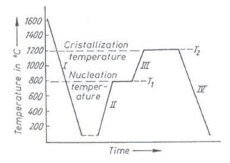
Figure 3.5: Nucleation and crystallization thermal treatments[1]
