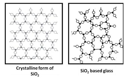
Figure 3.3:Difference between crystalline and amorphous SiO2 [1]
