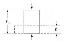
Figure 5.7: ideal compression test, following the application of a force the hight of the sample change from lo from l with a deformation of the specimen.
