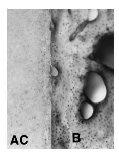
Figure 2.8: HAp precipitation at the bone implant interface. The effect is due to the presence of a bioactive phase into the polymer. AC is a bioactive bone cement while B is a bone [21]
