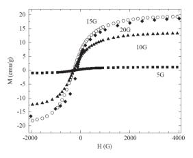
Figure 3.25: M–H plots of the samples with 5%, 10%, 15% and 20% molar fraction of Fe2O3 in the reacting oxides. The response in applied magnetic field H up to 4 kG is shown.[18]
