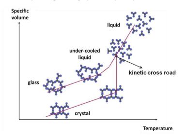
Figure 3.2: Mechanism of glass formation Specific volume vs temperature diagram . [2]
