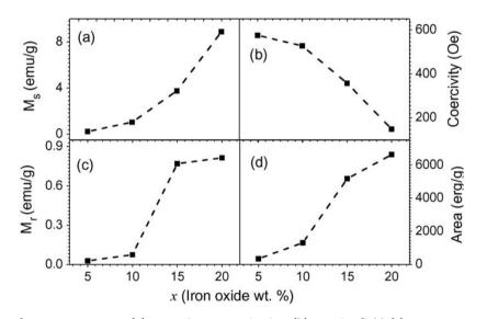
Figure 3.22: Variation of room temperature (a) saturation magnetization, (b) coercive field, (c) remanent magnetization, and (d) area under the M–H loop of glassceramics as a function of iron oxide content.[17]
