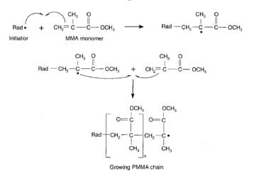
Figure 2.1: Polymerization of PMMA by an addition reaction. MMA monomer reacts with a radical to generate e second radical that can attack the double bond of another MMA monomer. [2]
