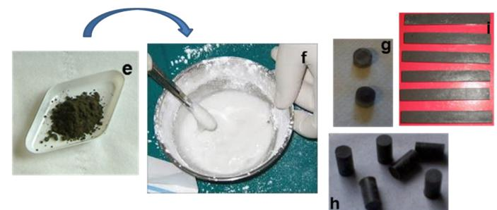
Figure 5.2: Synthesis steps of magnetic bone cement production: manual mixing with PMMA/MMA + SC45 < 20 μm in different % wt proportion (10-15-20) (e-f). After setting and extrusion from mould , different samples are prepared for different test: compression test (h), bioactivity and calorimetric tests (g), four point bending test (i).
