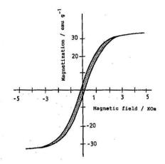
Figure 3.17: hysteresis loop of CSFe+B<sub>2</sub>O<sub>3</sub>+P<sub>2</sub>O<sub>5</sub> (CSFe+BP) glass heat treat at 1050 °C [13]
