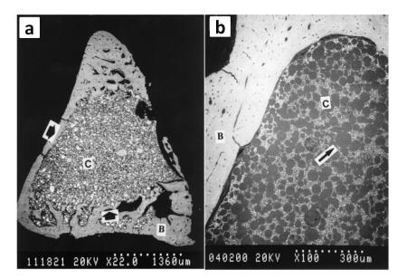
Figure 2.7: SEM microphotographs showing axial sections of rat tibiae 8 weeks after the implantation.(a) bioactive bone cement and(b) control cement with no bioactive phase;
