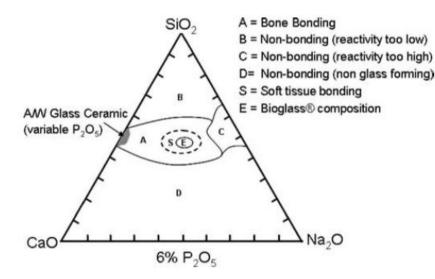
Figure 3.6: The graph shows compositional dependence (in weight percent, %wt) of the ternary compounds for the identification of the best bioglass formulation  $P_2O_5$  is constant at 6 %wt.[4]
