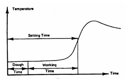
Figure 2.4: Setting time test: evaluation of the hardening time
