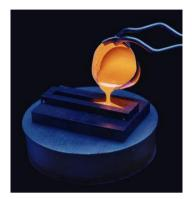
Figure 3.1: Cast of a glass into a mould[1]
