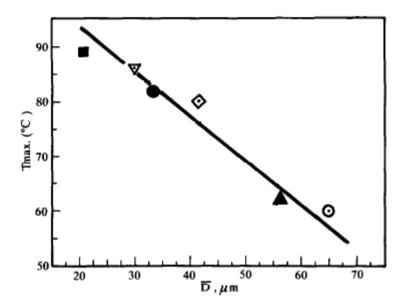
Figure 2.5: Relationship between average size of PMMA and the maximum temperature reached during the polymerization process of acrylic bone cement formulations[2]
