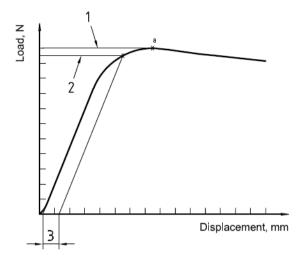
Figure 5.8 Theoretical load-displacement diagram for a cement
