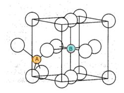
Figure 3.27: Tetrahedral and octahedral cation sites in the crystal structure of magnetite (Fe<sub>3</sub>O<sub>4</sub>). In a tetrahedral site A the iron ion is surrounded by 4 atoms of oxygens while in octahedral site the iron ion is surrounded by six oxygen atoms. [10]
