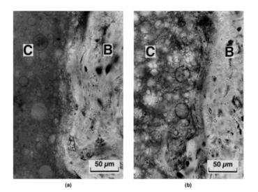
Figure 2.10: (a) bioactive cement with 4 μm disperse glass particles and (b) bioactive cement with 13 μm disperse glass particles in rat tibiae at 4 weeks after implantation. Direct bone formation was observed on two different bioactive glass cement formulations without intervening soft tissue layer. C, cement; B, bone. Original magnification at 400x.[23]
