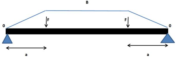
Figure 5.9: Distribution of bending moment in a 4 point flexural test
