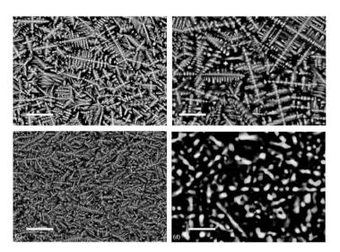
Figure 3.24: SEM images from samples of the series 20G presenting the effect of heat-treatment temperature on the microstructure of FBC: (a) as prepared,(b) heat-treated at 600 1C, (c) at 800 1C and (d) at 1100 1C. Bar is 2 mm.[18]
