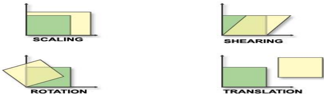
Figure 2.3. General concepts of Affine registration in which the transformation functions consist of only linear transformation.
