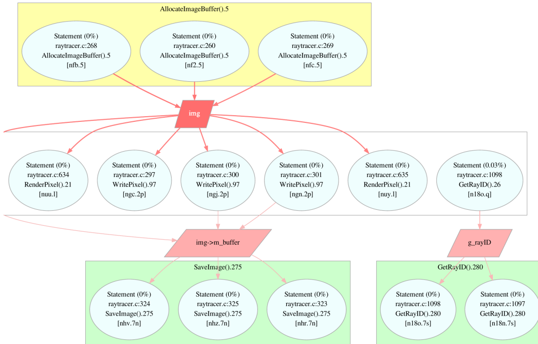
Fig. 12. Excerpt of the data dependency view of the full RenderPixel call stack of the ray tracer application. From top to bottom the layers in the view are: statements producing data dependencies outside the call stack; the data produced by these; the statements that consume/produce data dependencies within the call stack; the data produced by these; the statements consuming the data dependencies outside the call stack.
