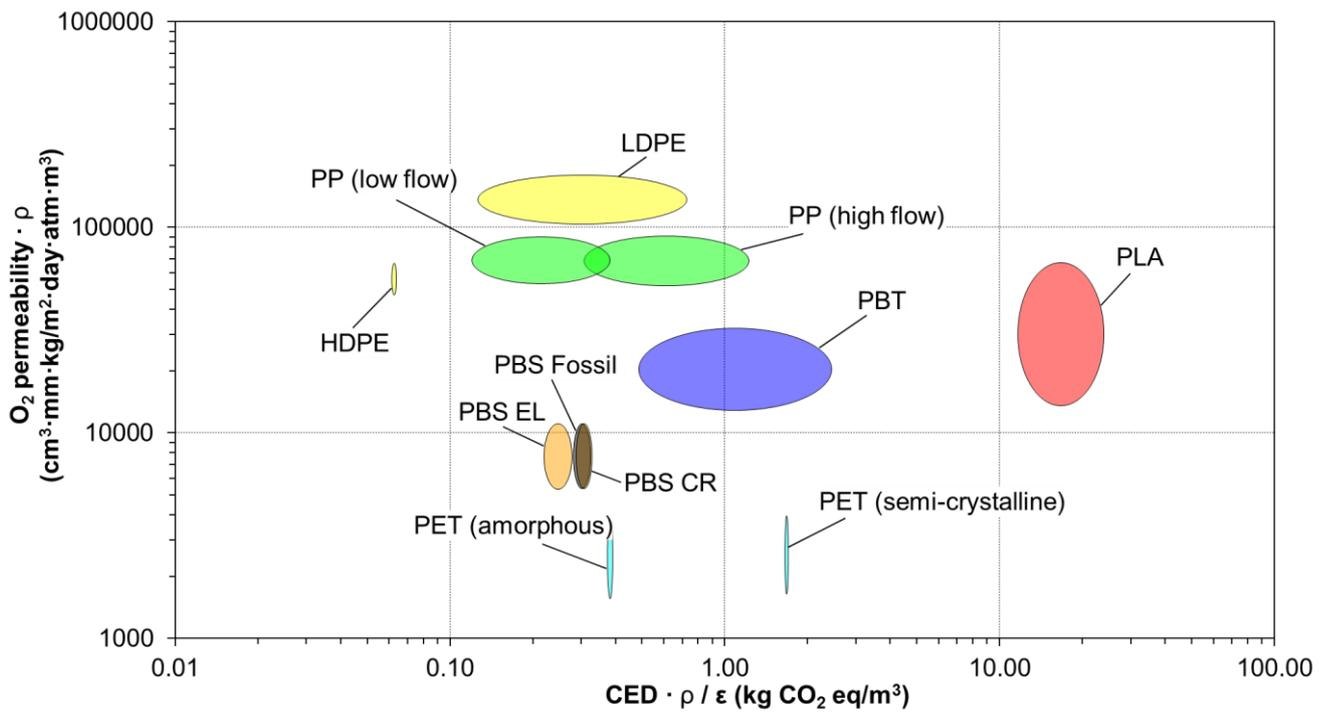
Figure 5.11 - Ashby plot for the multi-criteria materials selection based on  $O_2$  permeability  $\cdot \rho$  and  $\frac{\epsilon}{CED \cdot \rho}$ .
