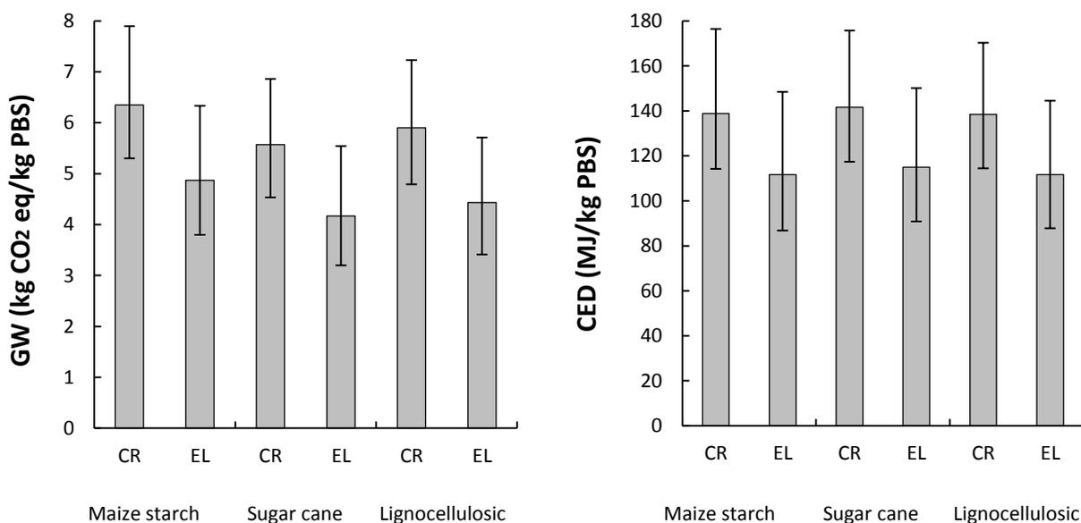
Figure 4.12 - Sensitivity analysis of GW and CED indicators for PBS with succinic acid from different renewable biomasses (maize starch, sugar cane, lignocellulosic biomass) and from different processes (CR = crystallization, EL = electro dialysis).
