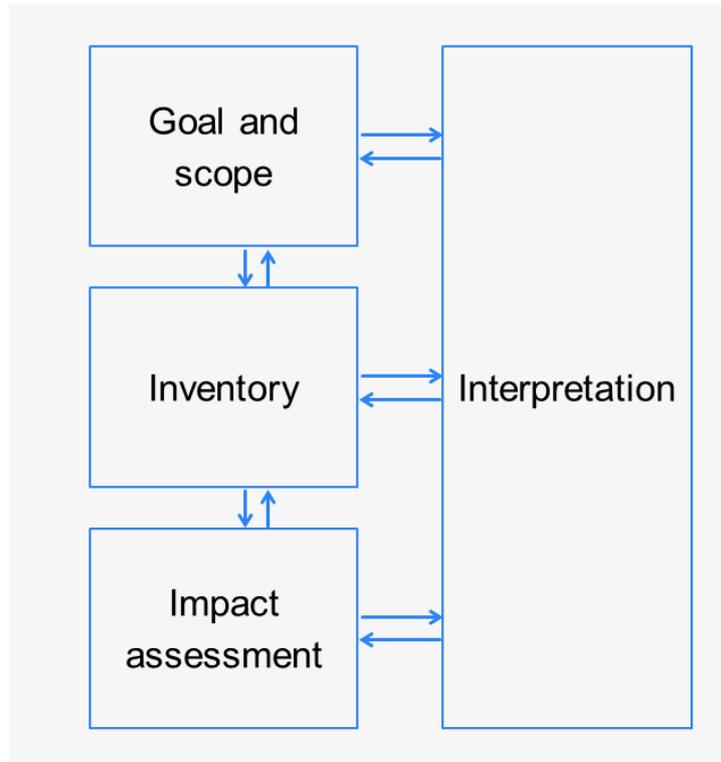
Figure 1.1 - LCA structure according to ISO 14040 and ISO 14044
