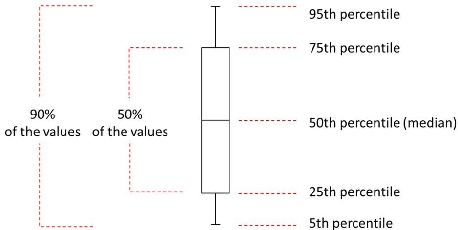
Figure 1.8 - Boxplot chart example. Definition of a probability distribution by means of 5<sup>th</sup>, 25<sup>th</sup>, 50<sup>th</sup>, 75<sup>th</sup> and 95<sup>th</sup> percentiles.
