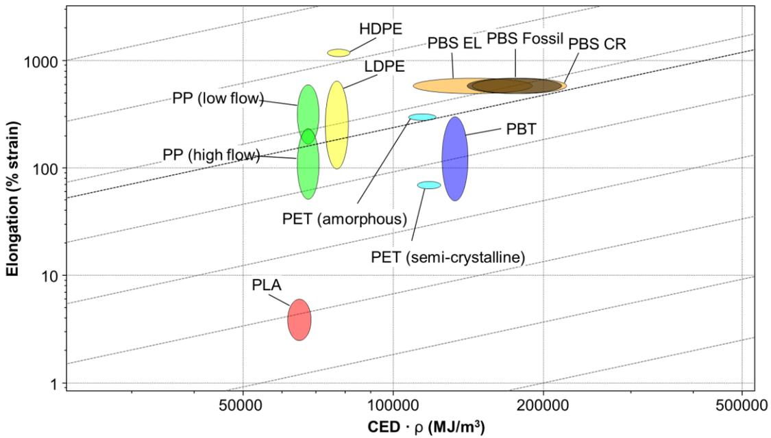
Figure 5.6 - Ashby plot for materials selection based on the material index  $\varepsilon$  vs  $CED \cdot \rho$
