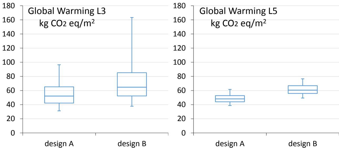
Figure 2.10 - Global warming distributions for design A and design B. On the left hand side distributions represent L3, in which material details are not specified ( $\beta = 69\%$ ). On the right hand side distributions represent L5, where BOMs are fully specified ( $\beta = 92\%$ ).
