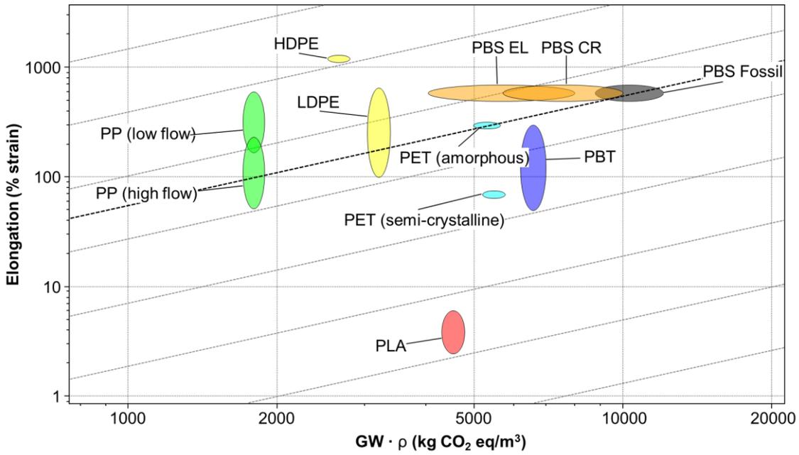
Figure 5.5 - Ashby plot for materials selection based on the material index  $\varepsilon$  vs  $GW \cdot \rho$
