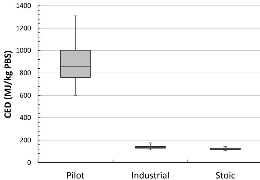
Figure 4.10 - CED for 1 kg of PBS (probability distributions, 5<sup>th</sup>, 25<sup>th</sup>, 50<sup>th</sup>, 75<sup>th</sup>, 95<sup>th</sup> percentiles) at different scales (pilot, industrial, stoichiometric).
