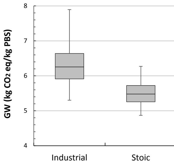
Figure 4.11 - Focus: GW impact of 1 kg of PBS (probability distributions, 5<sup>th</sup>, 25<sup>th</sup>, 50<sup>th</sup>, 75<sup>th</sup>, 95<sup>th</sup> percentiles) at different scales (industrial, stoichiometric)
