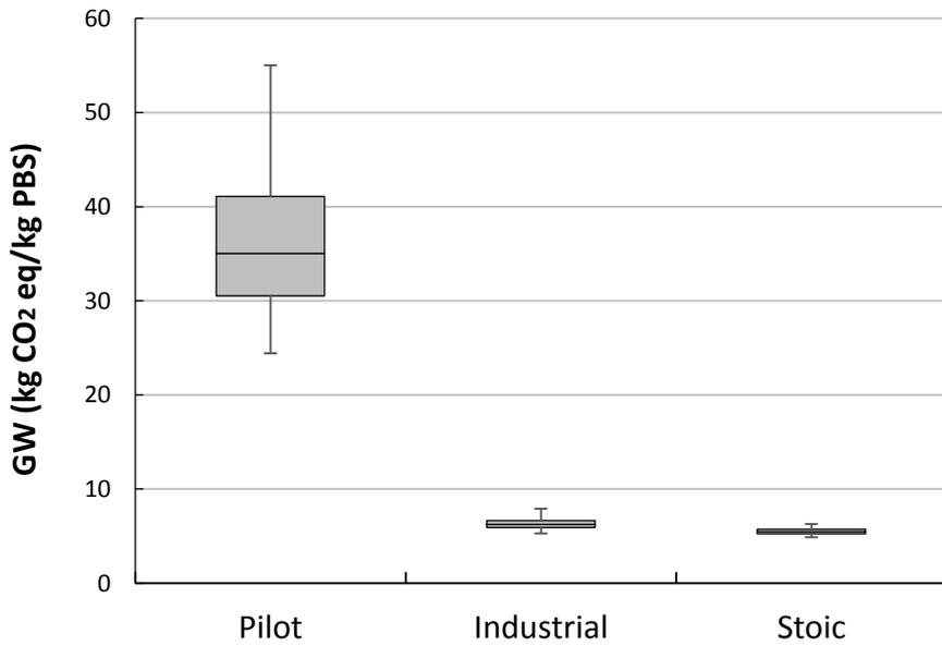
Figure 4.9 - GW impact of 1 kg of PBS (probability distributions, 5<sup>th</sup>, 25<sup>th</sup>, 50<sup>th</sup>, 75<sup>th</sup>, 95<sup>th</sup> percentiles) at different scales (pilot, industrial, stoichiometric).
