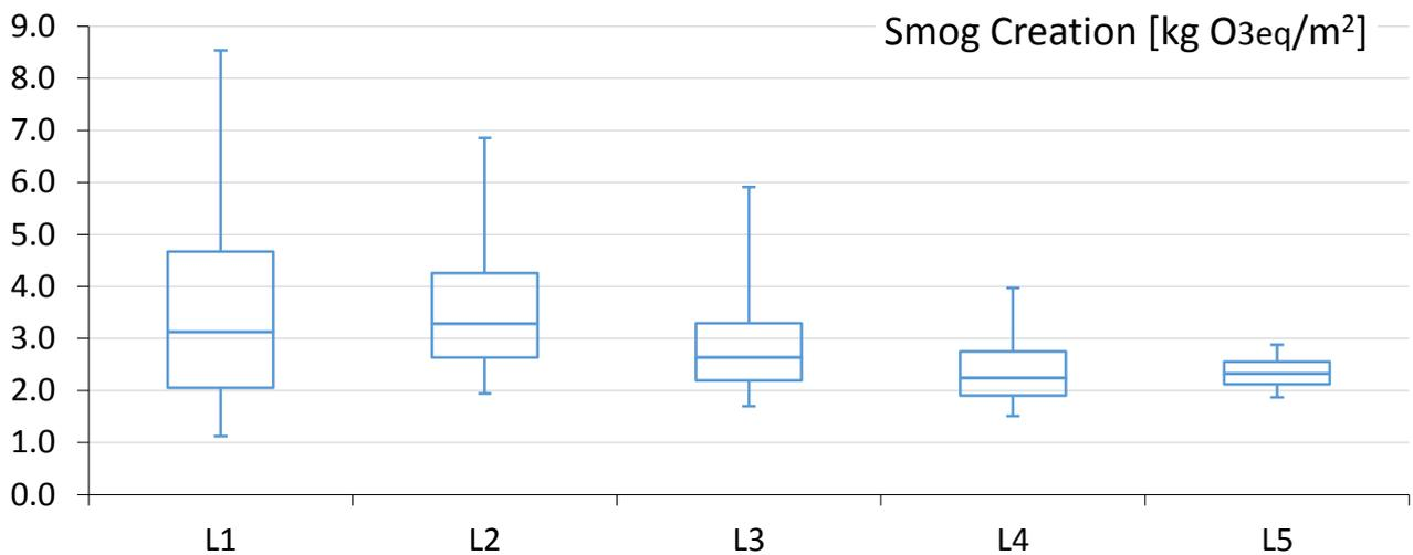
Figure 2.6 - Probabilistic distributions of smog creation results applied to an exterior wall (ICF). Typical results from an LCA study are represented by L5, while from L4 to L1 the probabilistic underspecification approach is used.
