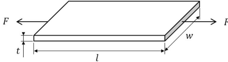
Figure 5.1 - Element of film undergoing a uniaxial load.
