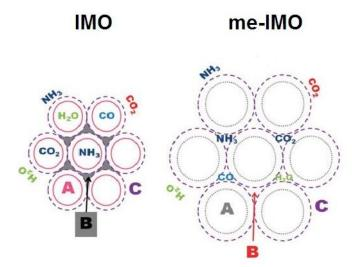
Fig. 2 Accessibility of the surfaces of IMO and Me-IMO NTs to probes having different composition and dimensions [8].
