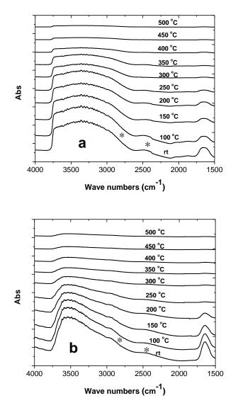
Fig. 3 IR spectra of self supporting samples a) Fe1.4-IMO and b) Fe1.4-loaded-IMO after outassing at different temperatures under vacuum with residual pressure  $< 10^{-3}$
