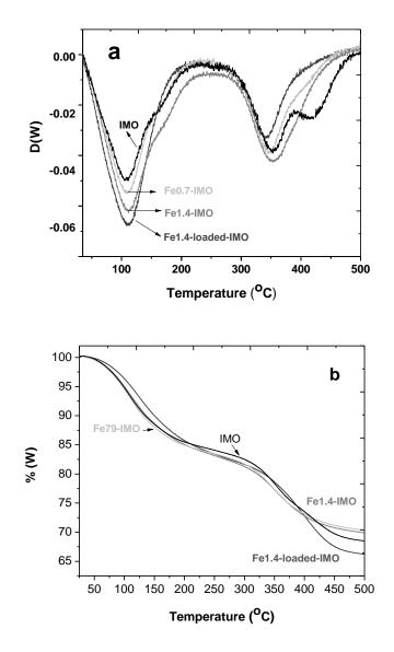
Fig.2 a) The differential thermal analysis (DTA) and b) thermo gravimetric analysis (TGA) of IMO, Fe0.7-IMO, Fe1.4-IMO and Fe1.4-loaded-IMO
