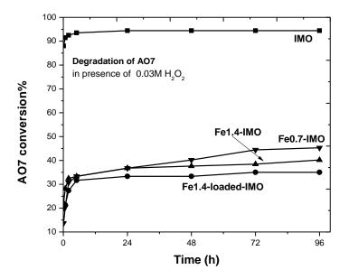
Fig. 16 catalytic activity in the degradation of AO7 in dark conditions in the presence of  $0.03 \text{ M H}_2\text{O}_2$  and 1 g/L catalyst reported as percentage of AO7 conversion versus time (h).
