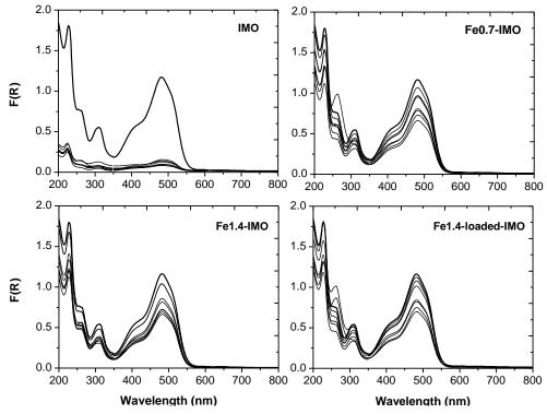
Fig. 20 UV-vis spectra of the supernatant solutions in the presence of 1.0 g/L catalysts and 0.1 M  $H_2O_2$ : 0.67 mM AO7 up to 96 h for IMO, Fe0.7-IMO, Fe1.4-IMO, Fe1.4-IOAded-IMO.
