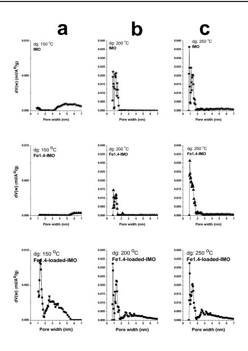
**Fig. 6** NL-DFT Pore Size Distributions of samples IMO (stars), Fe1.4-IMO (triangles) and Fe1.4-loadedIMO (squers) at different degassing temperatures a) 150 °C, b) 200 °C, C) 250 °C obtained by applying a N<sub>2</sub>-zeolite kernel to adsorption branches.
