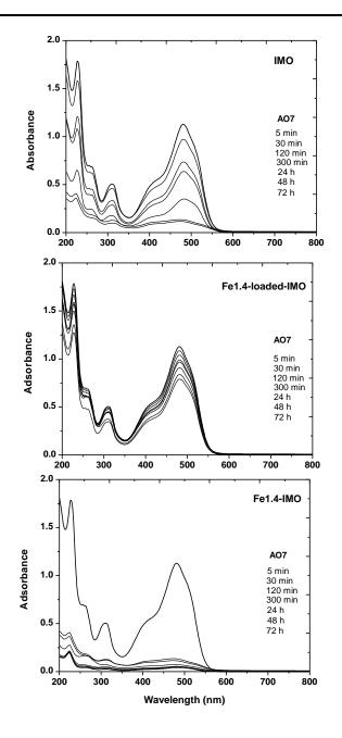
**Fig. 13** UV-Vis spectra of the supernatant solutions obtained after different contact times between 0.67 mM AO7 aqueous solution in presence of IMO (a) and Fe1.4-Ioaded-IMO (b) and Fe1.4-IMO (c) all three sections report the spectrum of the starting AO7 solution (bold curve) and those of the supernatant solutions obtained after 5 min, 30 min, 120 min, 24 h, 48 h and 72 h.
