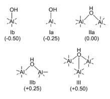
Fig. 18 Idealized hydroxyl configurations on the alumina surface proposed in the Knözinger and Ratnasamy model. The values in parentheses are the global charge on the hydroxyl groups [41].
