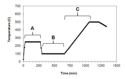
**Fig. 2** temperature program used for propylene oxidation test: A) dehydration of samples under helium flow (50 ml min<sup>-1</sup>) at 250  $^{\circ}$ C and for catalytic teat at B) 100  $^{\circ}$ C (steady state) and C) increasing temperature up to 500  $^{\circ}$ C.
