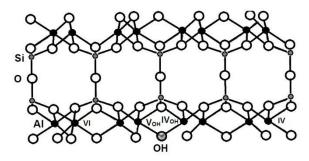
**Fig. 10** Scheme shows the structure proposed in the literature for the lamellar phase, as obtained from cleavage and subsequent condensation of nanotubes: Al may be six-coordinated (site VI in the scheme), four-coordinated (site IV) and four- or five-coordinated with residual hydroxyl (sites IVOH and VOH, respectively), whereas Si tends to form Si–O–Si bonds rather than silanols [3, 14].
