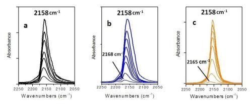
**Fig. 5** Difference IR spectra obtained after dosing CO at nominal -196 °C on IMO (a), Fe1.4-IMO (b) and Fe1.4-loaded-IMO (c) CO equilibrium pressure in the 0.50 - 20 mbar range, after degassing the samples at 250 °C under the residual pressure of  $10^{-3}$  mbar.
