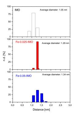
Fig. 7 Diameter distributions of IMO, Fe-0.025-IMO and Fe-0.05-IMO as obtained by HRTEM analysis.
