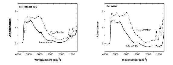
Fig. 9 Comparison of Fe1.4-loaded-IMO and Fe1.4-IMO spectra after outgassing at 250  $^{\circ}$ C (solid line) and after dosage of 30 mbar NH<sub>3</sub> at room temperature (dashed line).
