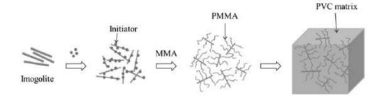
Fig. 5 Illustration of the fabrication procedure for PVC/PMMA-g-imogolite nanohybrid
