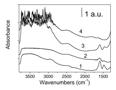
Fig. 3 IR spectra of IMO (1), Fe0.7-IMO (2), Fe1.4-loaded-IMO (3) and Fe1.4-IMO (4) samples that were dehydrated at 250 °C.
