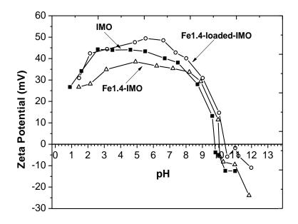
Fig. 10  $\zeta$  potential curves of IMO (squares), Fe1.4-IMO (triangles) and Fe1.4-loaded-IMO (circles).
