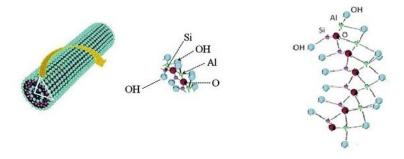
Fig. 1 schematic of present hydroxyls in imogolite structure
