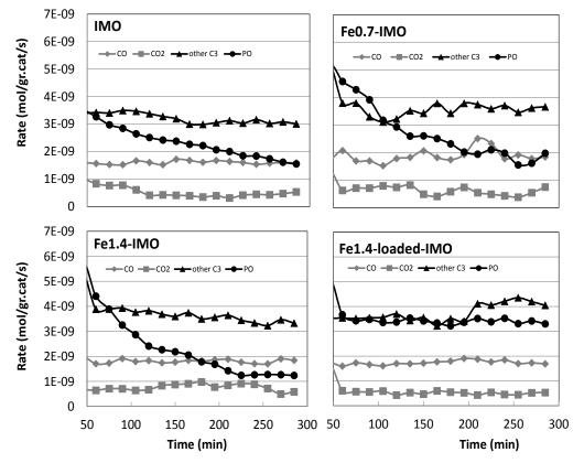
Fig. 6 Rate of different products (mol/gr.cat/s) at constant temperature (100 °C)
