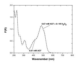
Fig. 19 UV-vis spectra concerning a solution obtained by mixing 0.67 mM AO7 and 0.1 M H<sub>2</sub>O<sub>2</sub> without any catalyst in the 200–800 nm range after 30 min
