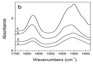
**Fig. 7** Section a: difference IR spectra obtained after dosing  $NH_3$  at r.t. on IMO dehydrated at 250 °C,  $NH_3$  equilibrium pressure in the 0.50-30 mbar range. Section b: difference IR spectra obtained with IMO (1), Fe0.7-IMO (2), Fe1.4-loaded-IMO (3) and Fe1.4-IMO (d). Differences were obtained by subtracting IR spectra of bare samples reported in Fig. 3.
