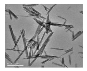
Fig. 4 TEM image of halloysite nanotubes [83].
