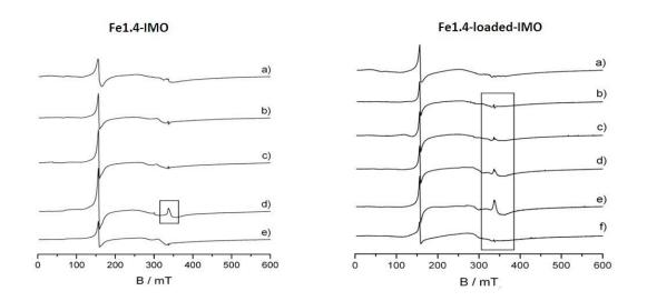
**Fig. 18** EPR spectra of Fe1.4-IMO (left side): a) dehydrated at room temperature, b) dehydrated at 200 °C, C) NO presuure:2 mbar, d) NO presuure:10 mbar, e) evacuated at room temperature. EPR spectra of Fe1.4-loaded-IMO (right side): a) dehydrated at room temperature, b) dehydrated at 200 °C, C) NO presuure:2 mbar, d) NO presuure:10 mbar, e) NO presuure:20 mbar, f) evacuated at room temperature.
