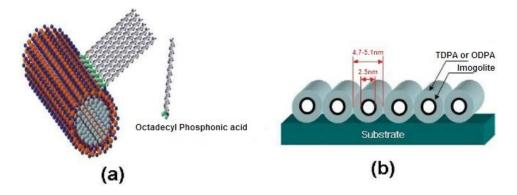
Fig. 6a) chemical structure of octadecyl phosphonic acid modified imogolite (ODPA-imogolite) and b) the dimension of ODPA- or TDPAimogolite on a solid surface [37].
