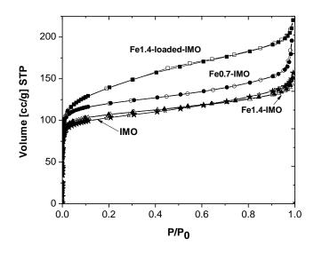
**Fig.11** N<sub>2</sub> adsorption isotherms at -196°C of IMO (stars) and Fe0.7-IMO (circle), Fe1.4-IMO (triangle) and Fe1.49-loaded-IMO (square) outgassed at 250°C. Full and empty symbols refer to adsorption and desorption branches, respectively.
