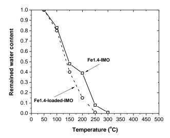
Fig. 4 Normalized physisorbed water concentrations in the SWNT at different heat treatment temperatures as calculated from FT-IR spectra, peak at 1640 cm<sup>-1</sup>
