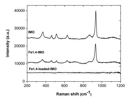
Fig. 9 Raman spectra of IMO, Fe1.4-IMO and Fe1.4-loaded-IMO in 200-1200 cm<sup>-1</sup> region.
