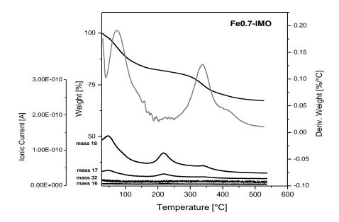
Fig.14 Thermo-Gravimetry (TG) and Differential Thermo-Gravimetry (DTG) curves of Fe-0.025-IMO, as obtained under  $N_2$  atmosphere in the 30-530 °C temperature range combined with quadrupole mass spectroscopy monitoring both  $O_2$  and  $H_2O$  related masses.
