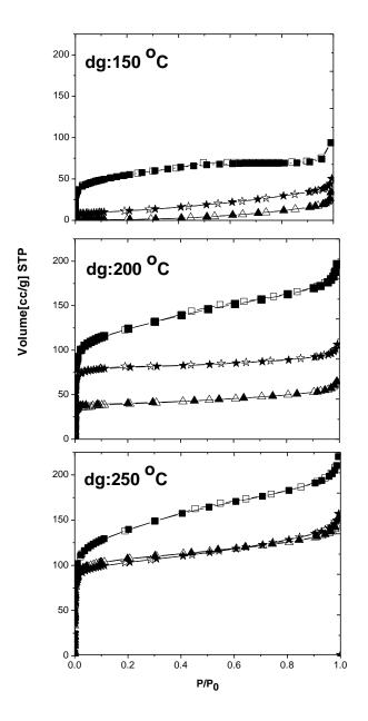
the adsorption/desorption isotherms for IMO, Fe1.4-IMO and Fe1.4-loaded-IMO after degassing at 150, 200 and 250 °C respectively.
