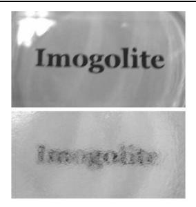
Fig. 15 Transparency of in situ hybrid (upper) and blend (lower) imogolite\PVA films. The thickness of films is ca 100 mm. Imogolite shows to be optically transparent in the multilayer film [286].
