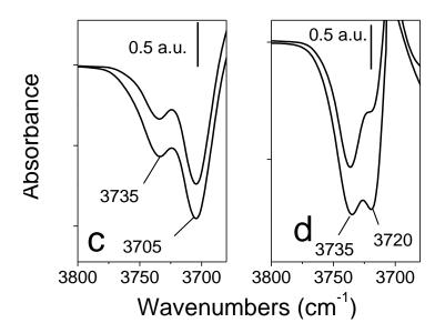
Fig. 8 Difference IR spectra, in the OH stretching region, obtained after dosing  $NH_3$  at r.t. on IMO (a), Fe0.7-IMO (b), Fe1.4-loaded-IMO (c) and Fe1.4-IMO (d) samples that were dehydrated at 250 °C.  $NH_3$  equilibrium pressure corresponding to 2.5 and 10 mbar.
