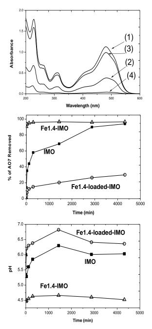
Fig. 14 Section a: UV-Vis spectra of the starting AO7 solution (1) and of the supernatant solutions after 120 min in contact with IMO (2), Fe1.4-loaded-IMO (3) and Fe1.4-IMO (4). Section b: percentage of AO7 removed by IMO (squares), Fe1.4-loaded-IMO (circles) and Fe1.4-IMO (triangles). Section c: pH of the solutions during AO7 adsorption measurements.
