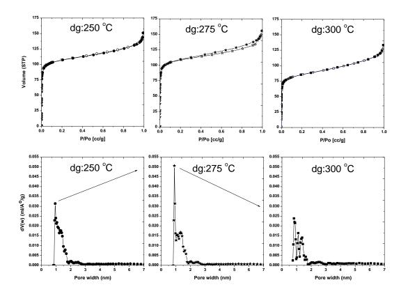
**Fig. 7** upper graphs: N<sub>2</sub> adsorption/desorption isotherms at -196°C of Fe1.4-IMO after degassing at 250, 275, 300 °C. Lower graphs: Correlated NL-DFT Pore Size Distributions of correlated sample degassed at different temperature (250, 275, 300 °C) obtained by applying a N<sub>2</sub>-zeolite kernel to adsorption branches.
