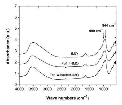
Fig. 5 FTIR spectra of imogolite, Fe1.4-IMO and Fe1.4-loaded-IMO
