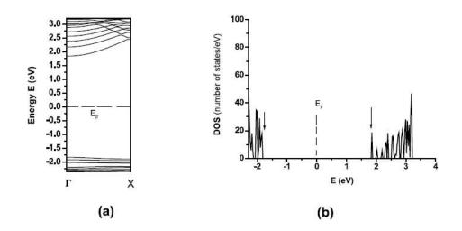
**Fig. 11** The energy bands of the single-walled imogolite nanotube and the electron density of states: (a) the energy bands near the Fermi level, showing the direct and wide energy gap, (b) the total electron density of states [136].
