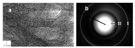
**Fig. 9** a) TEM micrograph of imogolite nanotubes in the interior region of a deposit formed by droplet evaporation in air from 0.1 mg/mL solution. b) SAED pattern of nanotubes. The numbers on the rings correspond to those in Table 1. The diffraction rings are due to the atomic periodicity within the nanotubes [36, 127].
