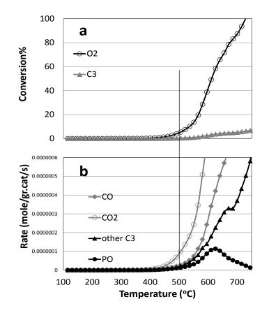
Fig. 12a) Conversion of reactants and b) rate of different products in empty reactor by increasing temperature
