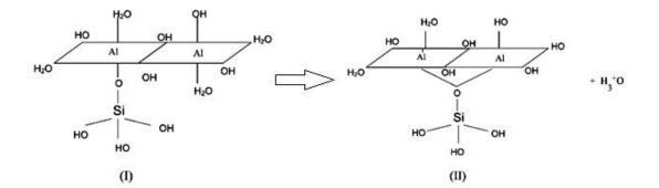
Fig. 2 loss of proton through bridging of aluminums during the polymerization step of imogolite synthesis
