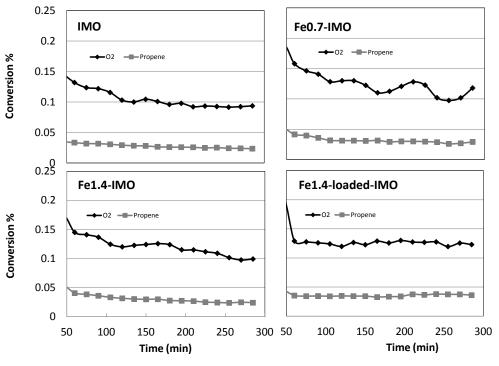
conversion of reactants at 100 °C. Generally the conversion rate of reactants (oxygen and propylene molecules) is extremely low at this temperature.
