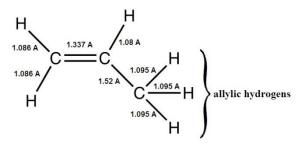
Fig. 3 estimation of Propylene molecule dimension
