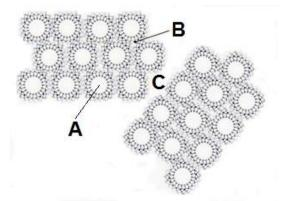
Fig. 8 Type of pores found in imogolite. Hexagonal packing of nanotubes is considered [142].
