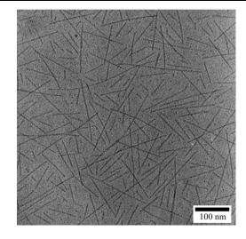
Fig. 10 BF electron micrograph of individually dispersed nanotubes formed by droplet evaporation in ethanol environment from 0.01 mg/mL solution [160].
