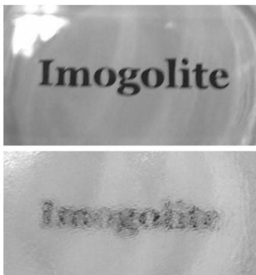
**Fig. 15** Transparency of in situ hybrid (upper) and blend (lower) imogolite/PVA films. The thickness of films is ca 100 nm. Imogolite shows to be optically transparent in the multilayer film [286].
