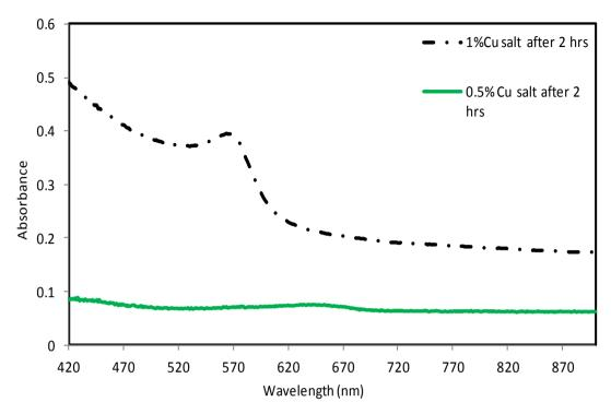
Figure 70 UV-Vis absorption spectra of the crosslinked film containing 1%CuCl<sub>2</sub> and 0.5wt% CuCl<sub>2</sub>, 5%PI, 2%DEA after 2 hrs in an open atmosphere
