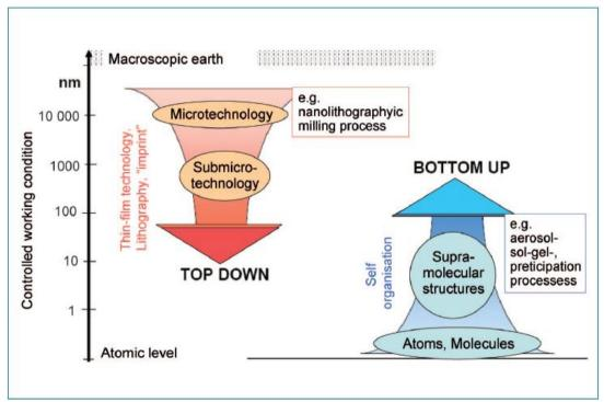
Figure5 Schematic view of Top-Down and Bottom-up technique
