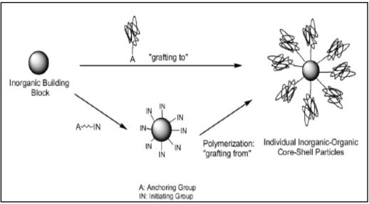
Figure 13 Schematic description of grafting-to and grafting-from approaches<sup>90</sup>
