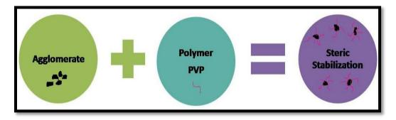
Figure 14 Schematic presentation of steric stabilization mechanism
