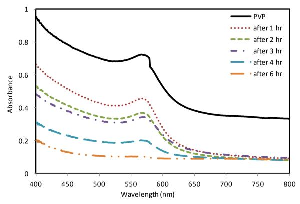
Figure 74 UV-vis spectra of the cross linked films containing 1%CuCl<sub>2</sub>, 5%PI, and 2% DEA in the presence of 0.5% PVP after regular intervals of time
