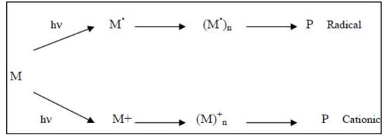
Figure 11 Mechanism of photopolymerization
