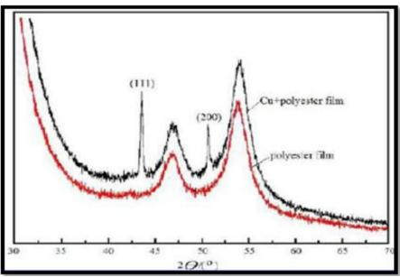
Figure 32 XRD pattern of the copper pattern on the polyester films<sup>50</sup>
