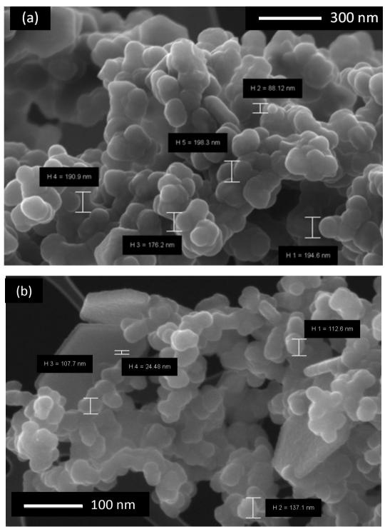
Figure 48 SEM analysis of the ethanol solution containing 10 wt% of AgNO<sub>3</sub> and 2 wt% of pyrrole, (a) with 1%PVP (b) with 2%PVP after 10 minutes of UV-irradiation
