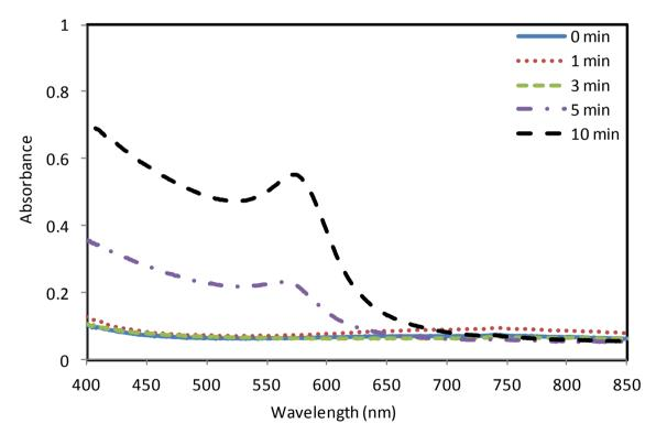
Figure 59 UV-visible spectra of  $CuCl_2$ -amine coordination complex in the presence of 0.5 %( w/v) PVP under UV-irradiation at different times of irradiation
