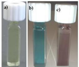
Figure 53 Color change observation: a) CuCl<sub>2</sub>-ethanolsolution, b) CuCl<sub>2</sub>-amine coordination complex, c) CuCl<sub>2</sub>-amine coordination complex after 10 mins UV-irradiation.
