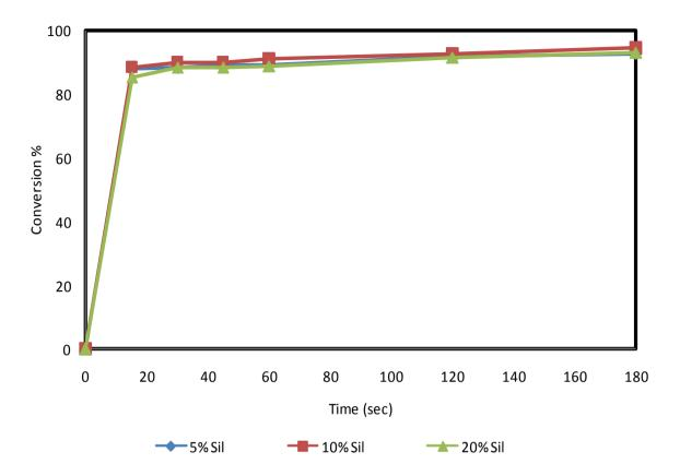
Figure 41 Real time FTIR acrylic group conversion as a function of irradiation time for the PEGDA formulations containing increasing amount of  $AgNO_3$  in the range between 5 - 20wt%.
