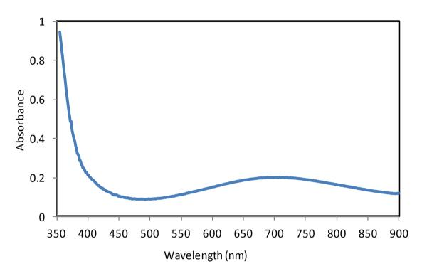
Figure 65 UV-vis absorption spectra of CuCl<sub>2</sub>-amine complex before UV-irradiation
