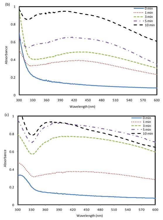
Figure35 UV-Vis spectra of the ethanol solution containing 5 wt% (a), 10 wt% (b) and 20 wt% (c) of AgNO<sub>3</sub>. All the solutions contained 2 wt% of pyrrole and the radical photoinitiator 0.002%PI.
