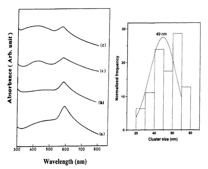
Figure (26-a) UV-vis spectra of copper nanoparticles in the presence of 5exp-3 M CuSO<sub>4</sub>, 2exp-1N 2-propanol, in different concentrations of PVA, (a) 0.79, (b) 1.5, (c) 2.3, (d) 3.4exp-2 M. (23-b) Histogram of Cu particles in the presence of 5exp-3 M CuSO<sub>4</sub>, 2exp-1N 2-propanol, 3.4 exp-2 M PVA<sup>211-a</sup>
