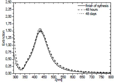
Figure 22 UV-vis spectra of stabilized silver nanoparticles after 48 hours and after 48 days<sup>232</sup>
