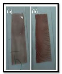
Figure 67 Color change observed in a freshly prepared film containing a)  $0.5wt\%CuCl_2$ , b)  $1wt\%CuCl_2$
