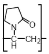
Figure 15 Structure of the repeat unit of PVP
