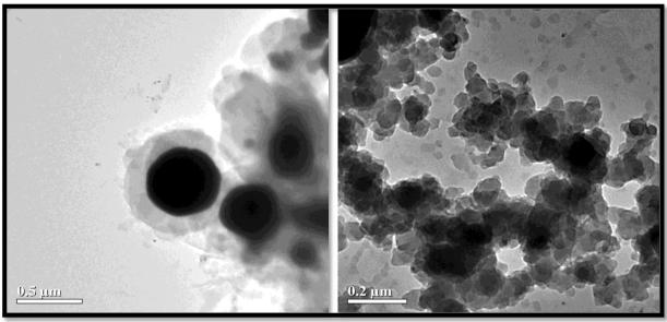
Figure 40 TEM analysis of the ethanol solution containing 5 wt% of AgNO<sub>3</sub> and 2 wt% of pyrrole, after 10 minutes of UV-irradiation.
