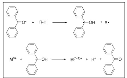
Figure 9 Photoreduction of Benzophenone followed by electron transfer to the metal ion  $M^{n+}$
