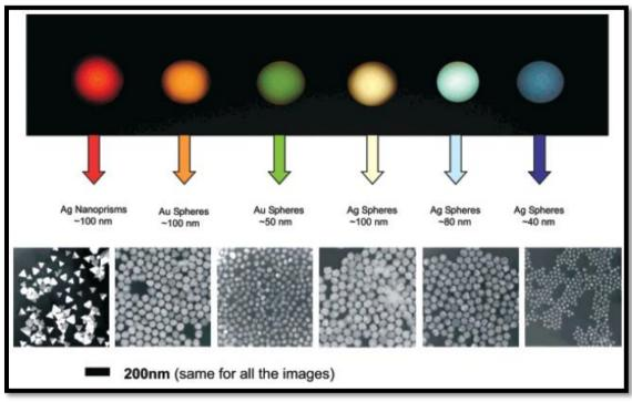
Figure 3 Sizes, shapes and composition of metal nanoparticles can be systematically varied to produce materials with distinct light-scattering properties<sup>27</sup>.
