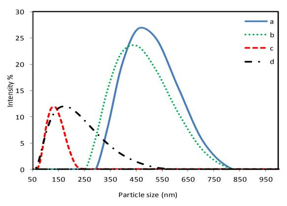
Figure 64 Particle size distribution from DLS (a) CuCl<sub>2</sub>-amine coordination complex (b) CuCl<sub>2</sub>-amine coordination complex in presence of 0.2wt%Py (c) CuCl<sub>2</sub>-amine coordination complex in presence of 0.5wt%PVP. (d). CuCl<sub>2</sub>-amine coordination complex in presence of 0.5wt%PVP in the presence of 0.4% Na-ascorbate
