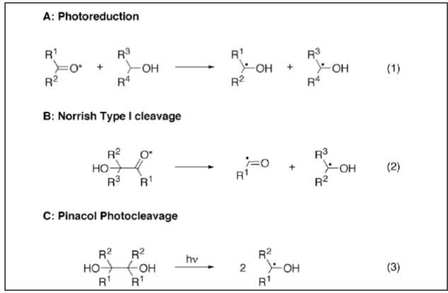
Figure 7 Photochemical strategies for the generation of ketyl radicals from organic precursors. The asterisk (\*) denotes the excited state of a molecule, frequently a triplet state in the examples used in this contribution, while "hv" indicates exposure to light<sup>67</sup>.
