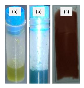
Figure 73 Change in color observed (a)  $CuCl_2$ -amine coordination complex in PEGDA, (b) in the presence of 0.5 %( w/w) PVP, (c) Crosslinked film in the presence of 0.5 %( w/w) PVP,
