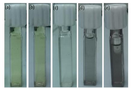
Figure 51 Color change observation of CuCl<sub>2</sub>-ethanol solution a) before UV, (b) 1mins, (c) 3mins, (d) 5mins, (e) after 10mins of UV-irradiation.
