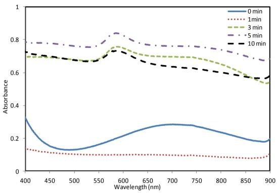
Figure 54 UV-visible spectra of copper chloride-amine coordination complex under UVirradiation at different times.
