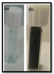
Figure 55 Color change observation: a) CuSO<sub>4</sub>-amine coordination complex bf UV, b) CuSO<sub>4</sub>amine coordination complex after 10 mins UV-irradiation.
