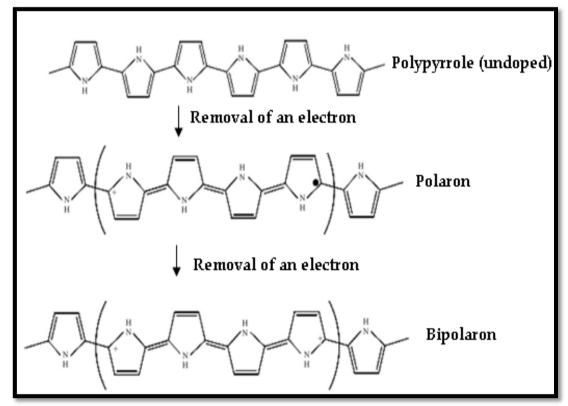
Figure 30 Conduction mechanisms in Polypyrrole<sup>97-b</sup>
