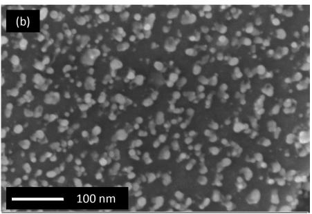
Figure 43 FESEM image of the fracture surface of the crosslinked films a) 10wt% AgNO $_3$  b) 20%AgNO $_3$
