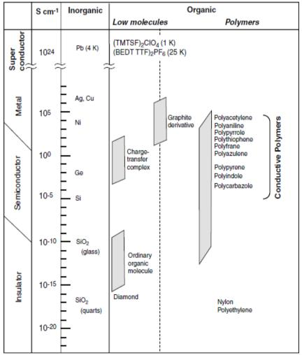
Figure 29 Conductivities of different materials (conductors, semi-conductors, insulators and superconductors) with comparison with the conducting polymers.<sup>96-c</sup>
