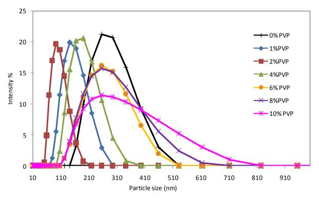
Figure 47 DLS-images of diameter distribution by intensity of nanosized silver colloids with different PVP concentrations after 10mins UV-irradiation.
