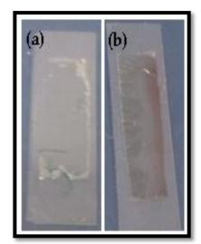
Figure 69 Color change observed in a film after 2 hrs containing a) 1wt%CuCl<sub>2</sub>, b)  $0.5wt\%CuCl_2$
