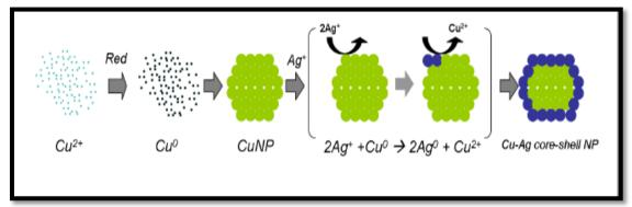
Figure 16 Schematic illustration of Cu-Ag core shell NP<sup>183</sup>
