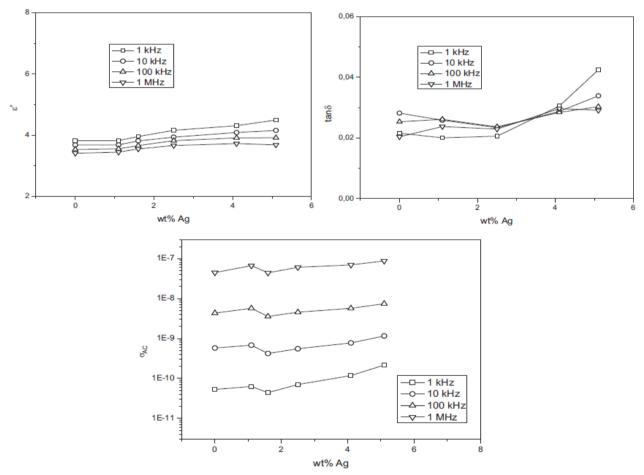
Figure 28 Evolution of dielectric constant,  $tan\delta$  and AC conductivity with nanoparticle content at room temperature and several frequencies ranging from 1 kHz to 1 MHz<sup>275</sup>
