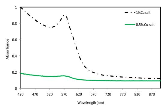
Figure 68 UV-Vis absorption spectra of the crosslinked film freshly prepared containing 0.5wt% and 1wt%CuCl<sub>2</sub>, 5wt%PI, 2wt%DEA
