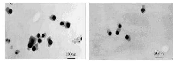
Figure 23 TEM image of silver/polypyrrole core shell nanoparticles<sup>22</sup>
