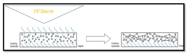
Figure 10 Schematic illustration of photopolymerization process
