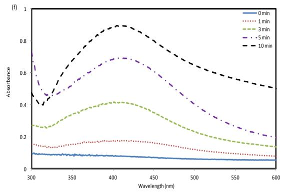
Figure 46 UV-Vis spectra of the ethanol solution containing 10 wt% of AgNO<sub>3</sub>+2 wt% of pyrrole and the radical photoinitiator 0.002%PI. (12a) 1%PVP (b) 2%PVP and (c) 4%PVP (d) 6%PVP (e) 8%PVP (f) 10% PVP
