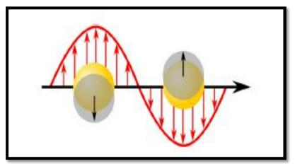
Figure 17 Effect of optical field on the electron cloud in a spherical metal nanoparticle<sup>191</sup>
