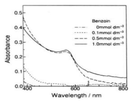
Figure 24 Change in the UV-vis absorption spectra of (Cu  $(ClO_4)_2$ ) in an ethanol solution irradiated for 60 mins<sup>230</sup>
