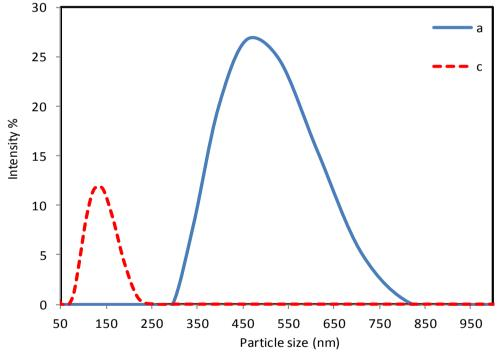
Figure 60 DLS images of diameter distribution by intensity of copper colloids (a) CuCl<sub>2</sub>amine coordination complex (c) CuCl<sub>2</sub>-amine coordination complex in the presence of 0.5 %(w/v) PVP
