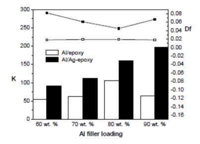
Figure 27 Dielectric properties of Al/epoxy and Al/Ag-epoxy composites with different Al filler loading<sup>95</sup>
