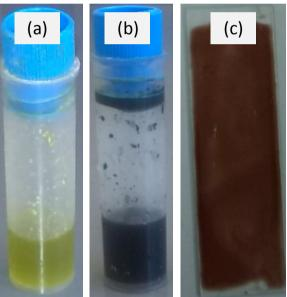
Figure 71 Change in color observed (a)  $CuCl_2$ -amine coordination complex in PEGDA, (b) in the presence of 0.2 %( w/w) pyrrole, (c) Freshly prepared crosslinked film in the presence of 0.2 %( w/w) pyrrole
