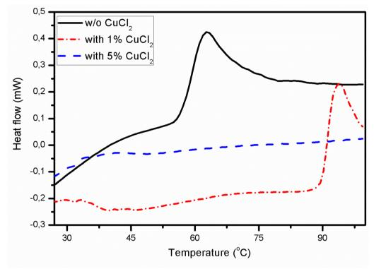
Figure 66 DSC curves of samples without  $CuCl_2$  and the samples containing 1wt% and 5wt%  $$CuCl_2$.$
