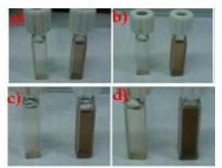
Figure 34 Color change observed after a) 1 min, b) 3 min, c) 5 min d) 10min of UVirradiation. [10%AgNO<sub>3</sub>+ 2%Py+ 0.002%PI].
