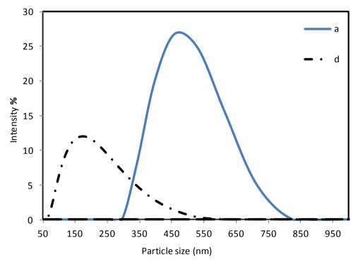
Figure 63 DLS images of diameter distribution by intensity of copper colloids (a) CuCl<sub>2</sub>amine coordination complex (d) CuCl<sub>2</sub>-amine coordination complex in the presence of 0.02M Sodium L-ascorbate and 0.5%(w/v) PVP
