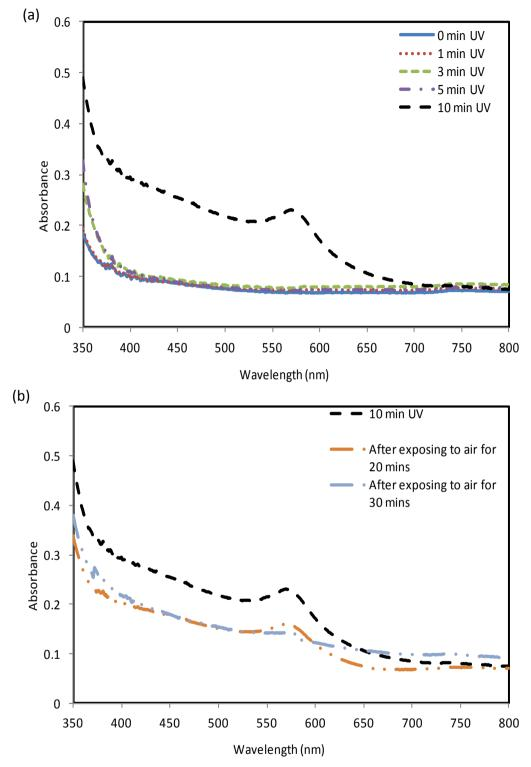
Figure 62(a) UV-vis spectra of CuCl<sub>2</sub>-diethanol amine coordination complex in the presence of 0.02MSodium L-ascorbate and 0.5%(w/v) PVP for different intervals of time.(b) same solution after exposing to open air.
