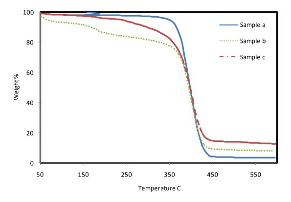
Figure 45 Thermograms of Samples: Sample-a (PEGDA+2wt%PI), Sample-b (PEGDA+10wt%AgNO<sub>3</sub>+2wt%PI), Sample-c (PEGDA+20wt%AgNO<sub>3</sub>+2wt%PI)
