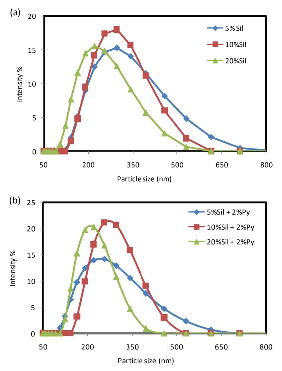
Figure 39 DLS-images of diameter distribution by intensity of nanosized silver colloids (a) with 5wt%, 10wt%,  $20wt\%AgNO_3 w/o$  (Py)pyrrole (b) with 5wt%, 10wt%,  $20wt\%AgNO_3 w/o$  (Py) after 10mins UV-irradiation
