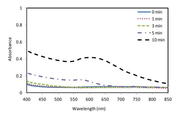
Figure 57 UV-visible spectra of CuCl<sub>2</sub>-amine coordination complex in the presence of 0.2 %( w/v) pyrrole under UV-irradiation at different times of irradiation.
