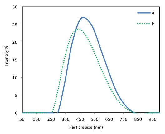
Figure 58 DLS images of diameter distribution by intensity of copper colloids (a)  $CuCl_2$ amine coordination complex (b)  $CuCl_2$ -amine coordination complex in the presence of 0.2 %( w/v) pyrrole
