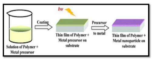
Figure 33 Block Diagram of the UV-curing process
