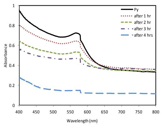
Figure 72 UV-vis spectra of the cross linked films containing 1%CuCl<sub>2</sub>, 5%PI, and 2% DEA in the presence of 0.2% pyrrole after regular intervals of time
