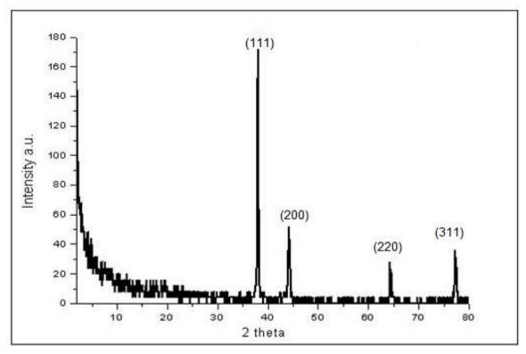
Figure 38 XRD analyses of the ethanol solution containing 5 wt% of AgNO $_3$  and 2 wt% of pyrrole, after 10 minutes of UV-irradiation
