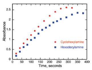
Figure 19 Growth of absorbance band by UV-irradiating silver trifluoroacetate in the presence of cyclohexylamine and hexadecylamine<sup>231</sup>
