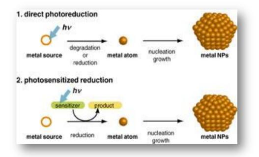
Figure 6 Schematic system of photo-induced synthesis of metal nanoparticles<sup>63</sup>
