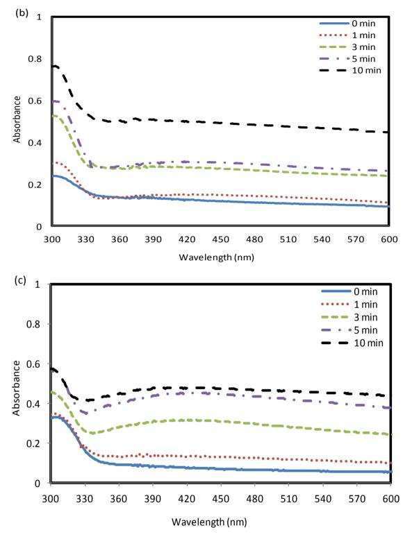
Figure37 UV-Vis spectra of the ethanol solution containing 5 wt% (a), 10 wt% (b) and 20 wt% (c) of AgNO<sub>3</sub> and the radical photoinitiator.
