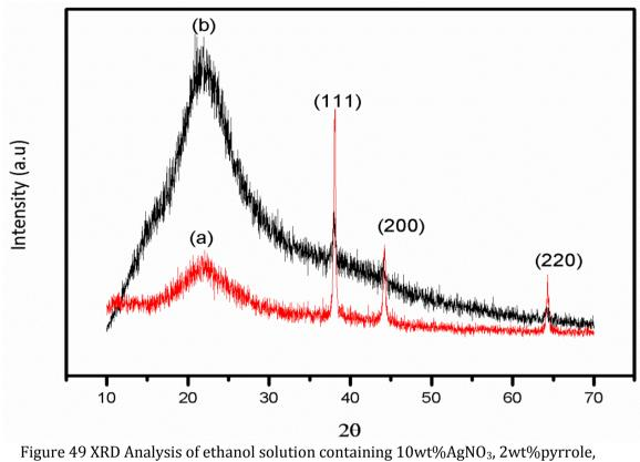
0.002%PI and (a) 6wt% PVP (b)4wt%PVP UV-irradiated for 10 mins.
