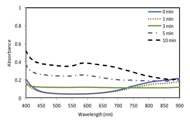
Figure 52 UV-vis spectra of  $CuCl_2$  ethanol solution under different irradiation times.
