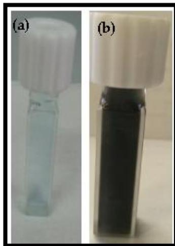
Figure 55 Color change observation: a)  $\text{CuSO}_4$ -amine coordination complex before UV, b)  $\text{CuSO}_4$ -amine coordination complex after 10 mins UV-irradiation.
