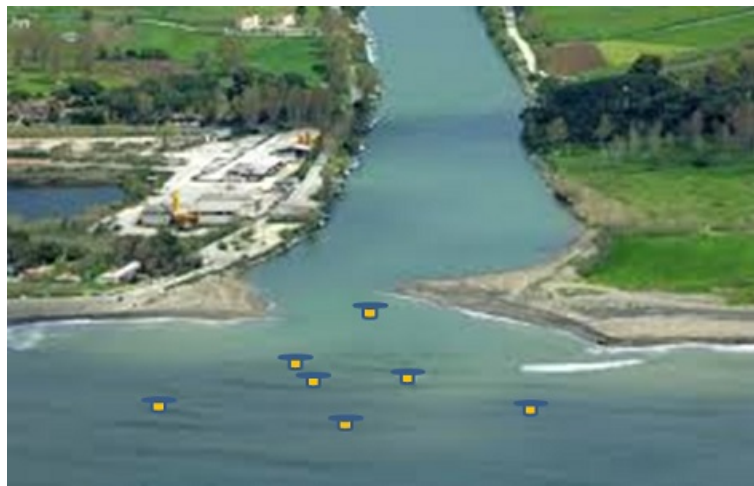
Figure 1. Example of application of the described WSNs of probes. It can be used to monitor the water at the mouth of a river.
