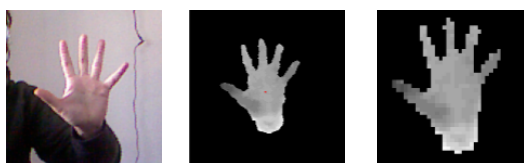
Figure 6. Hand segmentation, computation of the palm center and generation of the re-coded depth map to be used for querying the pose database: (a) image observed by the sensor; (b) segmented depth map; and (c) 40 \times 40 pixel re-coded map.
