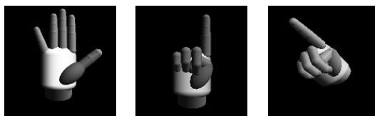
Figure 5. 3D hand model used for generating the reference poses (three configurations are shown, obtained by working on a subset of the possible DOFs).
