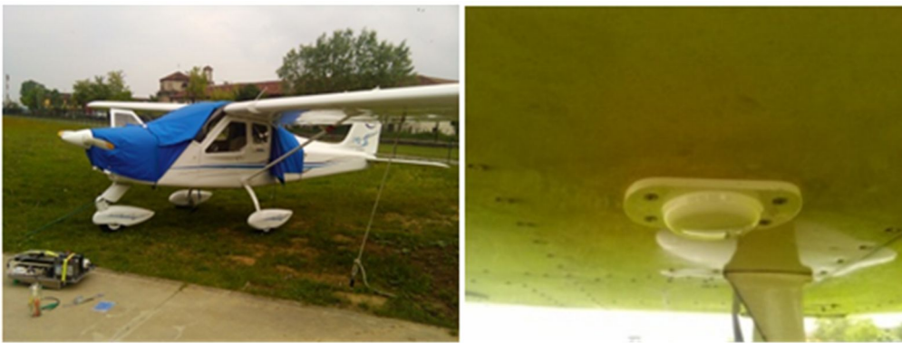
Figure 5-3 The aircraft used (left panel) and down-looking LHCP antenna (right panel)
