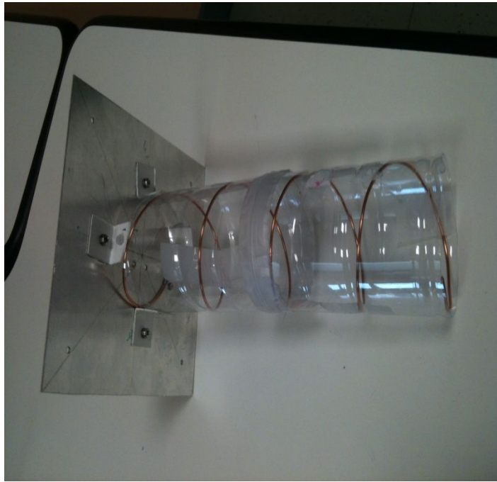
Figure 3-1 Built helix antenna with 4 turns
