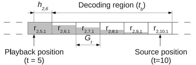
Fig. 3. Sample status of node  $\mathcal{N}_j$ , for  $j = 2$  and  $S = 1$ . The source seeds generation  $t = 10$ , the node plays out generation  $t = 5$  and buffers generations  $t \in [6, 10]$ . Next played out generation ( $t = 6$ ) deadline is  $h_{2,6}$ .
