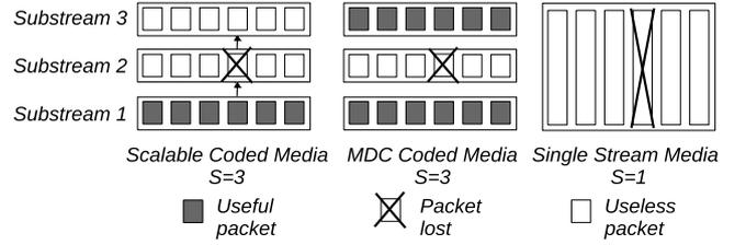
Fig. 1. Media stream model for single stream media, multiple-descriptions and scalable-coded media streams as a stack of substreams for one generation  $T = 1$ . Decoding dependencies between substreams are illustrated with arrows.
