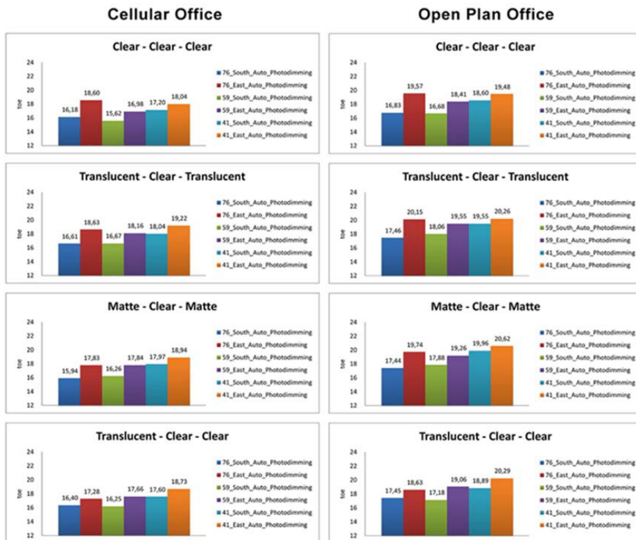
Fig. 6. Variation of the EP_{gl} values as a function of orientation vs. glazing type and façade lay-out (step III).
