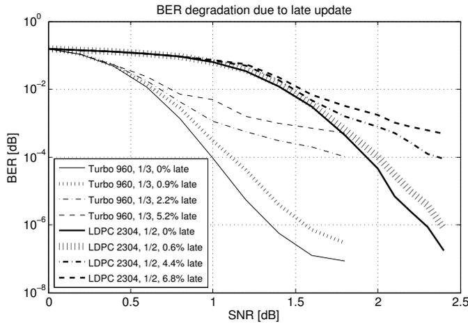
Fig. 4 BER degradation due to late information update
