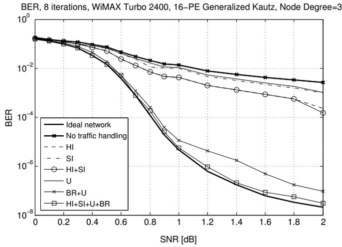
Fig. 6 Impact of the proposed techniques and their combinations - turbo codes
