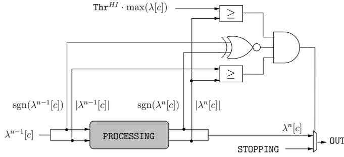
Fig. 10 HI implementation for LDPC codes - STOPPING message
