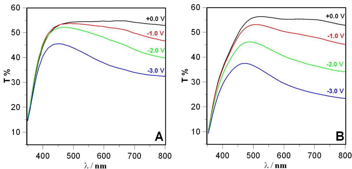
**Figure 8.** Typical UV-VIS transmittance spectrum of  $WO_3/PE/V_2O_5$  ECD at different values of applied potential. Each spectrum was registered after biasing for 60 seconds the ECD at the selected potential ranging from 0 to -3 V vs.  $V_2O_5$  electrode. (A section) EC-DEC as solvent; (B section) RTIL as solvent. Electrodes configuration:  $WO_3$  as Cathode and Working Electrode;  $V_2O_5$  as Anode, Counter and Reference Electrode.
