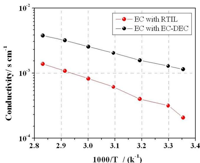
**Figure 5.** Arrhenius plot showing the Ionic conductivity of polymer electrolyte membrane based on the reactive formulation containing BEMA /PEGMA (composition 20 %/ 10 % w:w) RTIL or EC-DEC (57% w:w) and LiTFSi (10 % w:w) between  $25^\circ\text{C}$  and  $80^\circ\text{C}$ .
