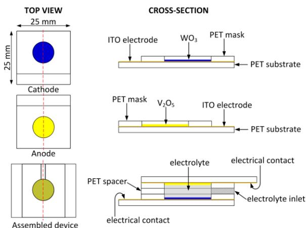
**Figure 4.** General Assembly of the prepared electrochromic devices.
