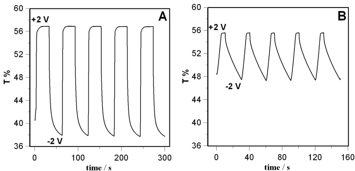
**Figure 7.** Typical time plot of  $T\%(700\text{ nm})$  during repeated switching between bleached and colored state for a  $WO_3/PE/V_2O_5$  ECD. (A section) EC-DEC as solvent; (B section) RTIL as solvent. Potential program:  $E_1 = +2$  V,  $E_2 = -2$  V;  $t_1 = t_2 = 20$  s. Potentials are vs.  $V_2O_5$  electrode. Electrodes configuration:  $WO_3$  as Cathode and Working Electrode;  $V_2O_5$  as Anode, Counter and Reference Electrode.
