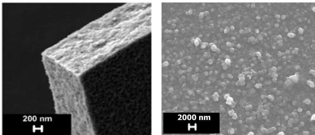
**Figure 2.** (Left) SEM picture showing the typical aspect and surface morphology of the  $\text{WO}_3$  film inkjet-printed on ITO-PET substrates; (Right) SEM image showing the template-mediated micro-porous structure of electro-deposited  $\text{V}_2\text{O}_5$  thin films on ITO (Adapted from Reference 25).
