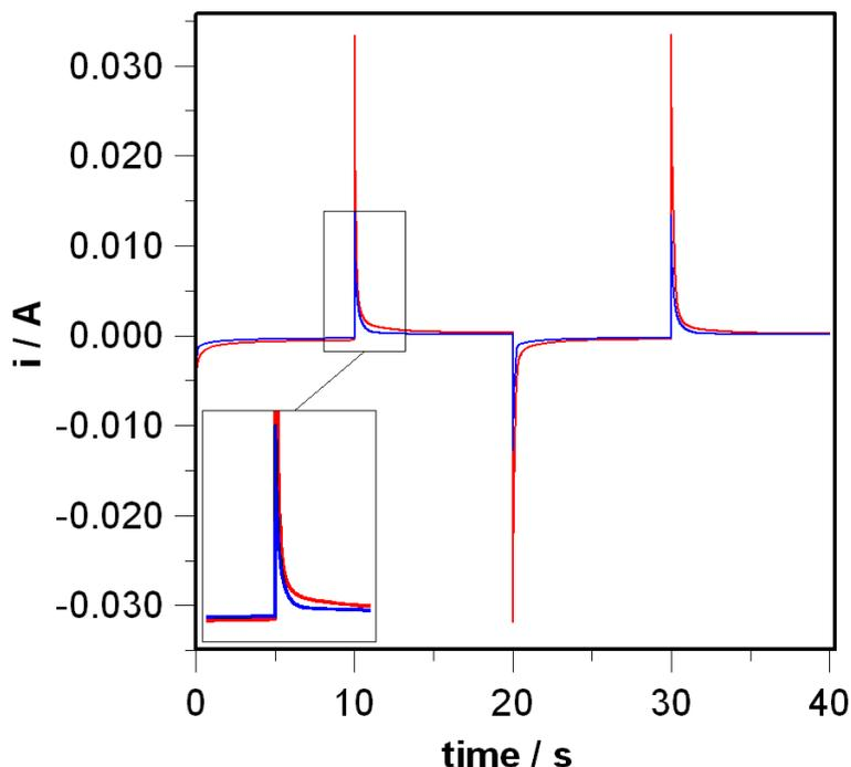
**Figure 6.** Chronoamperometric profiles of WO<sub>3</sub>/PE/V<sub>2</sub>O<sub>5</sub> ECD with methacrylate based electrolytes. (blue curve) RTIL as solvent; (red curve) EC-DEC 1:1 as solvent. Potential program:  $E_1 = -2.0$  V,  $E_2 = +2.0$  V.  $t_1 = t_2 = 10$  s. Potentials are vs. V<sub>2</sub>O<sub>5</sub> electrode.
