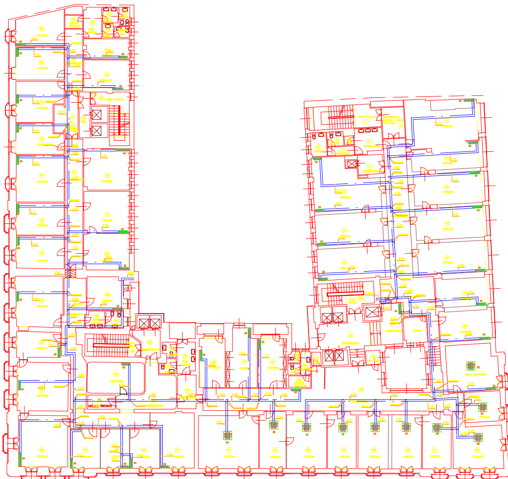
Plan of the fourth floor, in blue the VRF tubes circuit
