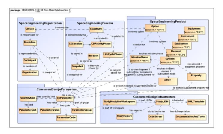
Figure 6.21: SEIM main information object types and relationships (informal UML class diagram), [61].
