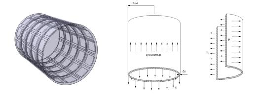
Figure 8.3: Simplified representation of the primary structure considered in the reference case.
