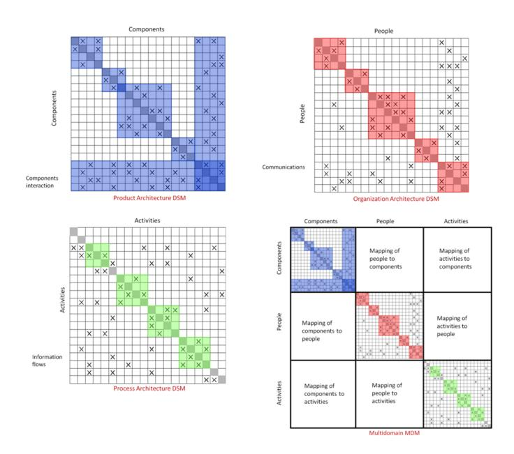
Figure 4.2: Examples of DSM concerning Product Architecture, Organization Architecture, Process Architecture and Multidomain matrix [36].
