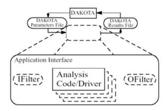
Figure 4.13: Components of the simulation interface [98].
