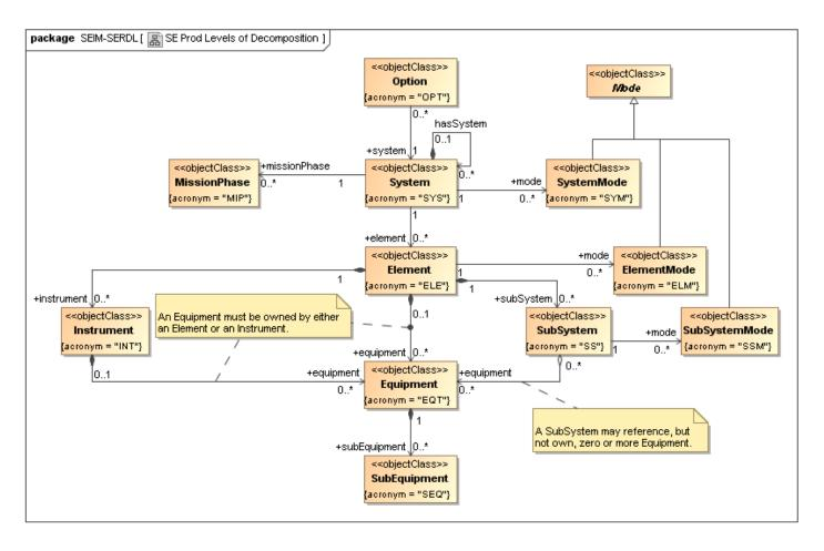
Figure 6.22: SEIM system decomposition and associated modes (UML class diagram), [61].
