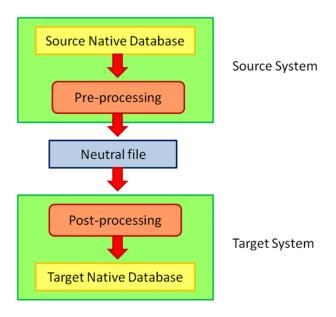
Figure 6.19: Data exchange mechanism.
