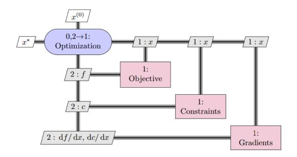
Figure 4.3: Simple example of gradient-based optimization process [35].
