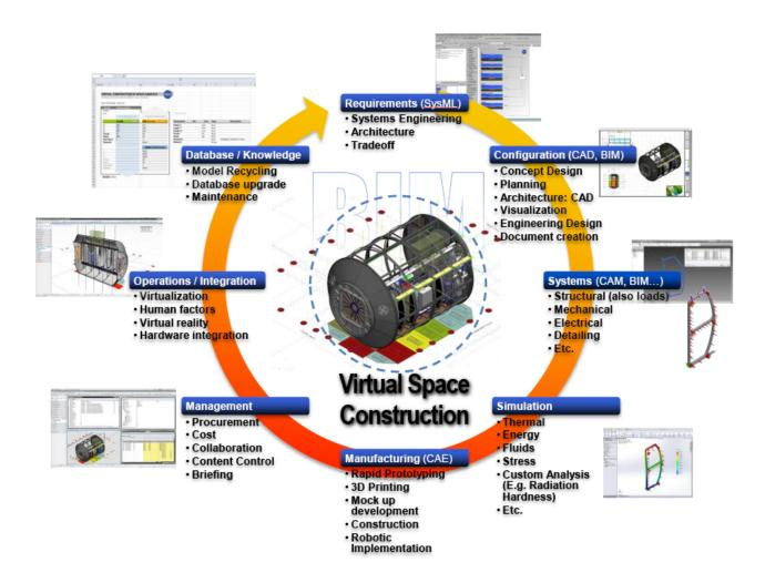
Figure 5.3: Conceptual overview of the lifecycle of an aerospace system and the phases that can be covered with the proposed Virtual Space Construction Process (VSC) [119].
