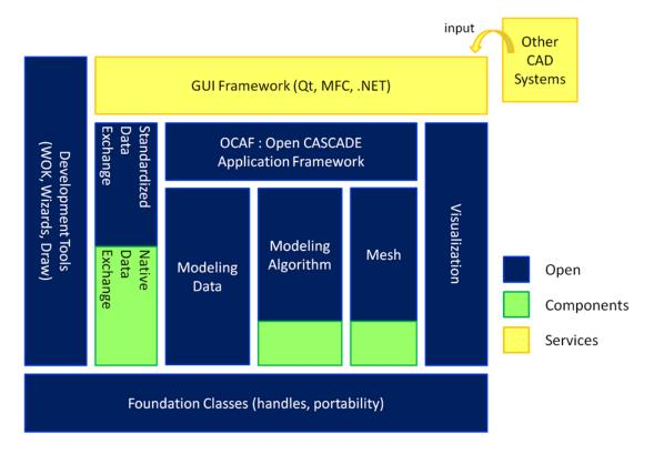
Figure 9.1: Modular structure of Open CASCADE platform [94].
