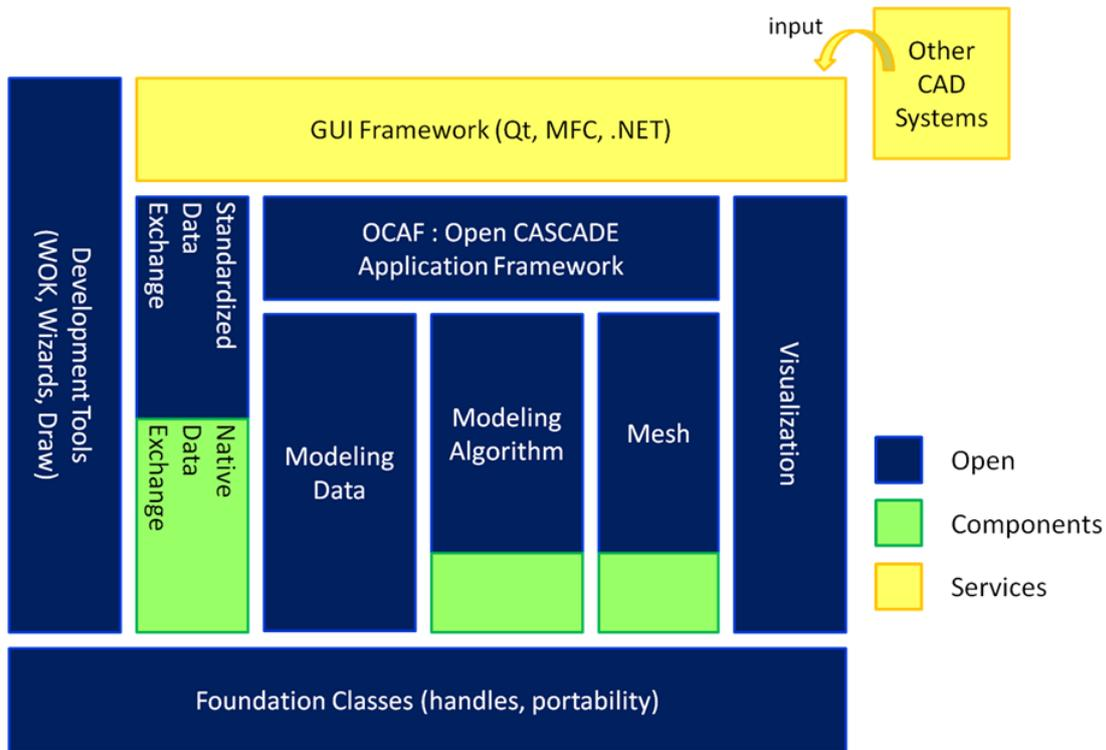
Figure 9.1: Modular structure of Open CASCADE platform [94].
