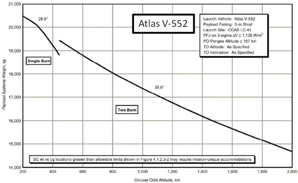
Figure 8.2: Example of payload capability expressing the mass as function of the altitude.
