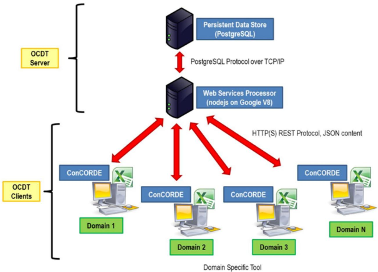
Figure 3.8: Open Concurrent Design Tool (OCDT) architecture overview.
