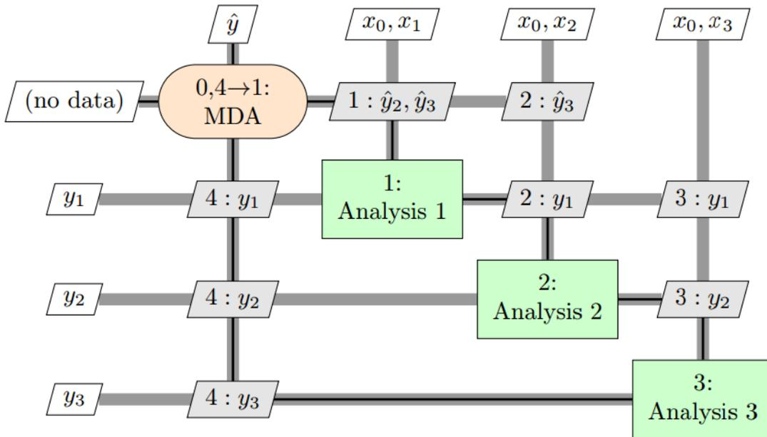
Figure 4.4: Gauss-Seidel MDA architecture for three coupled analyses [35].
