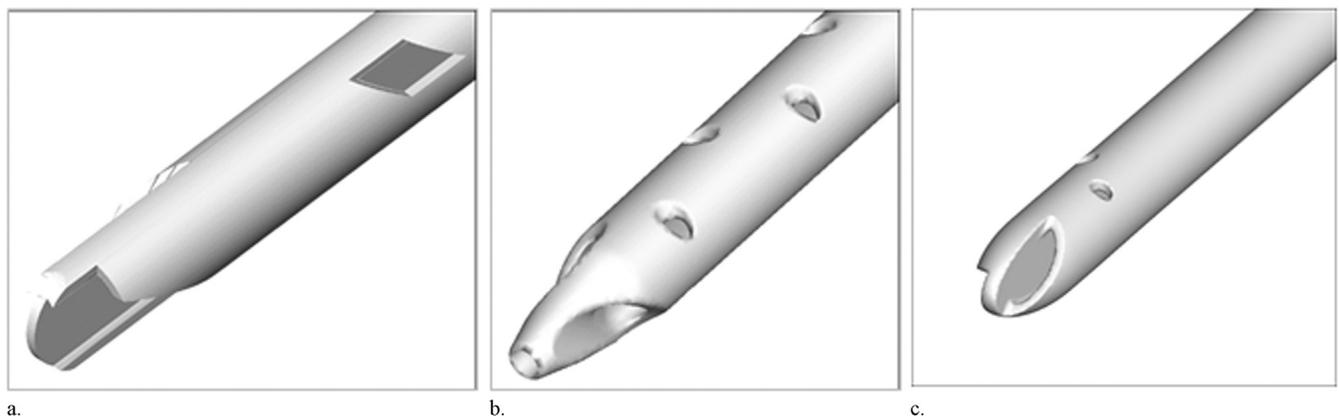
**Figure 1.** Three-dimensional computer-aided design models of the Palindrome (a), GlidePath (b), and VectorFlow (c) catheters before tetrahedral/hexahedral meshing for analysis using CFD. The Palindrome catheter is completely symmetric. The GlidePath catheter is not perfectly symmetric; it has a guide wire aperture at the distal tip as part of the venous lumen, as well as offset side holes. The VectorFlow catheter has complete symmetry of its distal tip but offsetting of its side holes.
