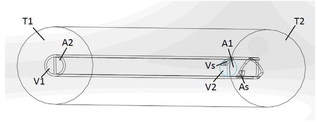
**Figure E1.** Conditions applied at the permeable boundaries. Schematics of the virtual bench test setup for Palindrome model (representation is not to scale). T1 and T2 are tube inlet and tube outlet, V1 and V2 are the venous inlet and outlet, and A2 and A1 are arterial inlet and outlet, respectively. Vs and As represent the venous and arterial side holes.
