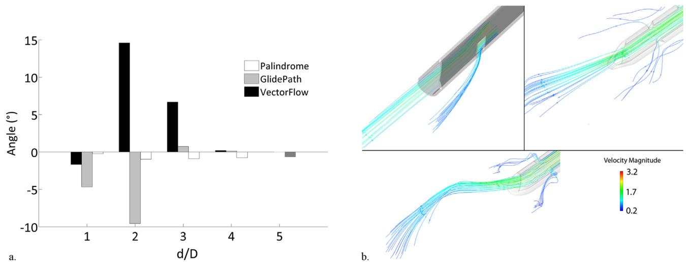
**Figure 5.** (a) Mean angle deflection of flow pathlines at a distance of one to five SVC diameters downstream of the distal tip of the catheter in forward configuration. (b) Representation of blood streamlines exiting venous lumen in Palindrome, GlidePath, and VectorFlow catheters colored by velocity magnitude (in meters per second).
