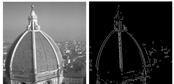
(e) Latent image restored by ABLUR (f) Edges extracted from de-blurred image
