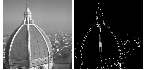
(e) Latent image restored by ABLUR (f) Edges extracted from de-blurred image
