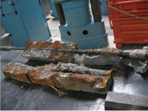
Fig. 3. Demolishing of the concrete specimen and cleaning of the reinforcing bar.
