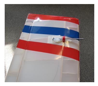
Fig. 7.17: Pitot installation on the Ultrastick 25e right wing
