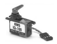
Fig. 3.9: GWS IQ-100 analog servo.
