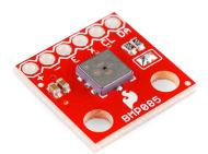
Fig. 7.3: Bosch BMP085 barometric sensor on Sparkfun breakout board
