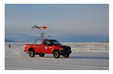
Fig. 2.2: Aerosonde Mark 4.7 UAV for Antartic climate studies [14].
