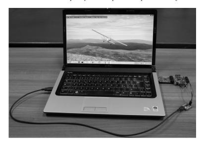
Fig. 6.16: FlightGear HIL setup
