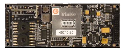
Fig.~4.6: MicroPilot MP2028 autopilot [109]
