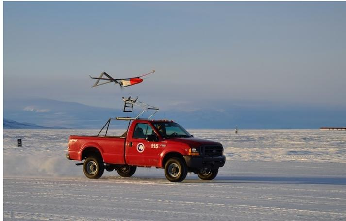
*Fig. 2.2: Aerosonde Mark 4.7 UAV for Antartic climate studies [14].*
