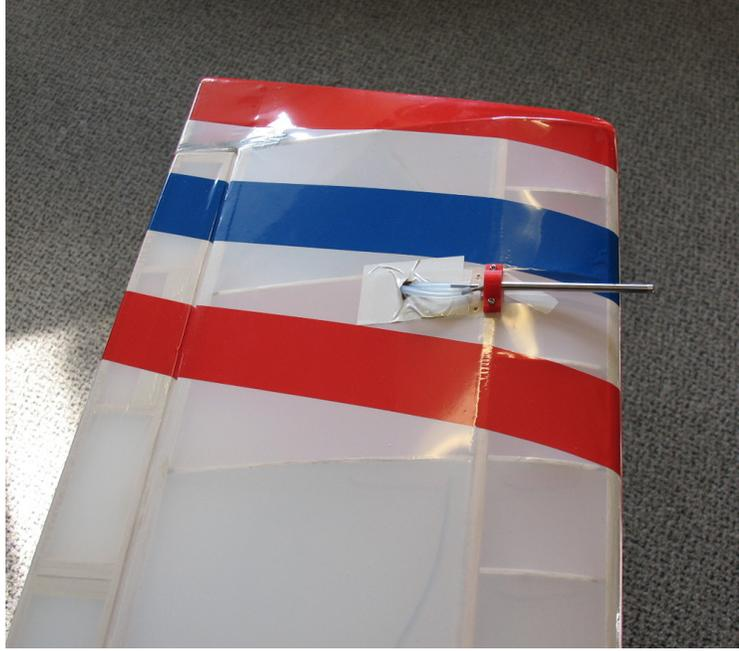
*Fig. 7.17:* Pitot installation on the Ultrastick 25e right wing
