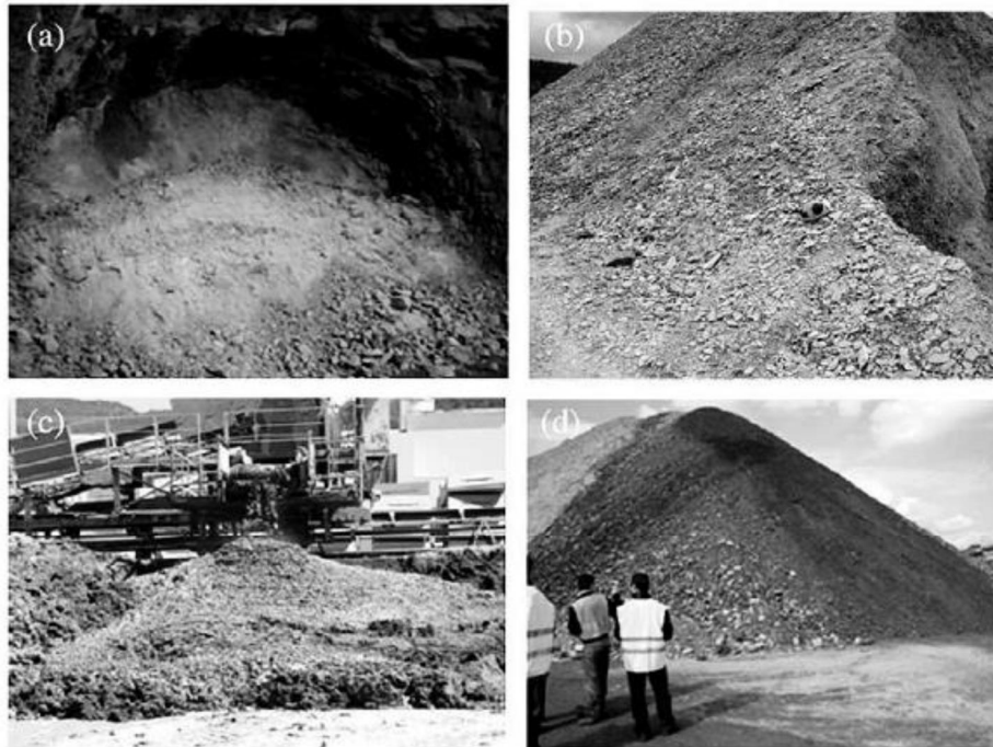
Fig. 1. Examples of tunnel spoil types. (a) Granitic rock, Drilling and Blasting in large-section road tunnel (Omegna Tunnel, Italy); (b) Granitic rock, full face TBM in small-section exploratory drift (Aica-Mules Tunnel, Italy); (c) Soft rock-hard soil, full face excavation and soil conditioning for large-section highway tunnel (Sparvo Tunnel, Italy); (d) Coarse soil, mechanised excavation for railway tunnel (Turin Railway "Passante", Italy). (Oggeri et al., 2014)
