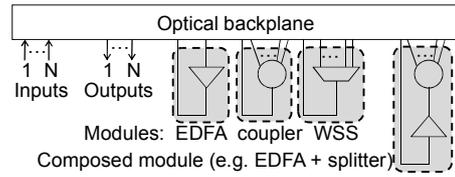
Fig. 1: Network function programmable (NFP) node
