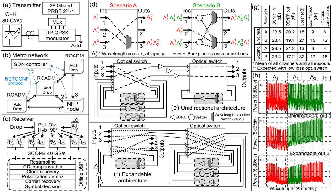
**Fig. 4:** (a) Transmitter, (b) metro network and (c) receiver setups for the validation of the NFP in (d) two scenarios using (e) the unidirectional and (f) the expandable backplane architectures. (g) Summary of results and (h) spectra at input 1 and outputs 1 and 3 for the unidirectional and expandable architectures respectively in scenario B.
