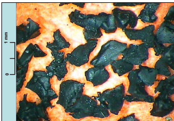
C 0.4-0.7 ("standard", ambient size reduction) Satisfactory degree of cleanliness
