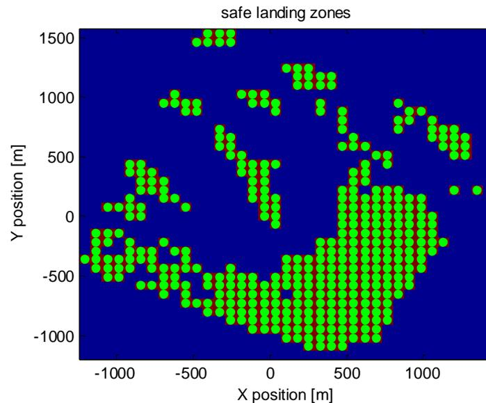
Figure 21. Safe landing pixels of the ASM in
