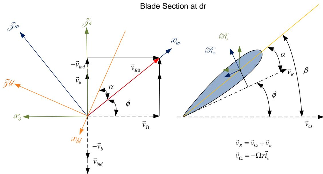
Figure 57. Geometry of a propeller Blade element
