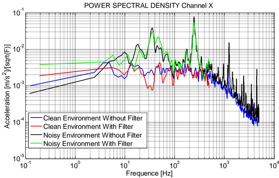
Figure 53. Accelerometer PSD (Channel X)
