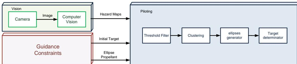
Figure 29. Piloting Scheme
