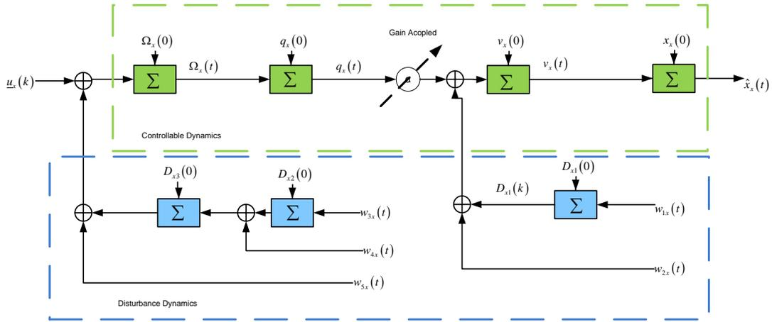
Figure 72. **Diagram Block of the Horizontal EM**
