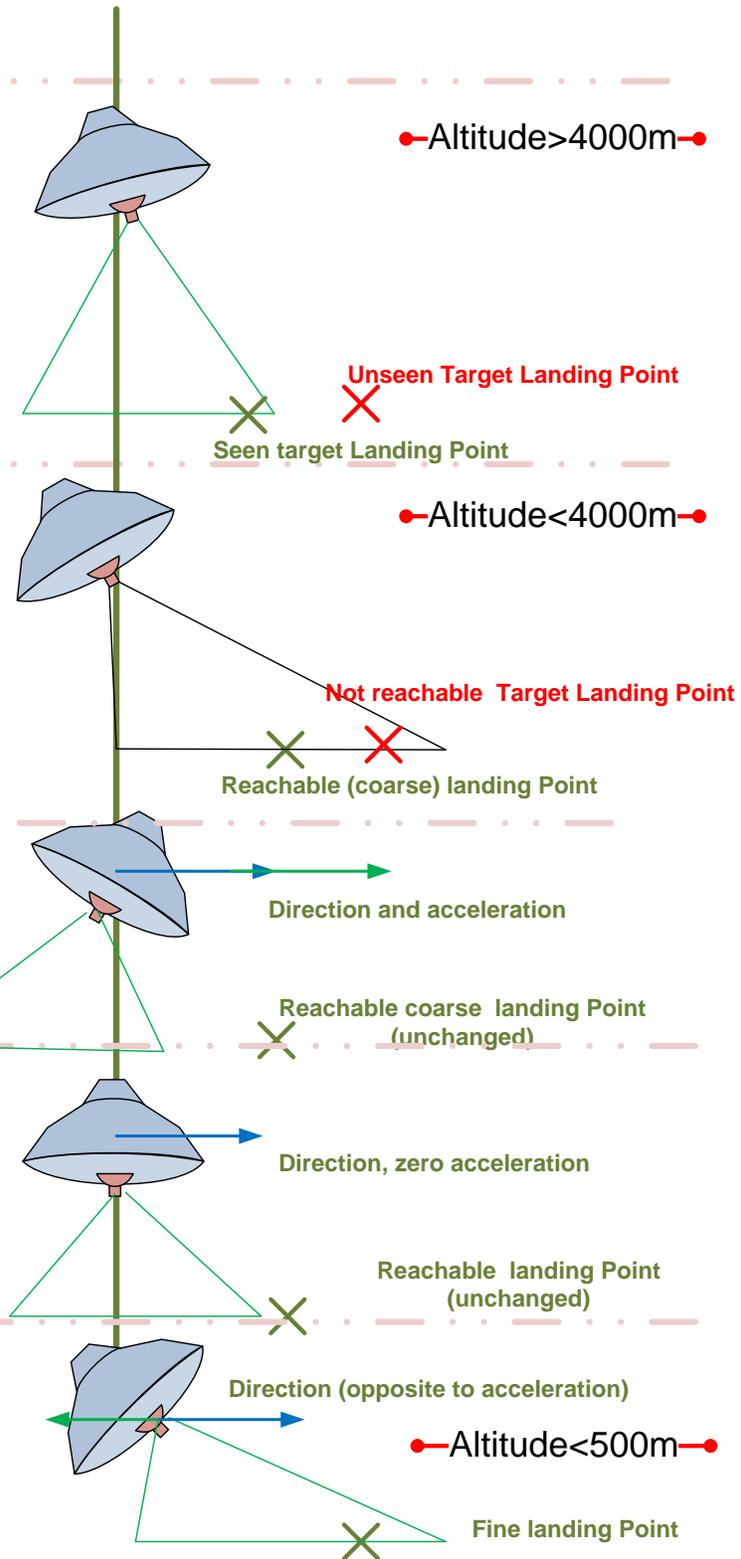
Figure 15. Phases of the landing site algorithm.
