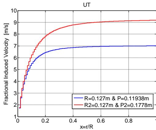
Figure 58. **Fractional Induced Velocity**  $v_{ind}$  **along the blade**
