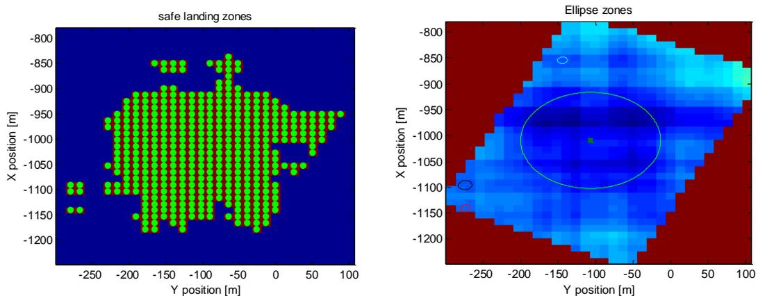
Figure 41. Target selection based landing ellipse (Height 201m)
