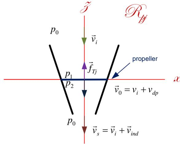
Figure 55. Axial wind flow through the propeller
