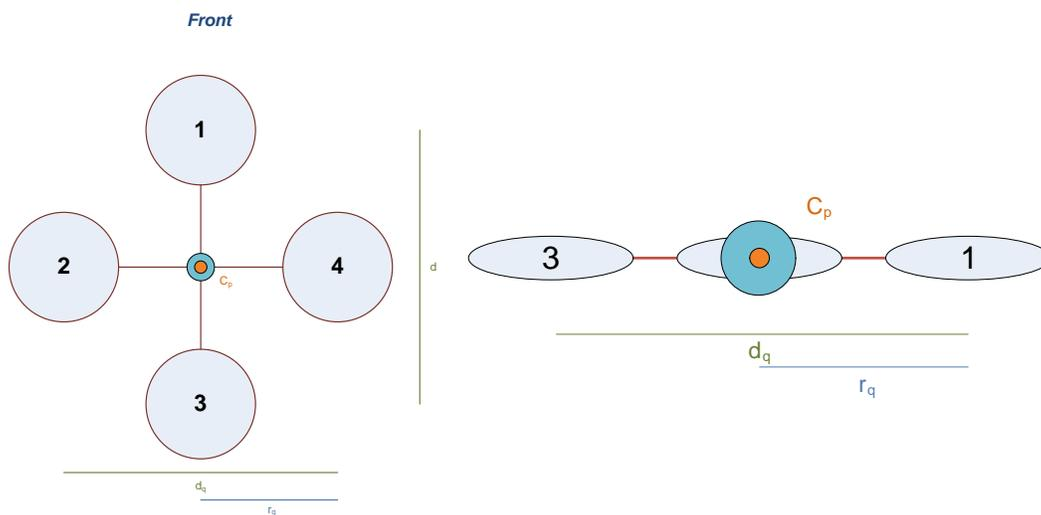
Figure 43. Quadcopter Left: Up view Right: Side Views
