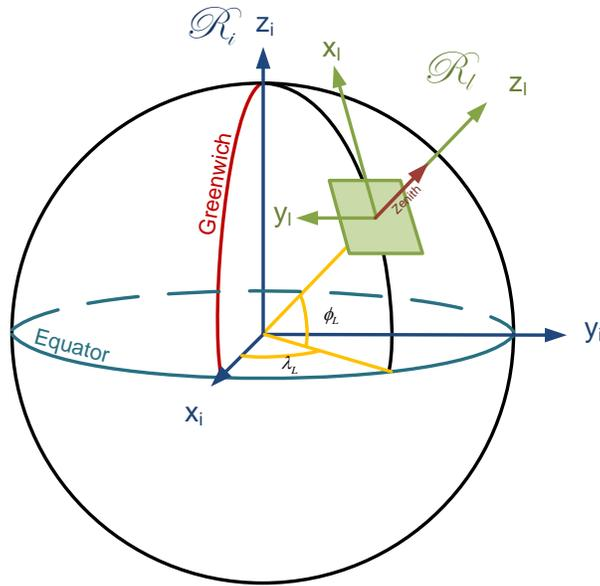
Figure 44. **Inertial and Local frames of references**
