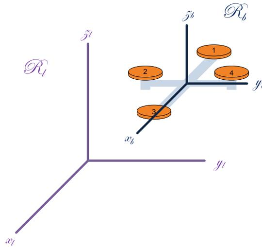
Figure 45. **Inertial and Body Frames of Reference**
