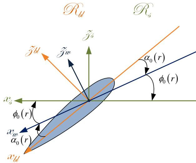
Figure 50. Wind frames of reference
