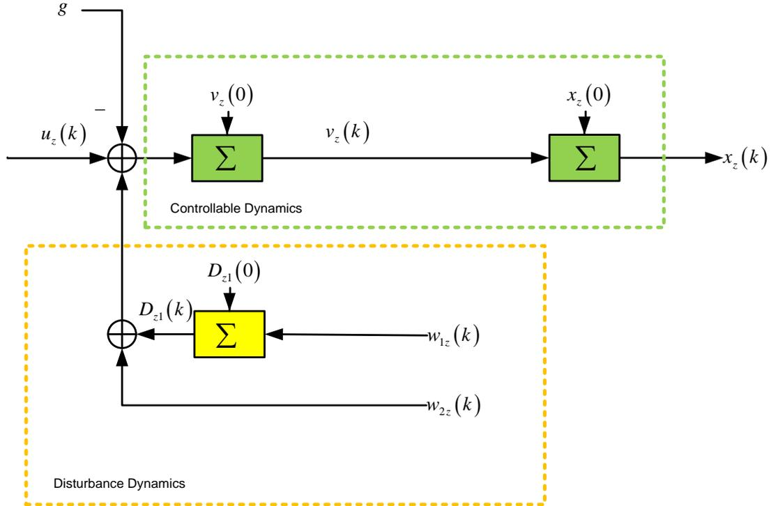
Figure 71. Diagram block of Vertical EM
