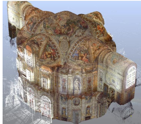
Figure 3 TLS point clouds adjusted in the same coordinate system
