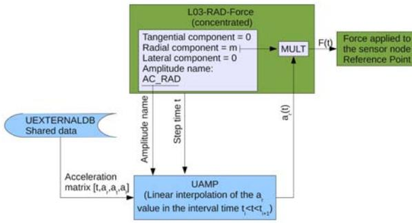
**Fig. 5** Computation of the concentrated radial force, acting on the sensor node, by the specification of the components and a user defined amplitude. The component is the sensor mass  $m$ , the amplitude returns the acceleration  $a_r(t)$  to which the material is subjected at the simulation time  $t$ .
