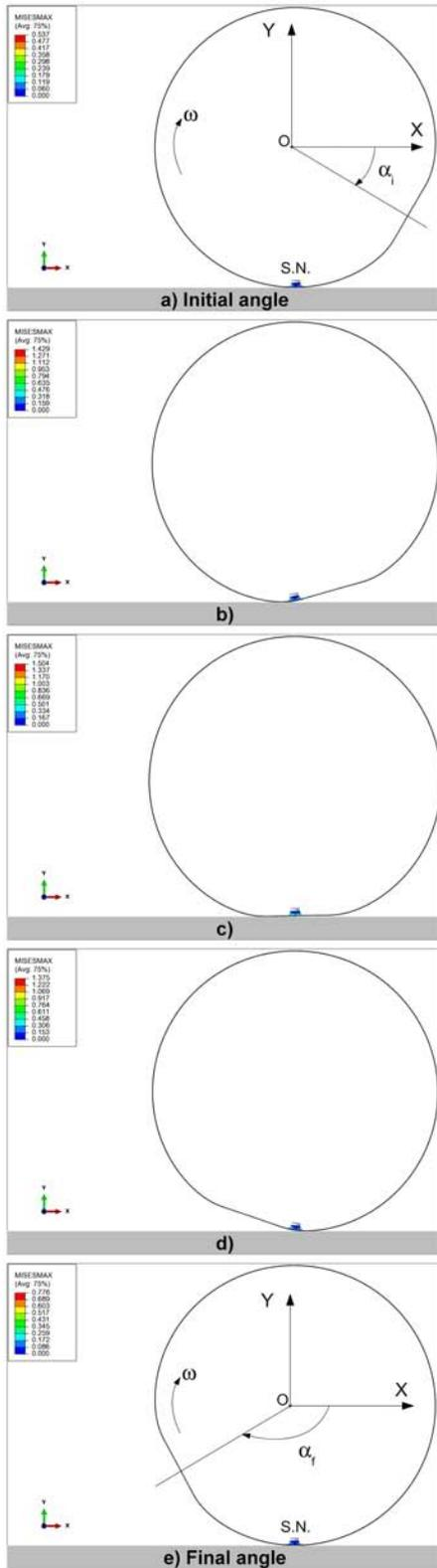
**Fig. 3** Deformed shape positions. a) The circular wheel has been deformed with the contact patch shape in the initial position  $\alpha_i$ . b, c, d) Other intermediate position of the deformed shape. e) Final simulation angle  $\alpha_f$ . The sensor node position does not change in the FEM reference system. The deformations are rotated under it.
