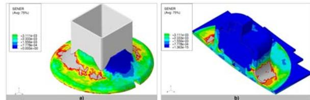
**Fig. 15** Simulation results of the final products and prototypes designed with the proposed methodology. a) Pirelli Cyber<sup>TM</sup> Tyre rubber house prototype [25]. b) Pirelli Cyber<sup>TM</sup> Fleet rubber house for TPMS [26].
