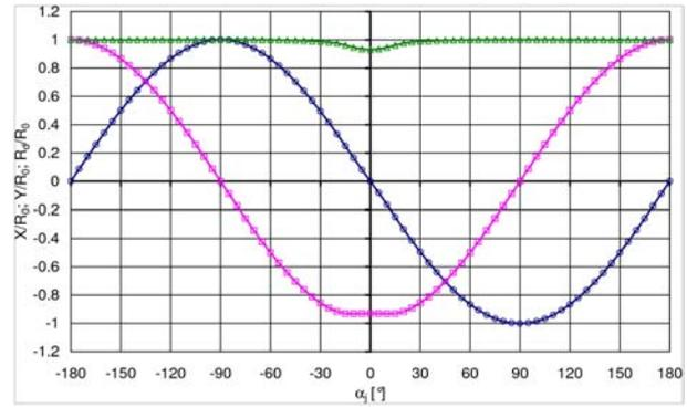
**Fig. 1** Deformed contour of the tyre. The coordinates of the measured points are expressed in Cartesian and Polar systems and made dimensionless by dividing by  $R_0$ , the undeformed tyre radius.  $\triangle R_d/R_0$ ;  $\circ X/R_0$ ;  $\square Y/R_0$ . The values are usually known at  $\alpha_j$  discrete angular positions. (Numerical results from a 3D FEM model, courtesy of Pirelli Tyre S.p.A.)
