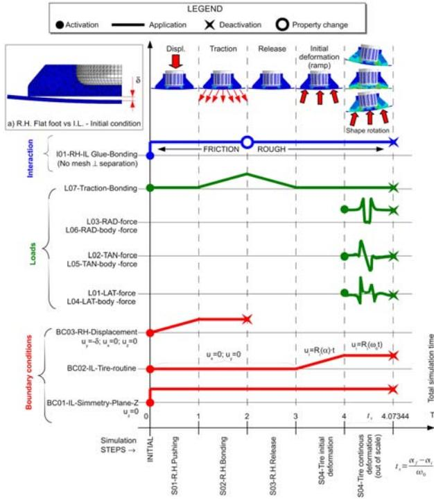
Fig. 9 Variation of the settings during the simulation.
