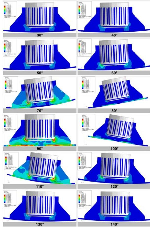
**Fig. 12** Elastic strain energy density results at different step frames. The scale for the SENER field output is set for all the images between 0 and  $0.075 \text{ J/cm}^3$ . The simulation frames have been saved with an increment in the angle  $\alpha$  of  $1^\circ$ , from  $\alpha_i = 30^\circ$  to  $\alpha_f = 150^\circ$ . Here are reproduced the frames with a step of  $10^\circ$ .
