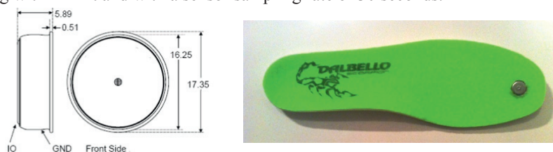
Fig. 1. Sensor shape and size [mm] and position of the sensors on the liner sole.
