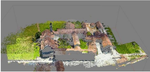
Figure 10. Calculated Tie Points in Photoscan
