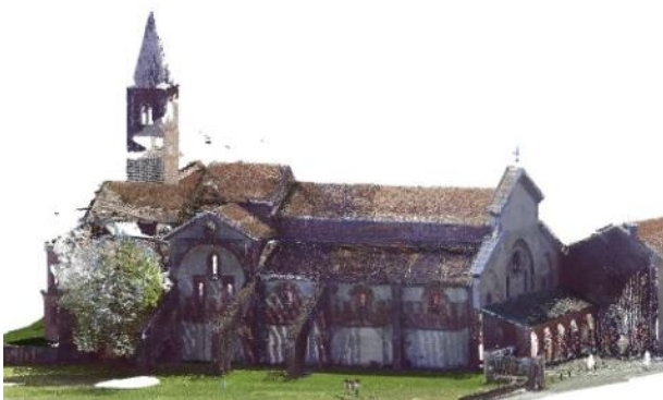
Figure 16. Point clouds data fusion
