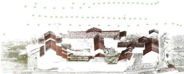
Figure 11. Visualization of calculated Tie Points with camera location in MicMac
