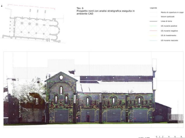
Figure 7.. Stratigraphic analysis of the north facade processed on image extracted from point cloud
