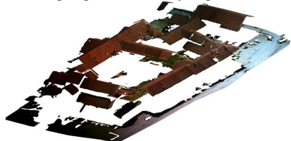
Figure 19. Point cloud extracted using MicMac software
