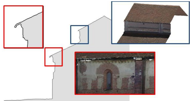
Figure 23. High details of ledges and adjacent areas on final textured model
