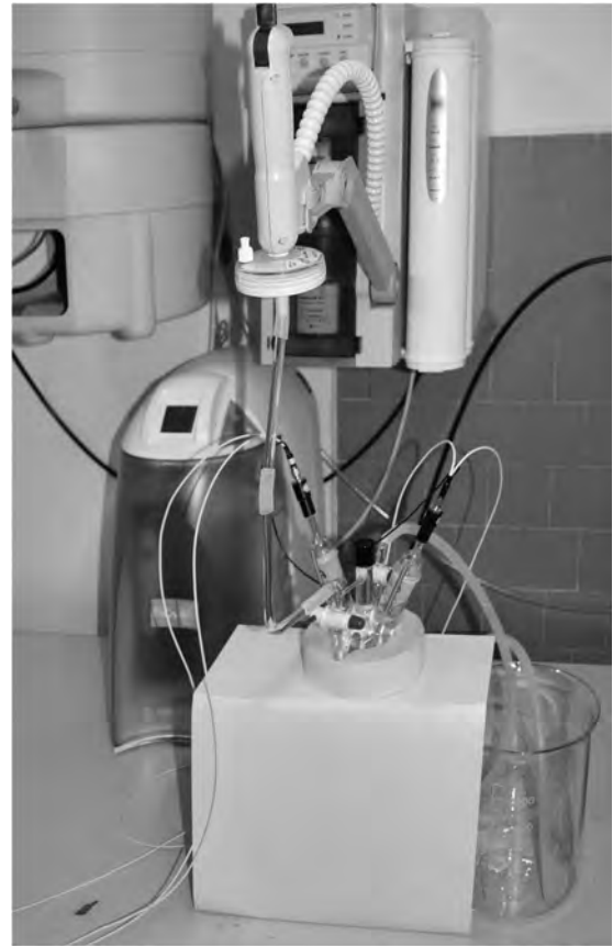
Fig. 3. In-flow setup for the measurement of ultrapure water. The production unit employed (Millipore mod. RiOs-Di and Milli-Q academic) is connected with Pyrex pipelines to the measurement cell in Fig. 2. Water outlet is collected in a beaker for temperature measurement.
