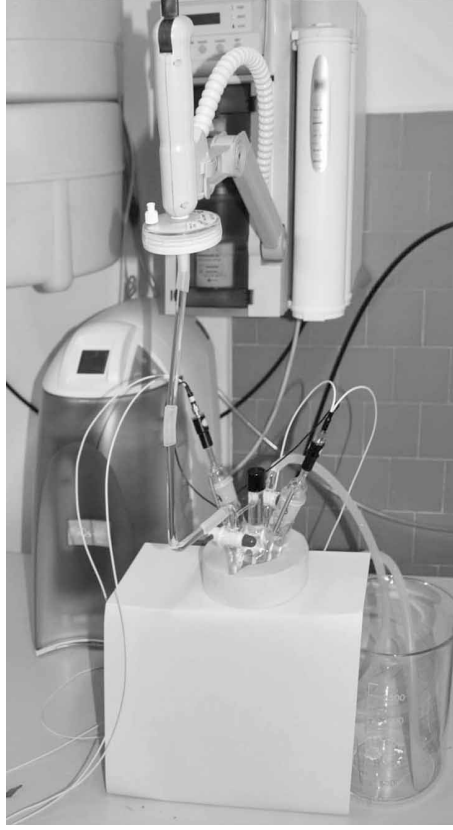
Figure 2.13: In-flow setup for the measurement of ultrapure water. The production unit employed (Millipore® mod. RiOs-Di and Milli-Q academic) is connected with Pyrex® pipelines to the measurement cell in Fig. 3.4. Water outlet is collected in a beaker for temperature measurement.
