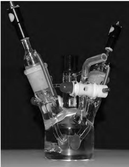
Fig. 2. Secondary cell employed for the measurements. The enclosure is in Pyrex glass, with a capacity of 150 ml; two circular parallel-plate Pt electrodes are supported by Pt wires that go through glass seals and permit electrical connection. The cell is provided with pipes for flowthrough measurements.
