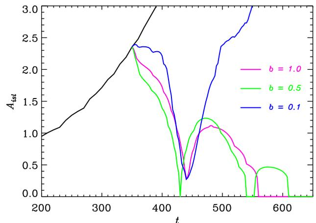
FIG. 2. Time evolution of the magnetic island area for three different values of the normalized current-drive width  $b = \delta/(\psi_X - \psi_O)|_{t_1}$ . The ECCD has been switched on at  $t_1 = 350$  with a maximum height of  $|J_m| = 10 \cdot (J_X - J_O)|_{t_1}$ .
