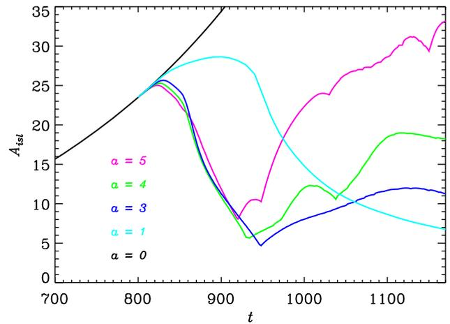
FIG. 4. Time evolution of the controlled magnetic island area for ECCD currents with different peak amplitudes  $J_m$  and a fixed beam width  $\delta = 0.5 \cdot (\psi_X - \psi_O)|_{t_1}$ . The control current injection starts at  $t_1 = 800$ .
