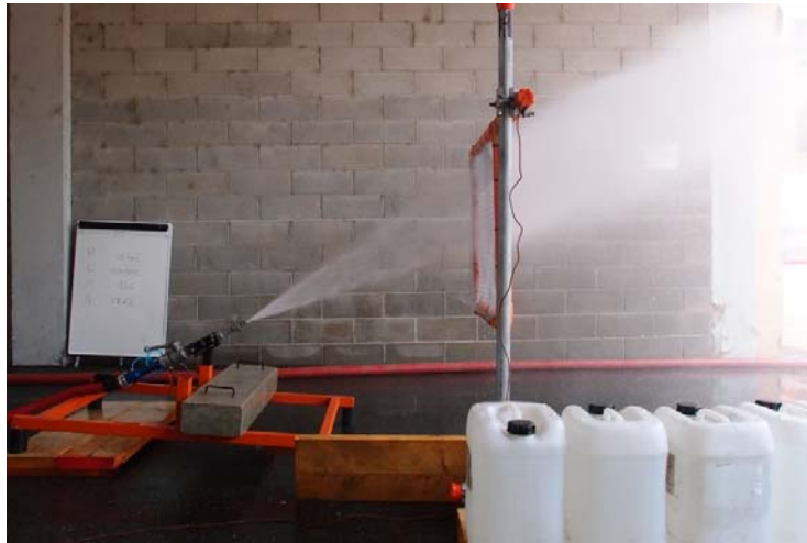
Figure 13. 'Branchpipe' hose – Spray stream
