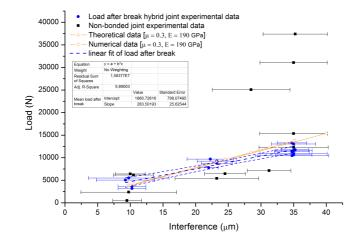
Figure 5.14: Comparison among the interference contribution detected from the load after break of hybrid joints, the unbonded interference samples, and the results of the analytical equations and the numerical analysis. The linear fits of the experimental points with the related 95% confidence bars are also depicted.
