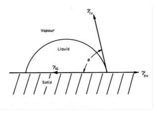
Figure 1.4: Equilibrium condition of a three-phase system: a liquid drop on a solid surface, exposed to a saturated vapor of the liquid [8].
