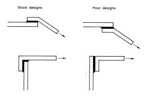
Figure 1.10: Schematic diagram of some good and poor joint design [8].
