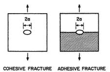
Figure 1.7: Comparison between cohesive and adhesive fracture [21].
