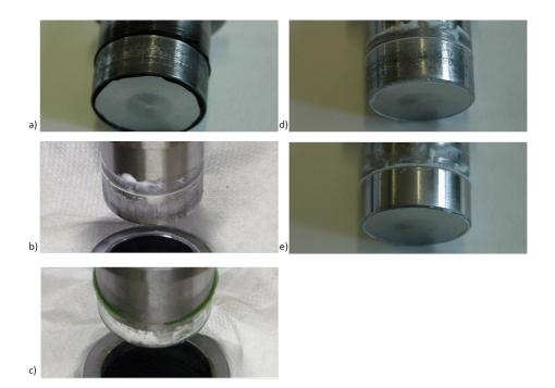
Figure 4.7: Fracture shaft surfaces of the decoupled joints: a) typical black layer of the cured FT-EP adhesive; b) typical white layer of the cured AC adhesive; c) typical grey residues of the cured PU adhesive; d) grey residues of the cured R-EP adhesive; e) R-EP sample where cured particles are not present on the mating surface.
