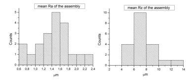
Figure 4.11: statistical distribution of the mean  $R_a$  and  $R_z$  calculated for every hub-shaft assembly [76].
