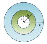
Figure 2.4: Schematic representation of the Lamè's theory system based on two thick walled cylinders.
