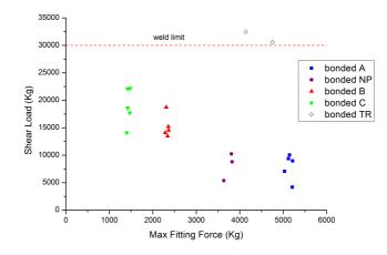
Figure 6.13: Shear test results of bonded wheels joined with different interference systems.
