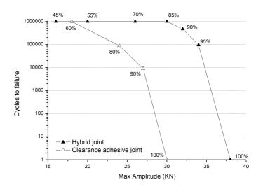
Figure 5.18: Comparison between the attained cycles to failure of hybrid joints and clearance adhesive joints at difference maximum stress amplitudes. The  $F_{max}$  in percentage of the total static resistance is indicated for both case.
