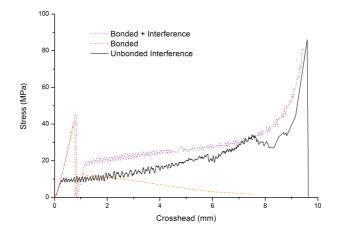
Figure 4.9: Average stress/displacement curves of the hybrid, bonded with clearance and the unbonded interference samples for the FT-EP adhesive [76].
