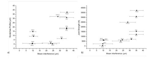
Figure 5.10: Relation between the  $spR_a$  and the interference level (a) and its consequence on the measured decoupling loads (b)
