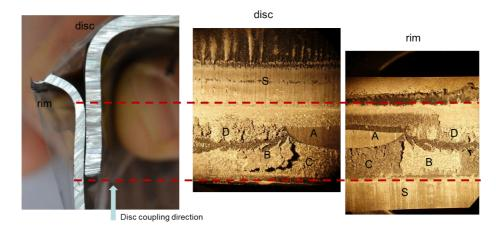
Figure 6.6: Mating fracture surfaces of disc and rim. The areas A, B, C, D and S are identified in both the rim and the disc surfaces. A section of the joint is depicted and the limits of the joint area are marked.
