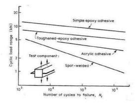
Figure 1.12: Fatigue properties of steel double-box hat structures either adhesively bonded or spot welded [44].
