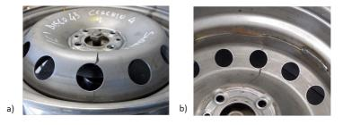
Figure 6.18: Failure mode common to all the samples tested to fatigue rolling. The crack, started by a disc window, reaches the joint area inducing the wheel decoupling
