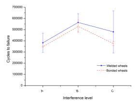
Figure 6.17: Results of the rolling tests of A, B and C wheels with the radial and lateral loads augmented of 15%
