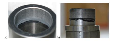
Figure 5.11: a) Hub and b) shaft of a hybrid joint at 35  $\mu m$  of interference after the decoupling phase [75]
