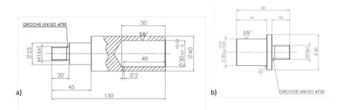
Figure 3.3: Dimensions in mm and tolerances of the specimens: a) hollow tube, b) shaft [75]
