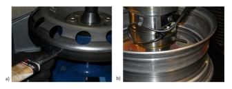
Figure 6.1: Two pictures of the assembly process of the wheel protopes: (a) the spreading of the adhesive on the disc flange; (b) the press-fit of the components
