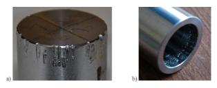
Figure 5.5: Scratches present after the decoupling on both the mating surfaces of: a) shaft and b) hub [75].
