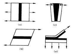
Figure 1.9: Types of stress: (a) normal (or direct) stress, (b) shear stress, (c) cleavage stress, (d) peel stress [8].
