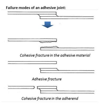
Figure 1.2: Schematic representation of the different failure modes of an adhesive joint. [22]
