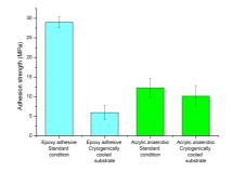
Figure 2.5: Shear strength of epoxy and anaerobic acrylic adhesive lap shear joints, bonded in standard condition and bonded with a frozen substrate.
