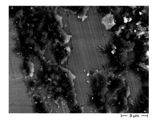
Figure 5.12: SEM magnification of the fracture surface of a shaft from a hybrid joint at 35  $\mu m$  of interference after the decoupling phase
