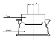
Figure 6.2: Schematic representation of the peel test on wheel [3].
