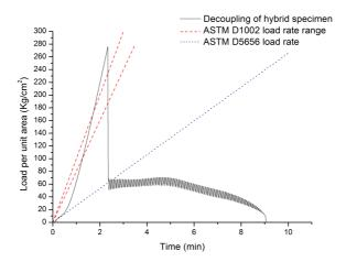
Figure 3.6: Load rate of decoupling test on hybrid joint at a crosshead speed of 1,3 mm/min, compared with the standard decoupling rate for the single lap shear and the thick adherend lap shear test
