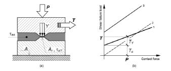
Figure 2.7: (a) Micromechanical model of the hybrid interface and (b) typical predictions for its macroscopic shear strength (curve 1 is related to the weaker anaerobic adhesive hybrid condition, curve 2 to the unbonded condition, curve 3 to the stronger anaerobic adhesive hybrid condition) [53].
