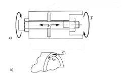
Figure 3.2: Schematic representation of the analogous test used for controlling the clamping force in clamped-bonded interfaces in Sawa et al. experiments [17]: a) testing scheme b) loads on the circumferential bonded area
