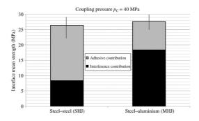
Figure 2.8: Comparison of total interface mean strength between steel-steel and steel-aluminum hybrid joint: interference contribution  $(P\mu)$  and adhesive contribution  $(\tau_a)$  are highlighted [15,55].
