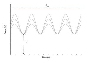
Figure 3.7: Schematic example of the load cycles employed in fatigue tests
