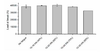
Figure 5.19: Strength decay of hybrid joint after  $10^6$  fatigue cycles at different force amplitude in respect to their static pull-out strength. The  $F_{max}$  in percentage of the total static resistance is also indicated.
