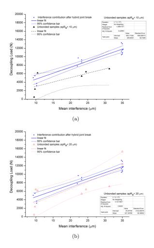
Figure 5.15: Comparison between the linear fits of the load after break points, and results of the unbonded joints characterized by values of (a):  $spR_a < 20$   $\mu$ m, and (b):  $spR_a < 10 \ \mu$ m
