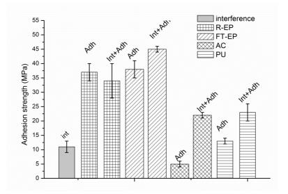
Figure 4.13: Comparison between the adhesion strength values of all the studied adhesive systems. The interference system is labeled as "Int", the bonded with clearance systems as "Adh", the hybrid systems as "Int+Adh" [76].
