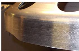
Figure 6.12: Roughness on the disk flange of the TR case, due to the turning operation .
