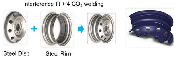
Figure 1: Schematic representation of the present joining technology of the wheel system.
