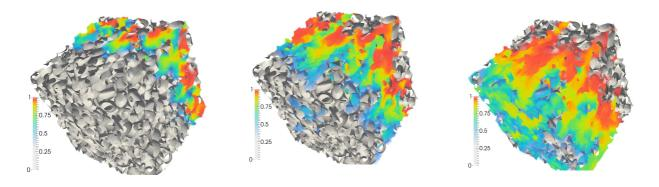
Results are then analyzed in terms of velocity distributions and dispersion rates in a wider range of operating conditions, when compared with other works carried out by solving the Stokes equation. Results show that dispersion within the analyzed porous medium is adequately described by classical power laws obtained by analytic homogenization. Eventually the validity of Fickian diffusion to treat dispersion in porous media is also assessed.
