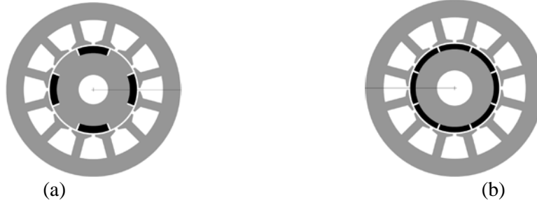
Fig. 5.2: Machines with same rotors as those of Fig. 5.1 and concentrated stator windings
