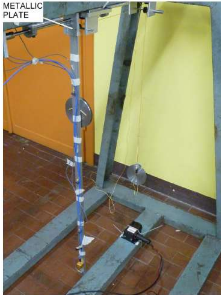
Fig. 2. Complete structure. At the top, the plate added to the system to enforce the clamp is highlighted. The travelling mass and the counterweight are observable on the left and on the right, respectively.
