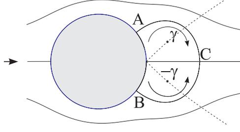
**Figure 2.** Symmetric Föppl solution,  $\gamma_0 = 0$ ;  $\gamma = \gamma_1 = -\gamma_2 = -4.2$ ;
