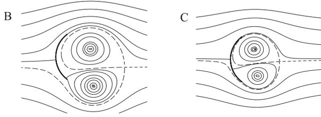
**Figure 5.** Flows past a circular arc ( $\alpha = 0$ ,  $b = -0.5$ ). **A:**  $\gamma_0 = 0$ ;  $\gamma_1 = -7.01$ ;  $\gamma_2 = 7.01$ . **B:**  $\gamma_0 = 0$ ;  $\gamma_1 = -10.87$ ;  $\gamma_2 = 9.85$ . **C:**  $\gamma_0 = 0.395$ ;  $\gamma_1 = -7.83$ ;  $\gamma_2 = 7.08$ .
