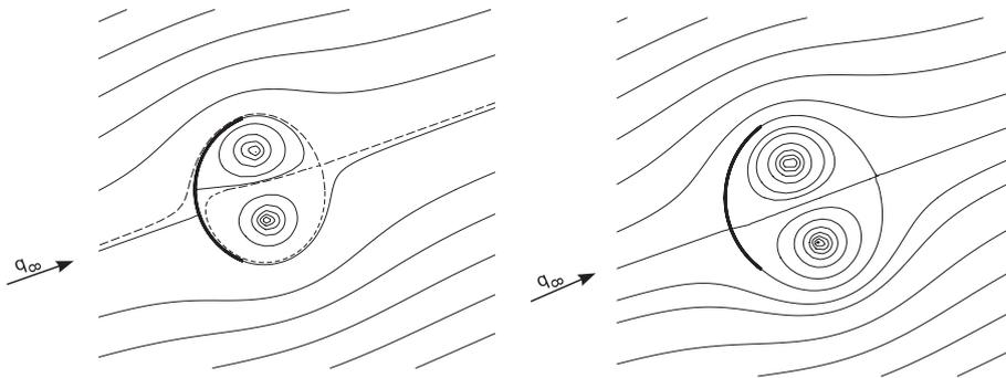
**Figure 7.** Circular arc at incidence ( $\alpha = 20^\circ$ ). Left:  $\gamma_0 = 0$ ,  $\Delta\psi_{st} \neq 0$ ; right:  $\gamma_0 = 0.18$ ,  $\Delta\psi_{st} = 0$
