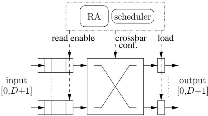
Fig. 4. Architecture of a node for intra-IP NoCs
