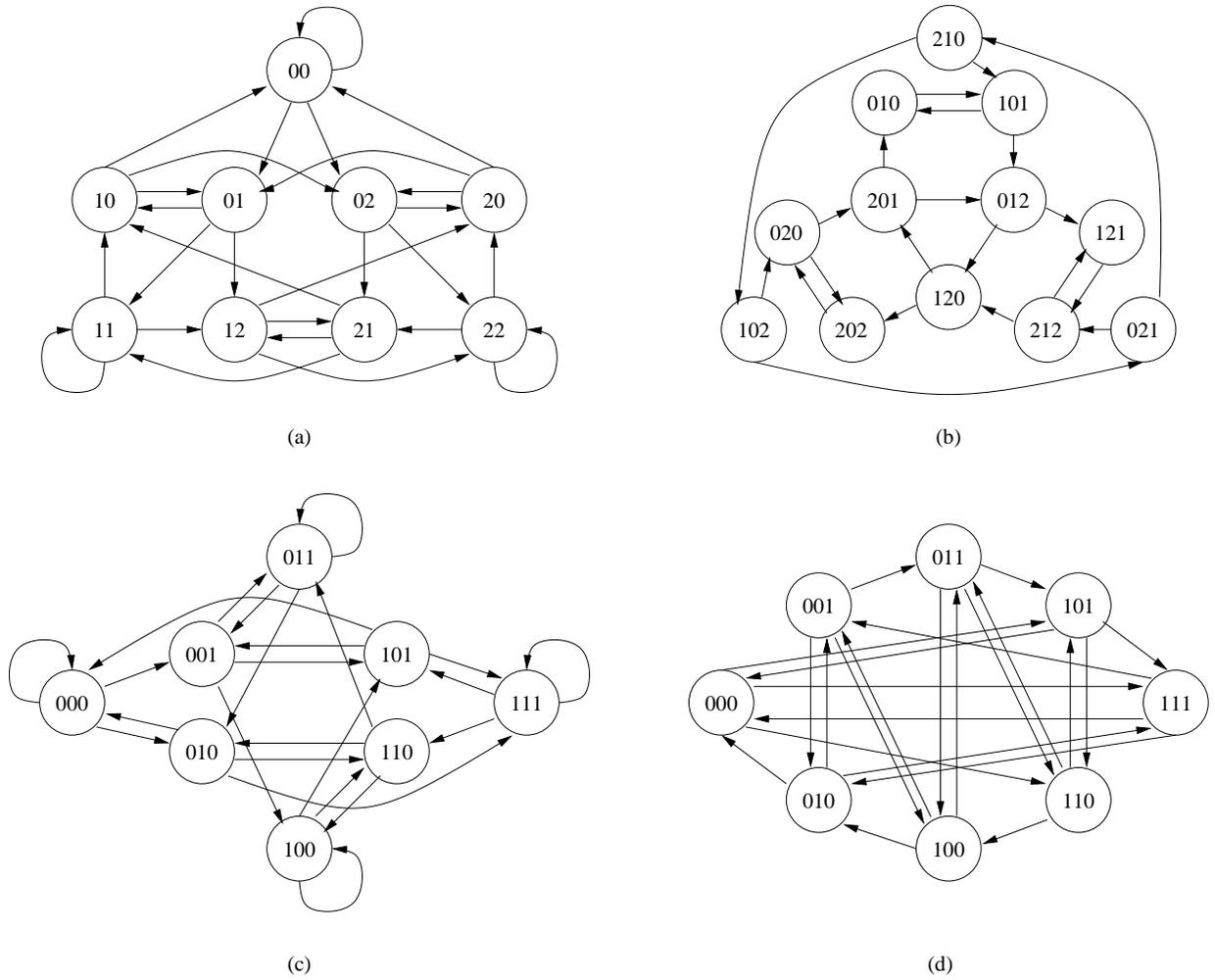
Fig. 1. Example of logarithmic diameter graphs: (a)  $q = 2, l = 3$  ( $D = 3, P = 9$ ) de-Bruijn graph, (b)  $q = 3, l = 3$  ( $D = 2, P = 12$ ) Kautz graph, (c)  $D = 3, P = 8$  generalized de-Bruijn graph, (d)  $D = 3, P = 8$  generalized Kautz graph.
