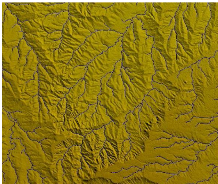
Figure 22: The figure shows the hydrographic grid obtained using GIS software for the NED in a sample area (ESRI ArcGIS Desktop) The evaluation has been performed by means of the procedure described below:
