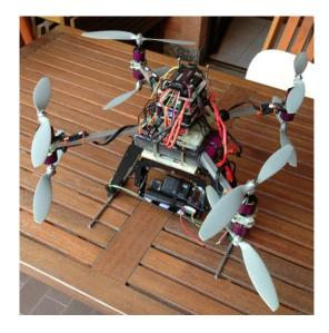
Figure 1.21: Qx-Rotor: the realized prototype
