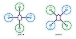
Figure 1.14: Quadrotor + and X flight configurations
