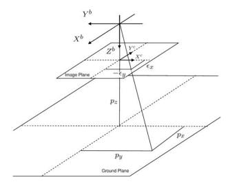
Figure 6.1: Camera model for the multirotor
