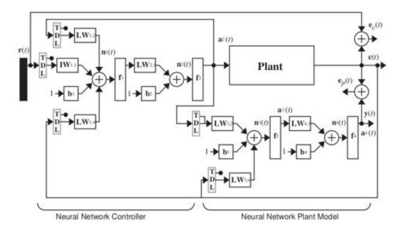
Figure 10.17: Detailed model reference control structure
