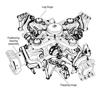
Figure 1.1: Full-scale helicopter swashplate [1]
