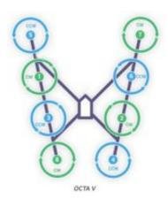
Figure 1.17: Octorotor V design configuration
