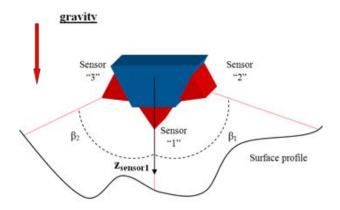
Figure 10.25: A three sensors setup
