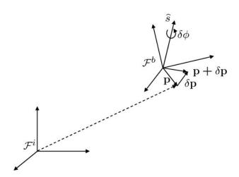
Figure 2.9: Derivation of the equation of Coriolis
