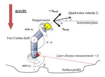
Figure 10.22: Distance sensor embodiment
