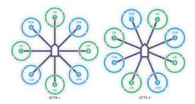
Figure 1.16: Octorotor + and X flight configurations
