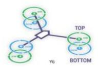
Figure 1.18: Hexarotor Y design configuration
