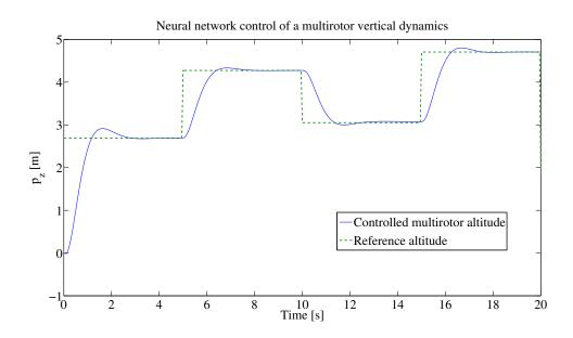
Figure 10.20: Neural network controlled vertical position
