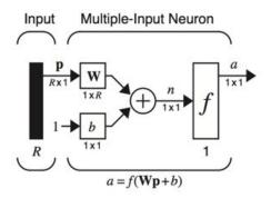
Figure 10.5: Neuron with R inputs, matrix notation
