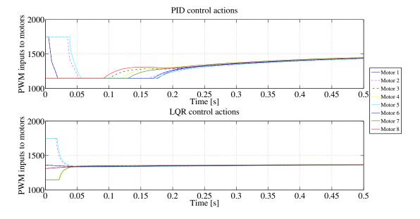
Figure 9.4: Control actions: PID vs. LQR
