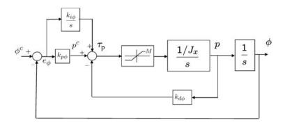
Figure 8.2: A block diagram of the roll attitude hold loop
