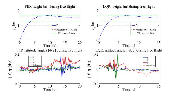
$\textbf{Figure 9.10:} \ \, \textbf{PID} \ \, \textbf{and} \ \, \textbf{LQR} \ \, \textbf{controlled height and attitude angles during free flight} \\$
