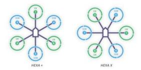
Figure 1.15: Hexarotor + and X flight configurations
