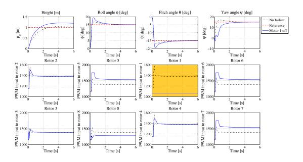
Figure 9.5: PID control simulation in case of motor "1" failure
