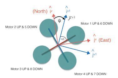
Figure 2.6: The vehicle-1 frame. If the roll and pitch angles are zero, then the x-axis points out the nose of the airframe, the y-axis points out to the right and the z-axis points into the earth
