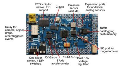
Figure 4.2: The OilPan Inertial Measurement Unit
