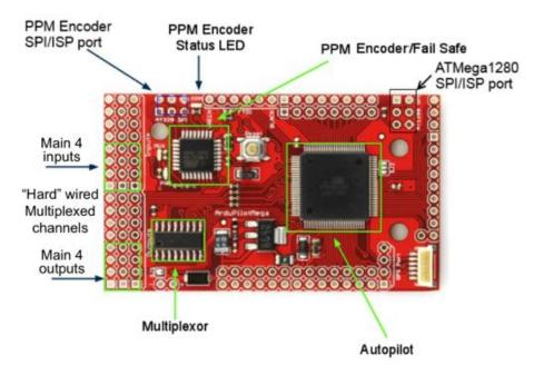
Figure 4.1: The Ardupilot Mega board
