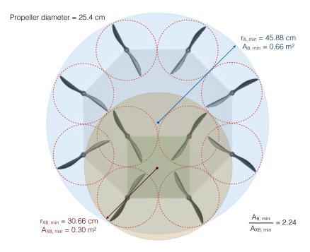
Figure 4.6: Comparison between the classical and X8 octorotor minimum size
