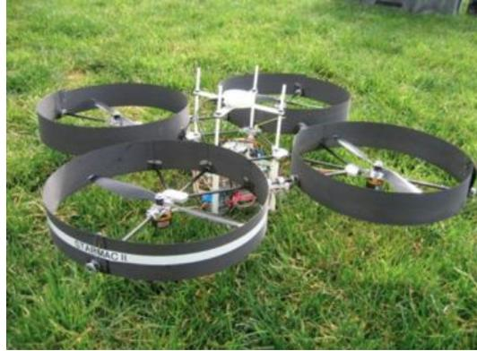
**Figure 1.12:** Stanford STARMAC Quadrotor
