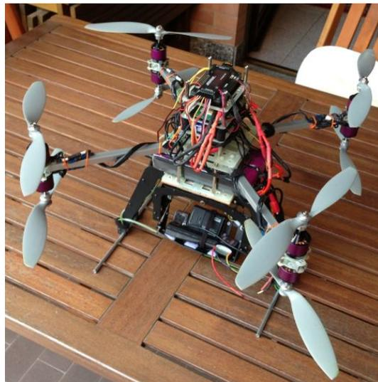
**Figure 1.21:** *Qx-Rotor*: the realized prototype
