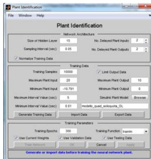
**Figure 10.18:** Matlab graphical user interface for plant identification and training
