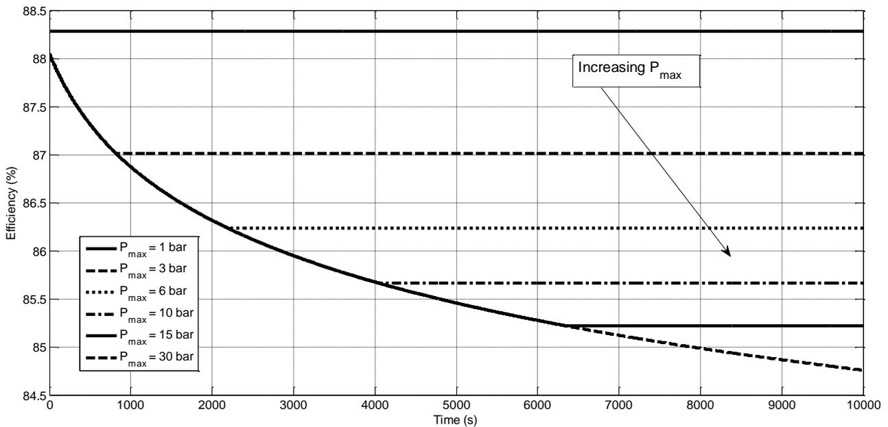
**Figure 4.59** Efficiency. Current = 375 A. Increasing maximum pressure. T = 70°C (343 K). Initial pressure set at 1 bar
