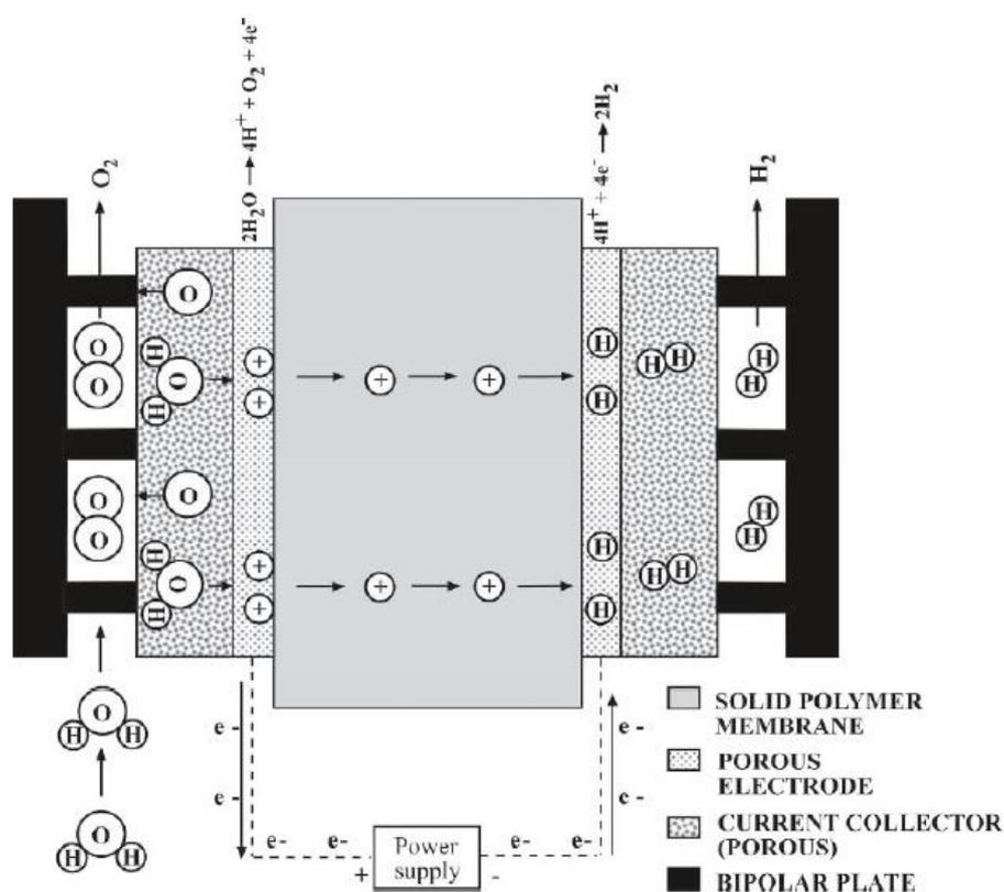
**Figure 1.17** A solid polymer electrolyser cell configuration
