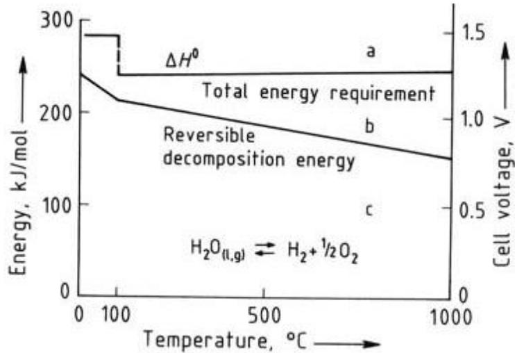
**Figure 1.18** Energy requirement for electrolysis as function of temperature (Häussinger et al., 2012)
