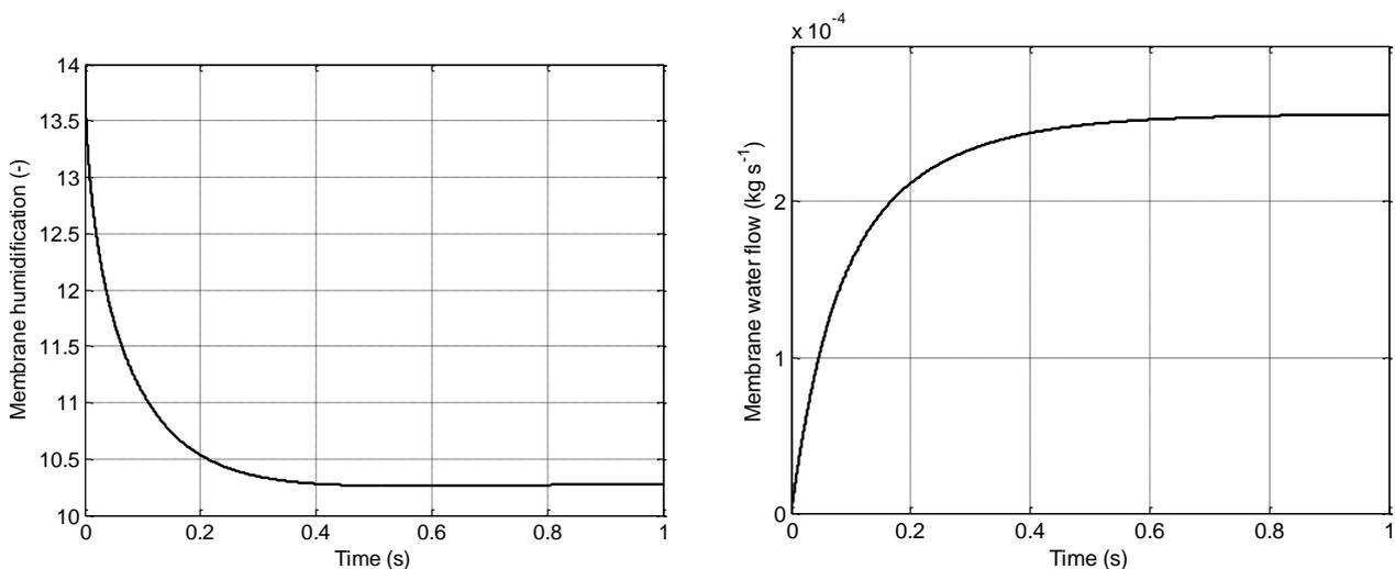
**Figure 3.46** Humidifier membrane humidification and water flow
