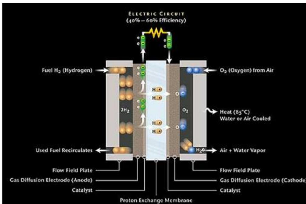
**Figure 1.3** A typical PEM fuel cell operation
