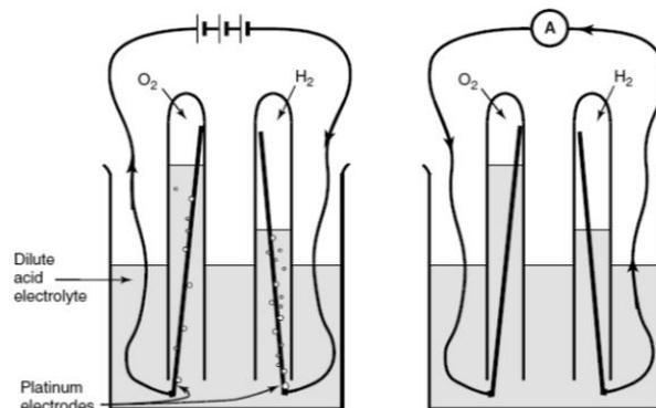
**Figure 1.1** (a) water electrolysis process; (b) fuel cell basic function principle
