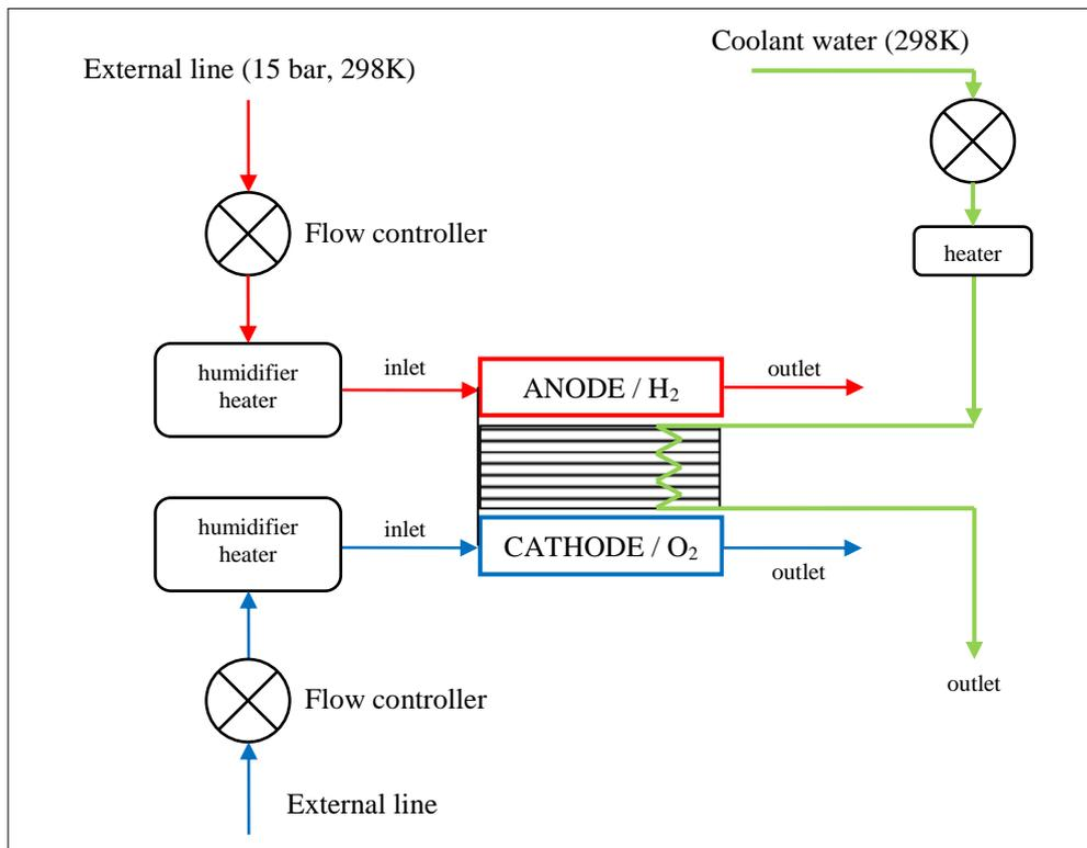
**Figure 4.1** Ballard fuel cell stack test rig layout
