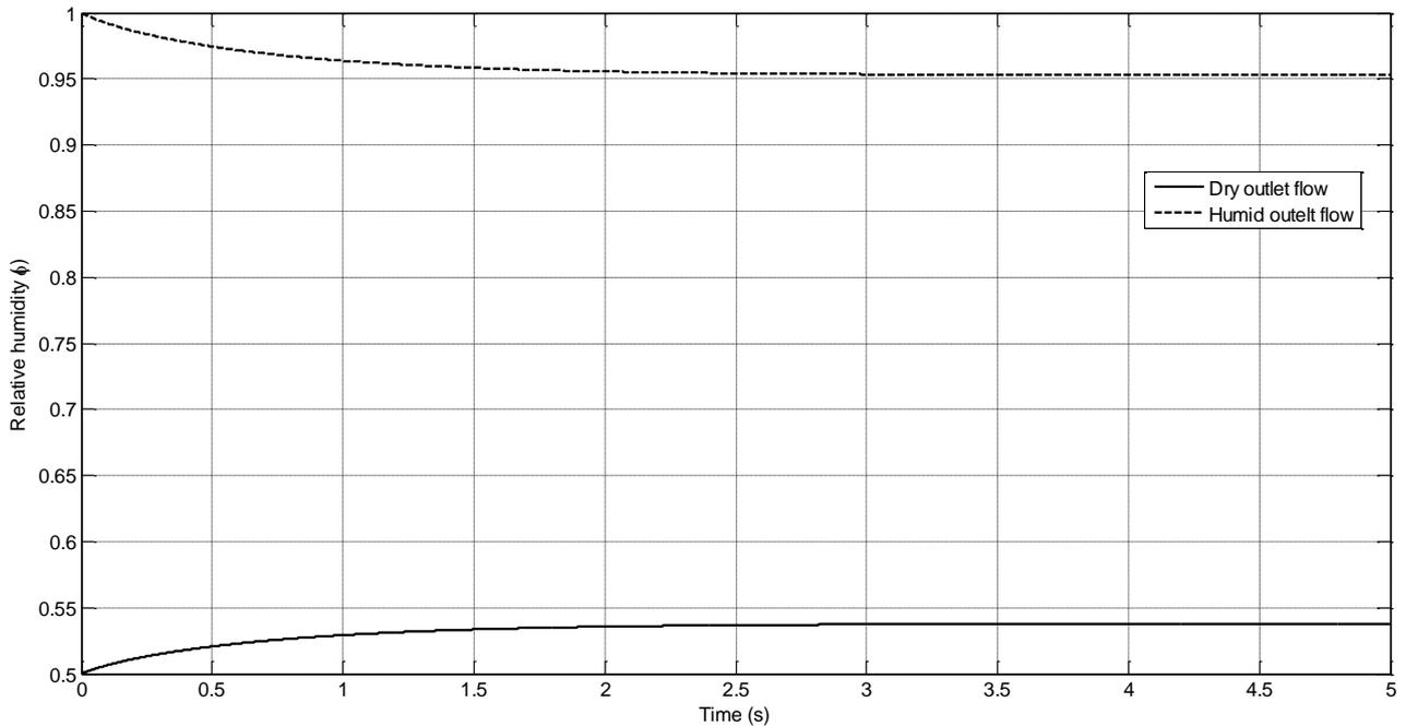
**Figure 3.42** Cathode humidifier outlet flow relative humidity
