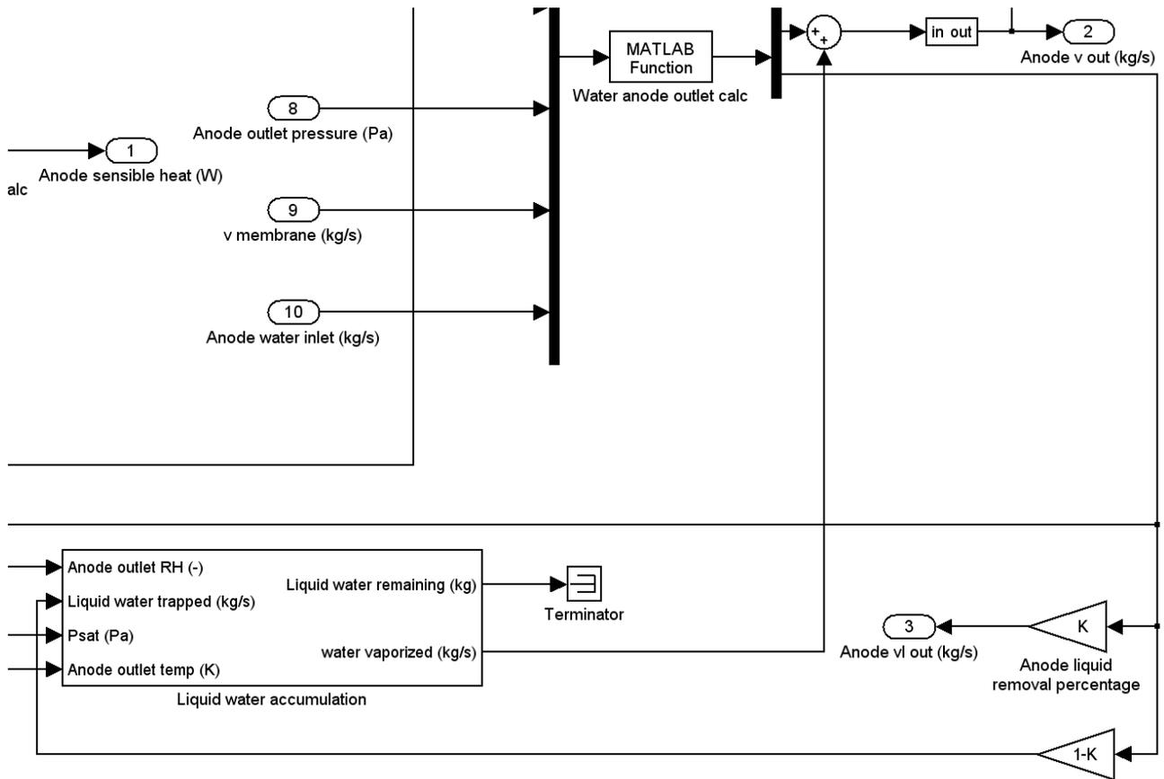
Figure 3.11 Liquid water accumulation and removal portion
