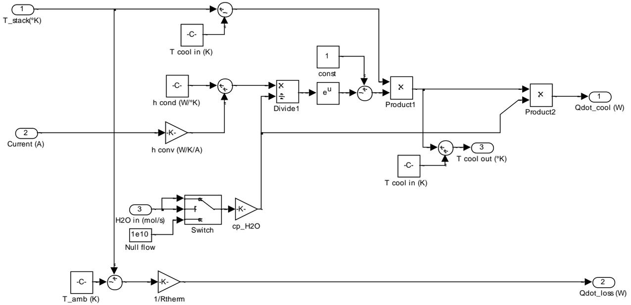
**Figure 2.4** Thermal cooling model block in Simulink
