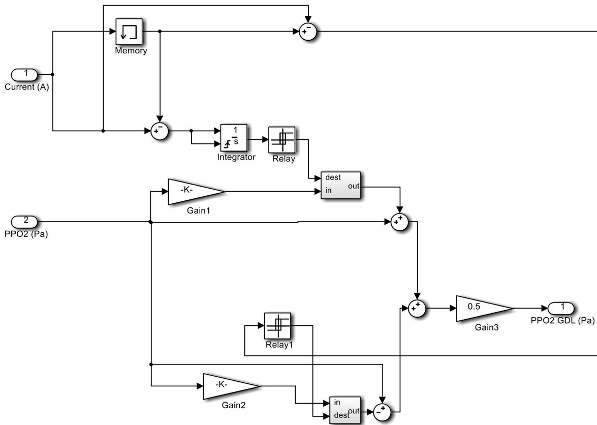
Figure 4.17 GDL model block in Simulink
