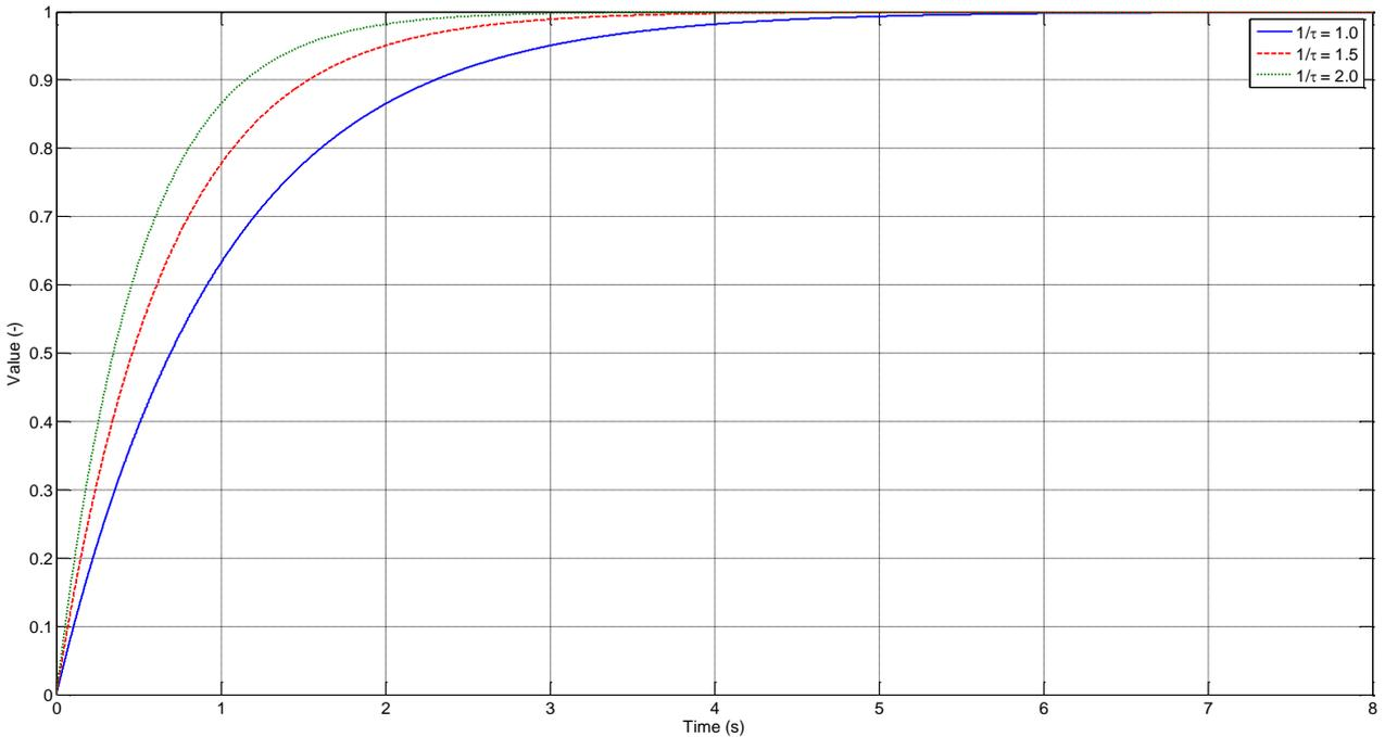
**Figure 3.12** Delay block behavior
