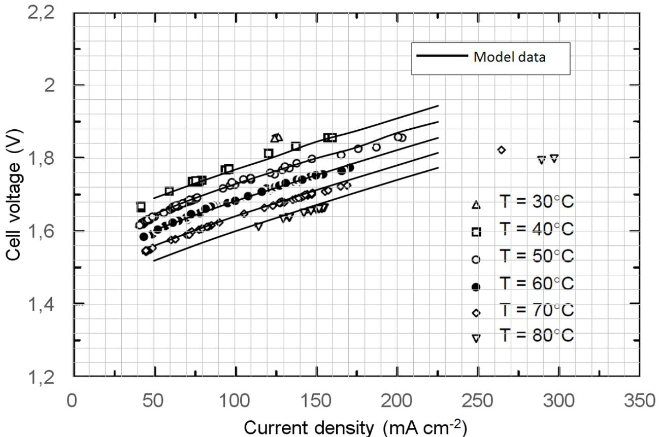
**Figure 4.54** Electrolyser model calibration and validation results
