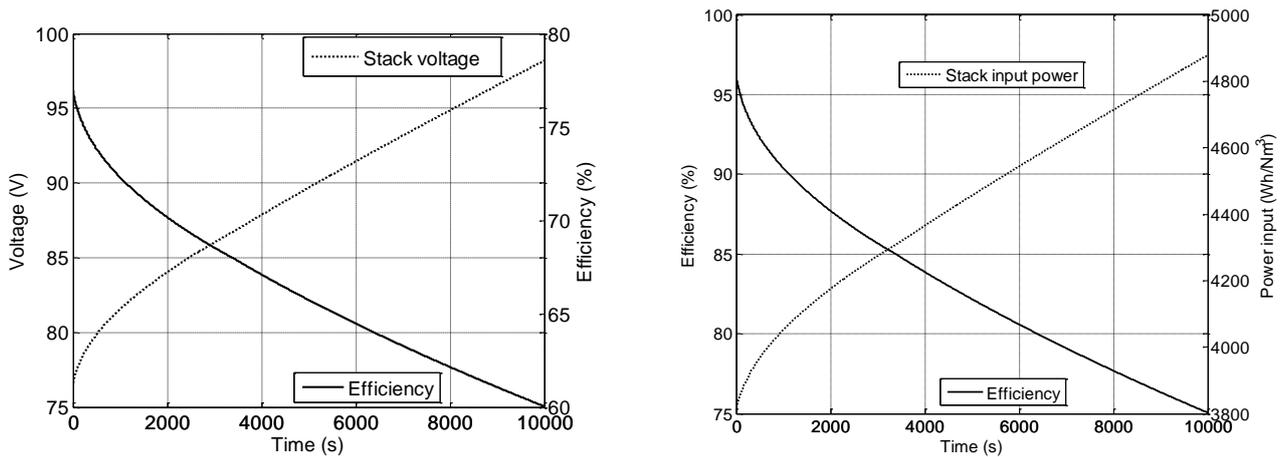
**Figure 4.61** Voltage and efficiency (left). Power input and efficiency (right). Ramp response. Pressure fixed at 1 bar.  $T_{\text{stack}} = 70^\circ\text{C}$  (353 K)
