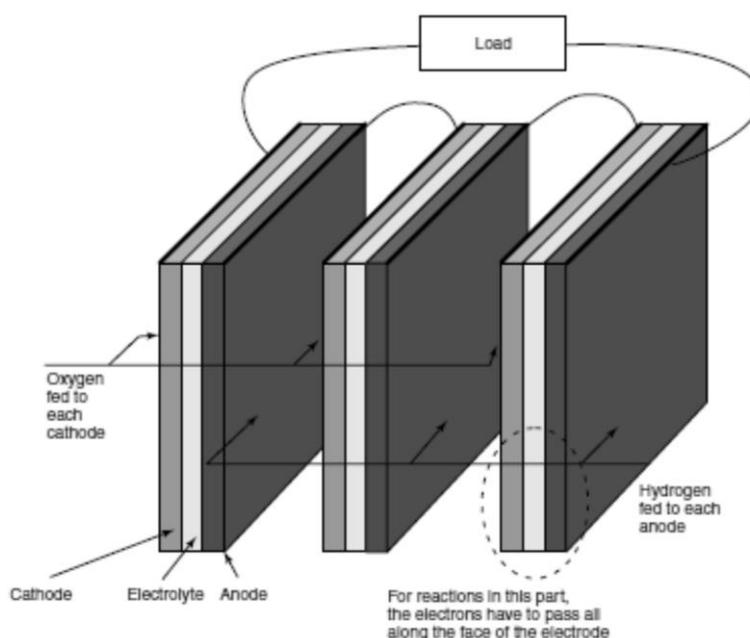
**Figure 1.7** Edge connection of cells in series
