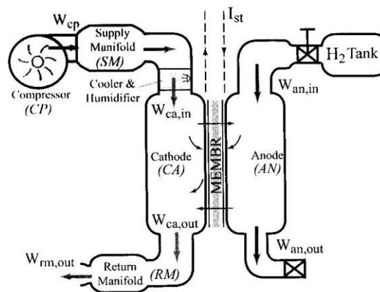
**Figure 3.4** System layout modeled in Pukrushpan et al. (2004)
