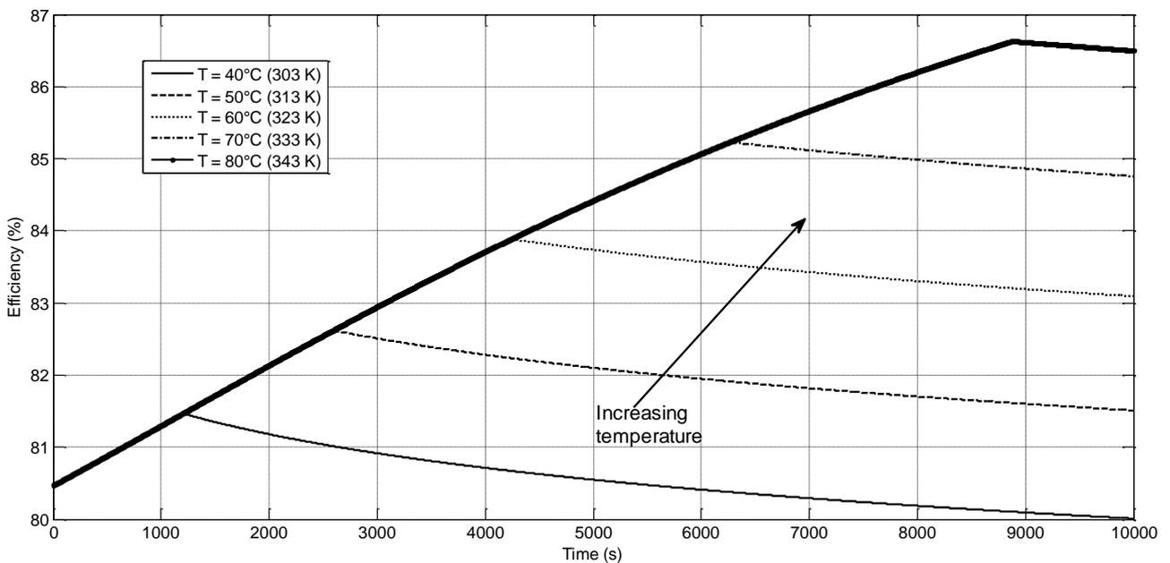
**Figure 4.58** Efficiency. Current = 375 A. Increasing temperature. P = 30 bar. Initial temperature set at 35°C (308 K)
