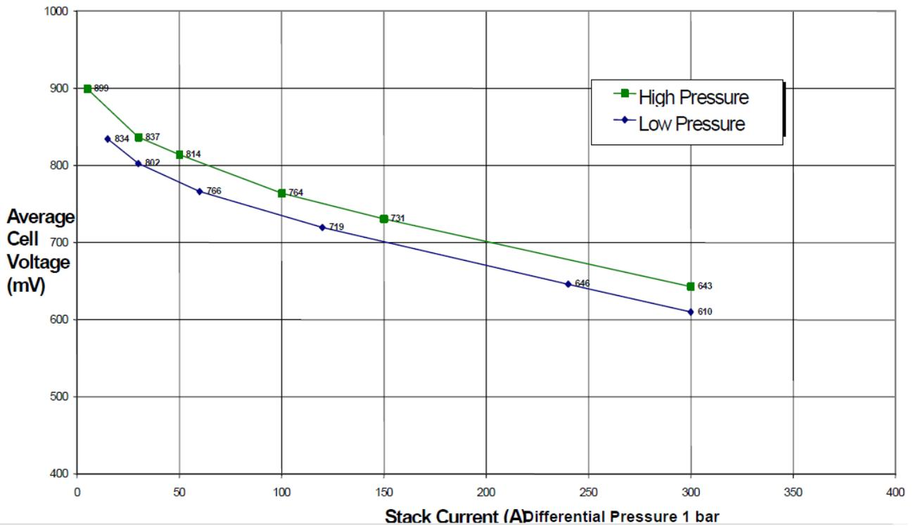
Figure 4.3 Ballard Mark 9<sup>TM</sup> SSL polarization curve
