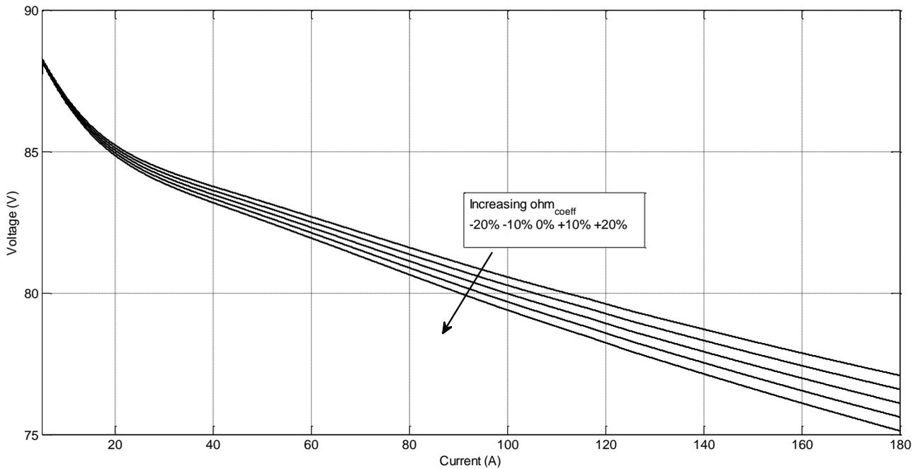
**Figure 4.46** Stack voltage vs. current.  $Ohm_{coeff}$  variations. -20%; -10%; 0%; +10%; +20%
