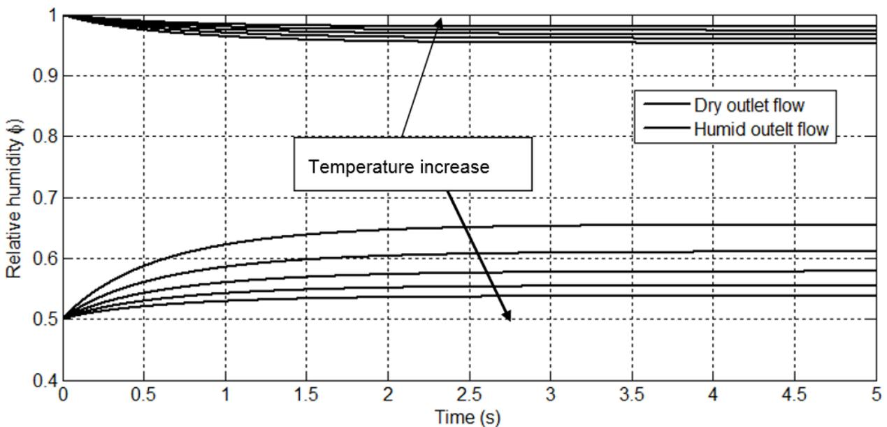
**Figure 3.43** Variation in outlet relative humidity with temperature. Null heat exchange. Uniform flows.
