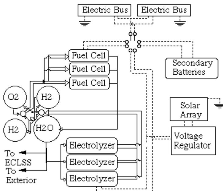
**Figure 1.5** Hypothetical electric power system based on RFCs
