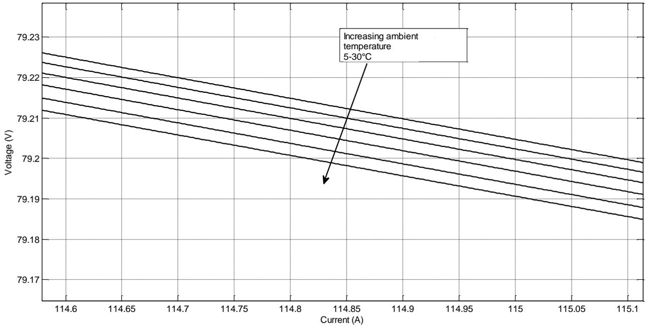
**Figure 4.44** Stack voltage vs. current. Ambient temperature variation. 5-30°C (278-303K). Zoomed area
