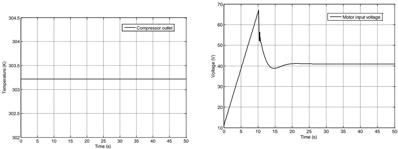
**Figure 3.27** Compressor outlet temperature (left side) and motor input voltage (right). Minimum pressure and flow
