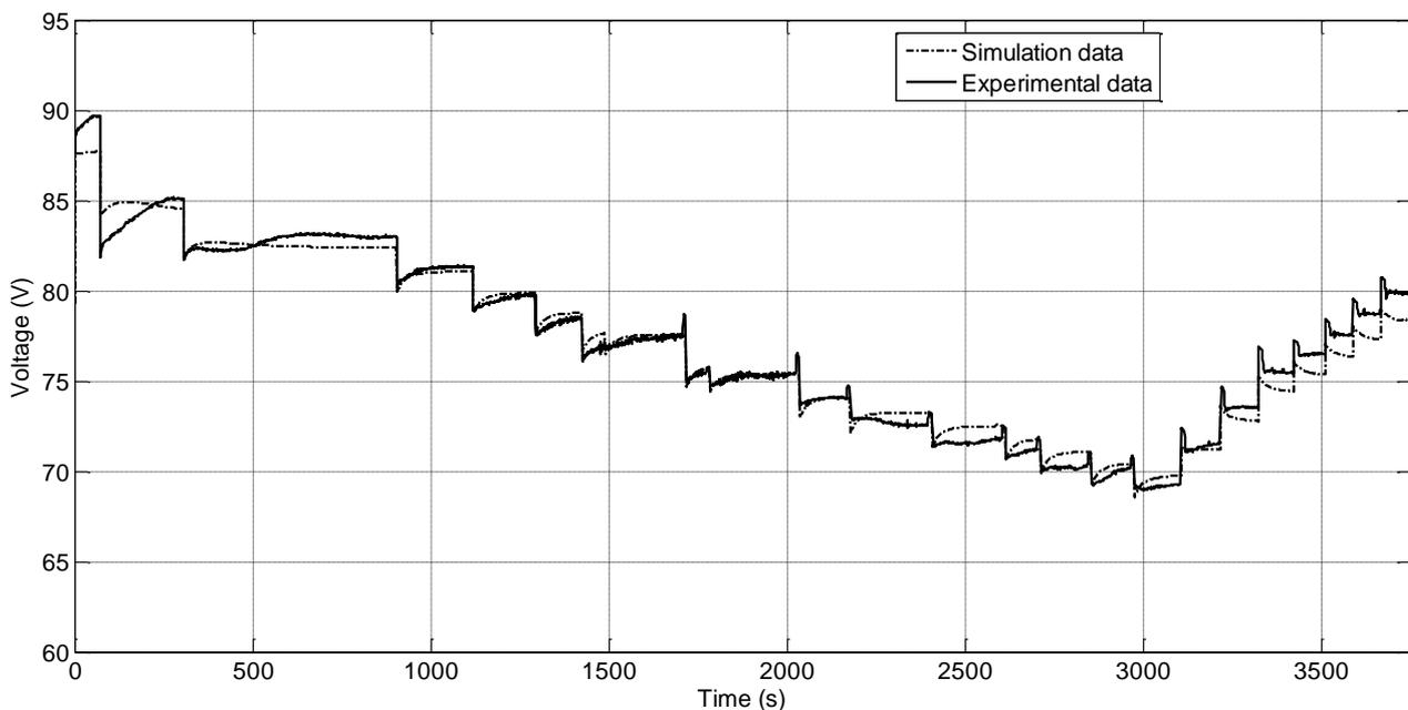
**Figure 4.19** Comparison between experimental and simulation voltage data using degraded membrane and new GDL formulation
