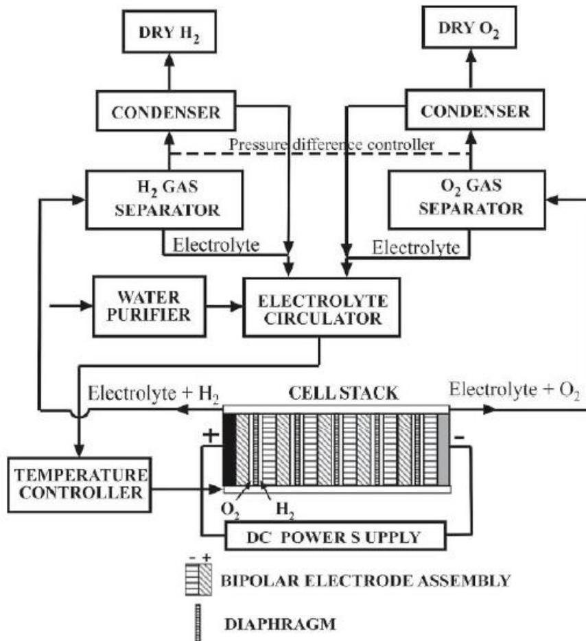
Figure 2.1 Typical alkaline or PEM electrolyser system layout
