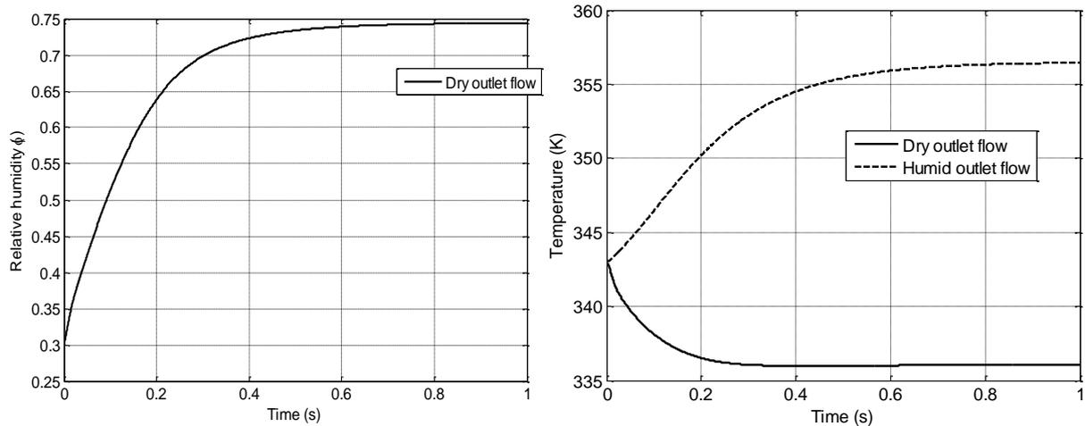
**Figure 3.45** Humidifier outlet humidity and temperature values using constant humid side relative humidity
