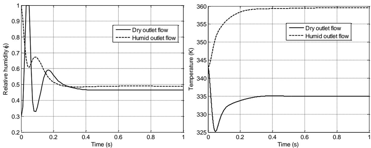
**Figure 3.44** Humidifier outlet humidity and temperature values
