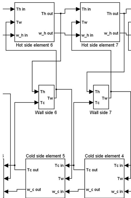
Figure 3.30 Detail of the intercooler Simulink model
