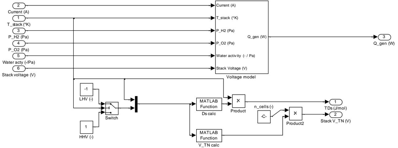
**Figure 2.3** Stack voltage / efficiency model block in Simulink
