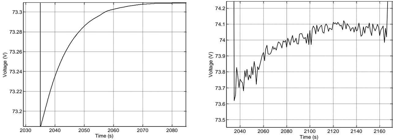
**Figure 4.14** Simulation (left) and experimental (right) transient response. Zoom of the voltage vs. current curves
