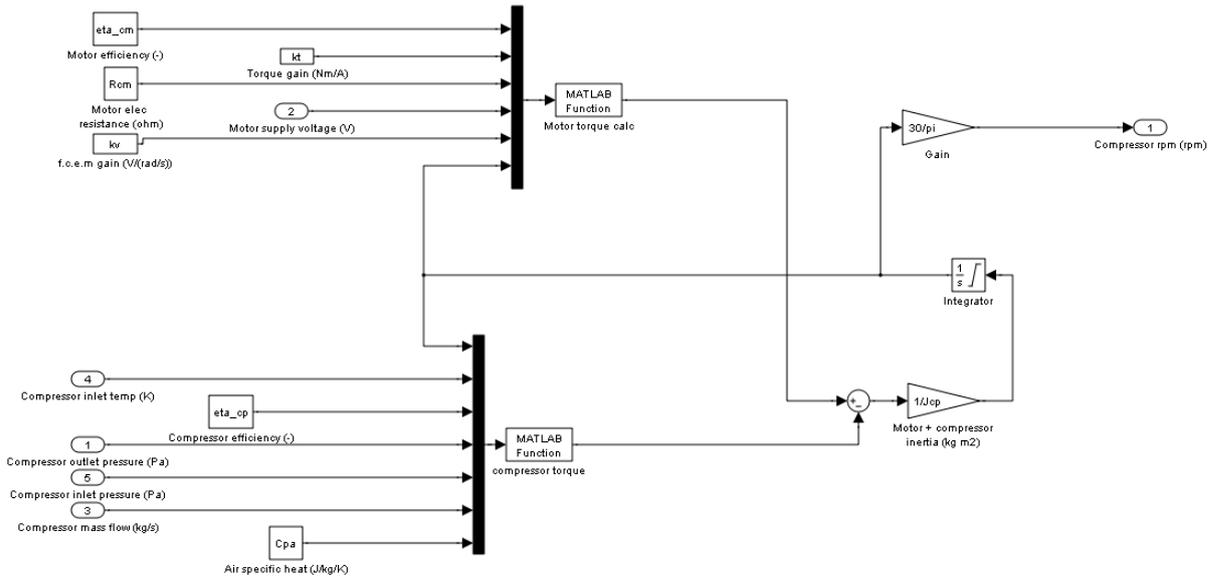
Figure 3.22 Compressor electric motor block
