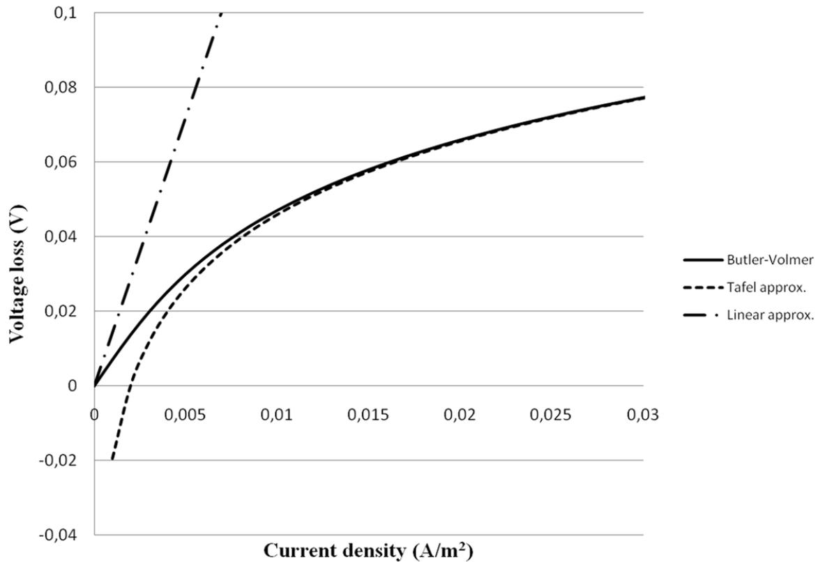
**Figure 2.6** Butler-Volmer equation and approximation comparisons for the cathode side
