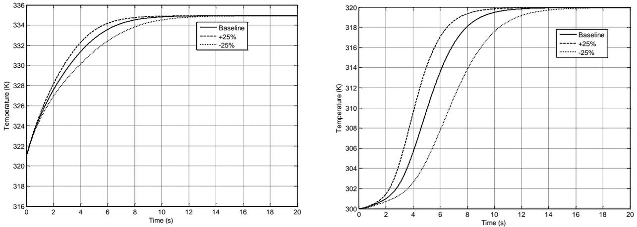
**Figure 3.36** Outlet temperature variation obtained varying the  $K_{1C_{ic}}$  and  $K_{2C_{ic}}$  variables. Air side (left). Water side (right)
