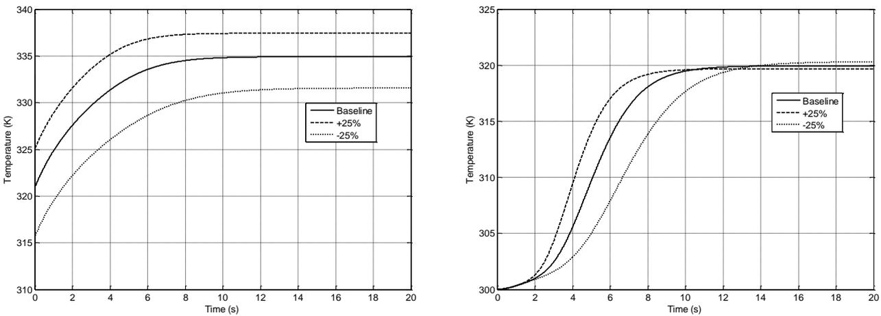
**Figure 3.37** Outlet temperature variation obtained varying the  $K_{1C_{ic}}$  and  $K_{1H_{ic}}$  variables. Air side (left). Water side (right)
