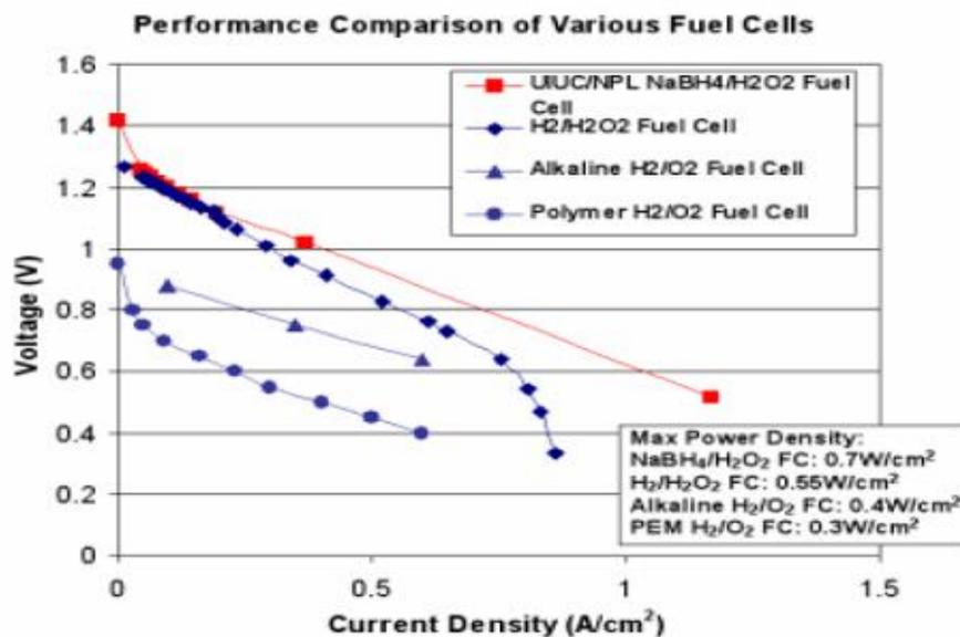
**Figure 1.4** H<sub>2</sub>O<sub>2</sub> fuel cell performance (Luo et al. 2008)
