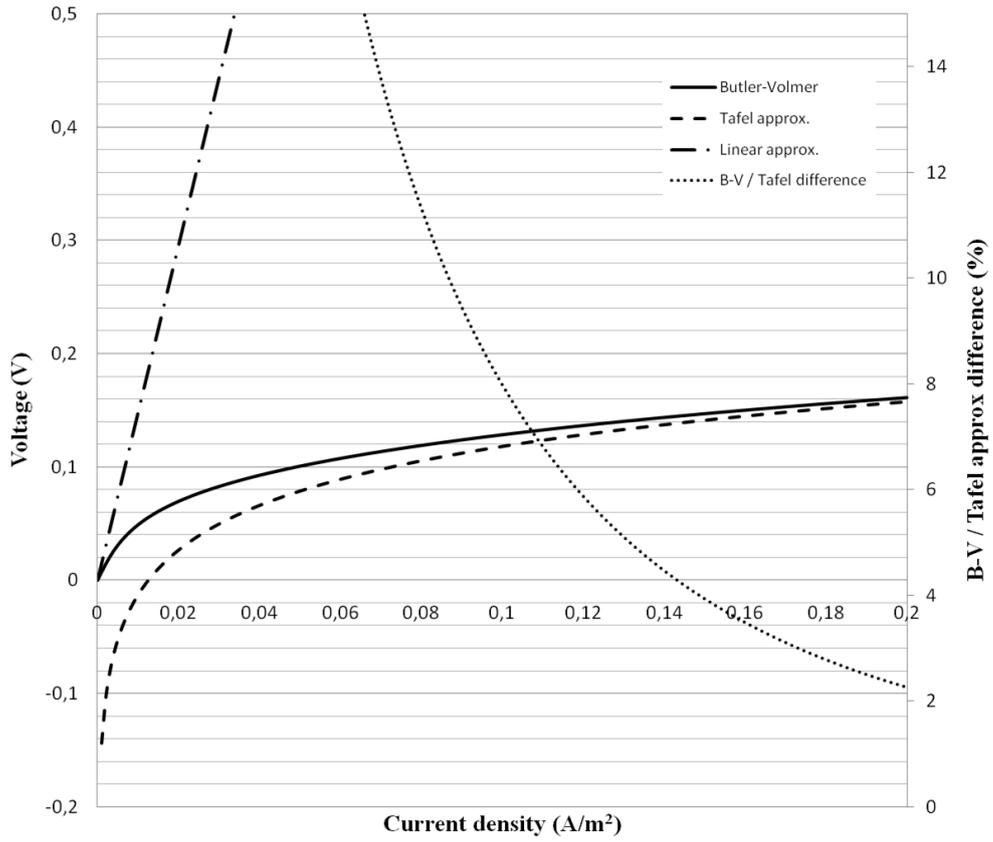
**Figure 2.8** Butler-Volmer equation and complete activation losses
