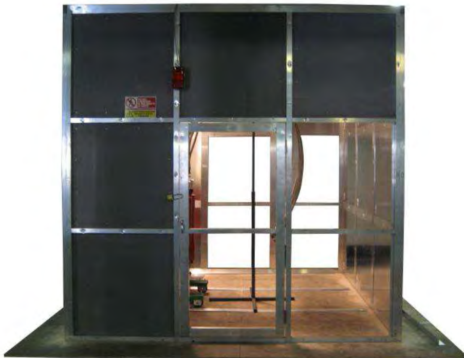
Figure 118 Shielding on the substation ceiling and on the side close to the transformer (Conf. 3)
