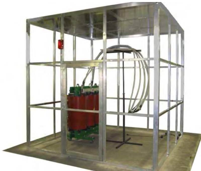
Figure 114 Shielding only on the substation ceiling (Conf. 1)
