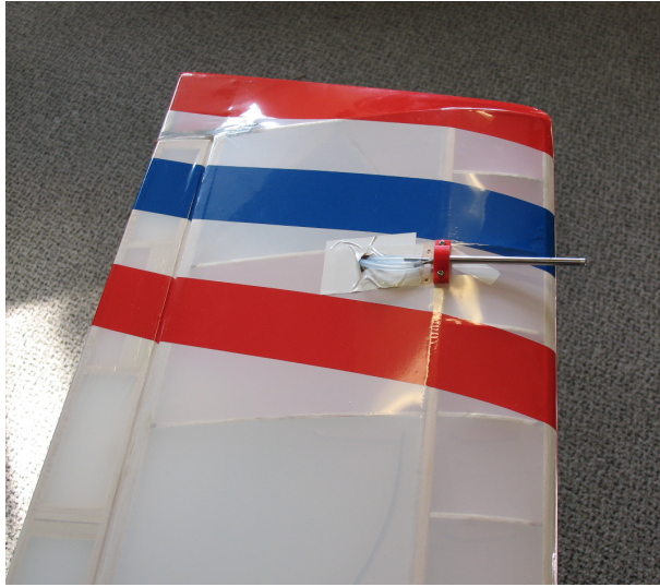
Fig. 16 Pitot installation on the Ultrastick 25e right wing
