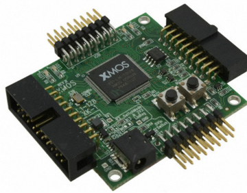
Fig. 10 XMOS XK-1A board
